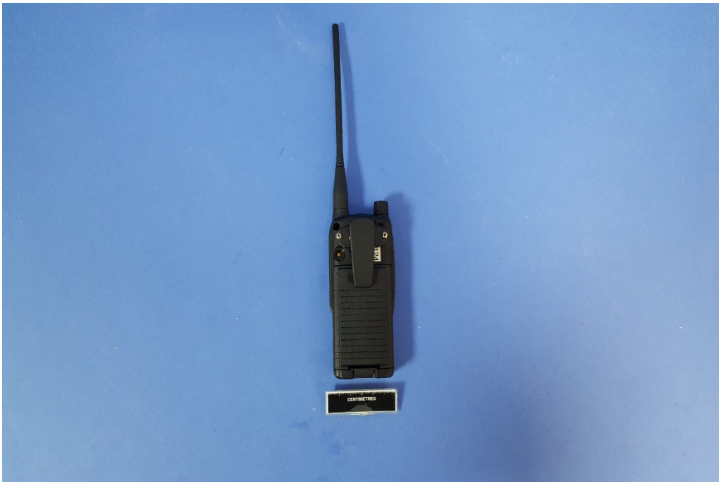
Figure 105 Rear (1/4 Wave Whip Antenna - part no: 310-00015 fitted ), 1160 mAh Battery (Part no: 300-01852)
