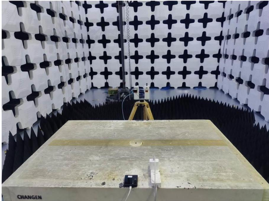
19. Radiated Emissions (Part 15B, Closed, Camera/Video Player/GSM receiver/WCDMA receiver/LTE receiver/NR receiver, 18GHz-26.5GHz)
