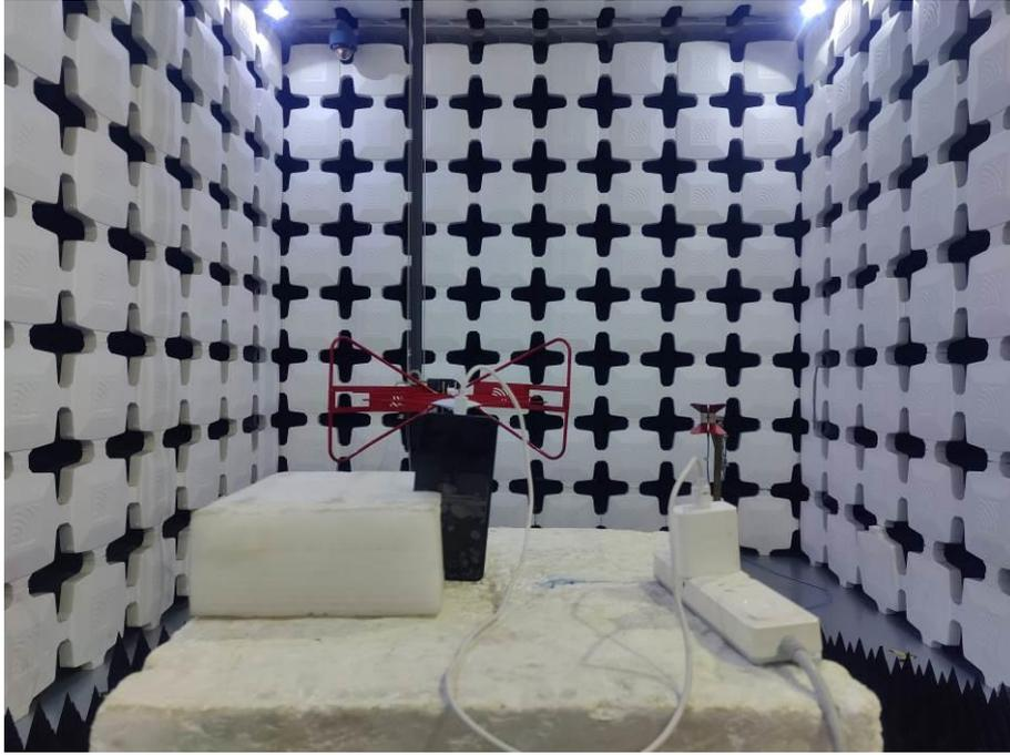
3. Radiated Emissions (Part 15C&Part 15E, Open, 1GHz -18GHz)
