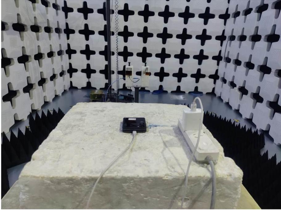
15. Radiated Emissions (Part 22/24/27/90, Closed, 18GHz-26.5GHz)
