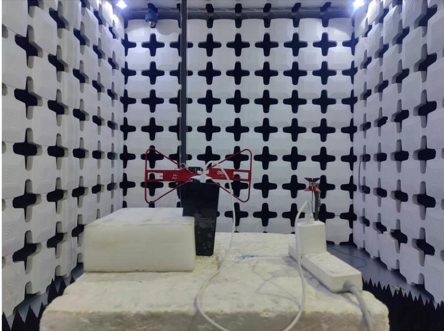
11. Radiated Emissions (Part 22/24/27/90, Open, 30MHz-18GHz)
