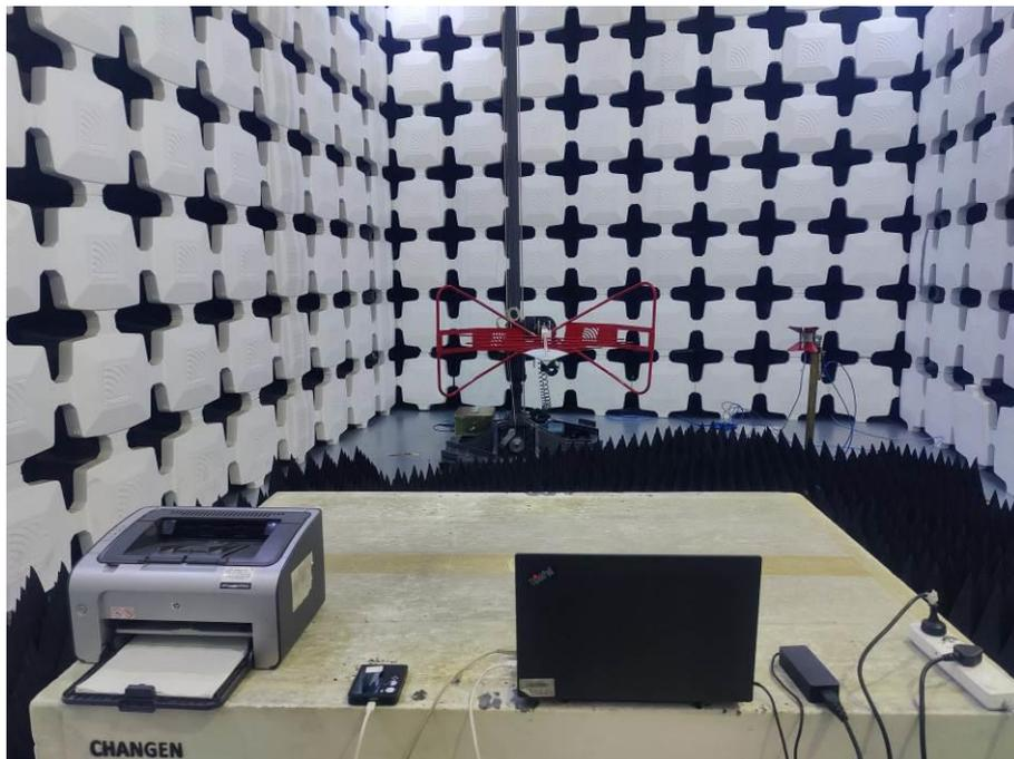
6. Radiated Emissions (Part 15B, Data Transfer, Closed, 1GHz-18GHz)
