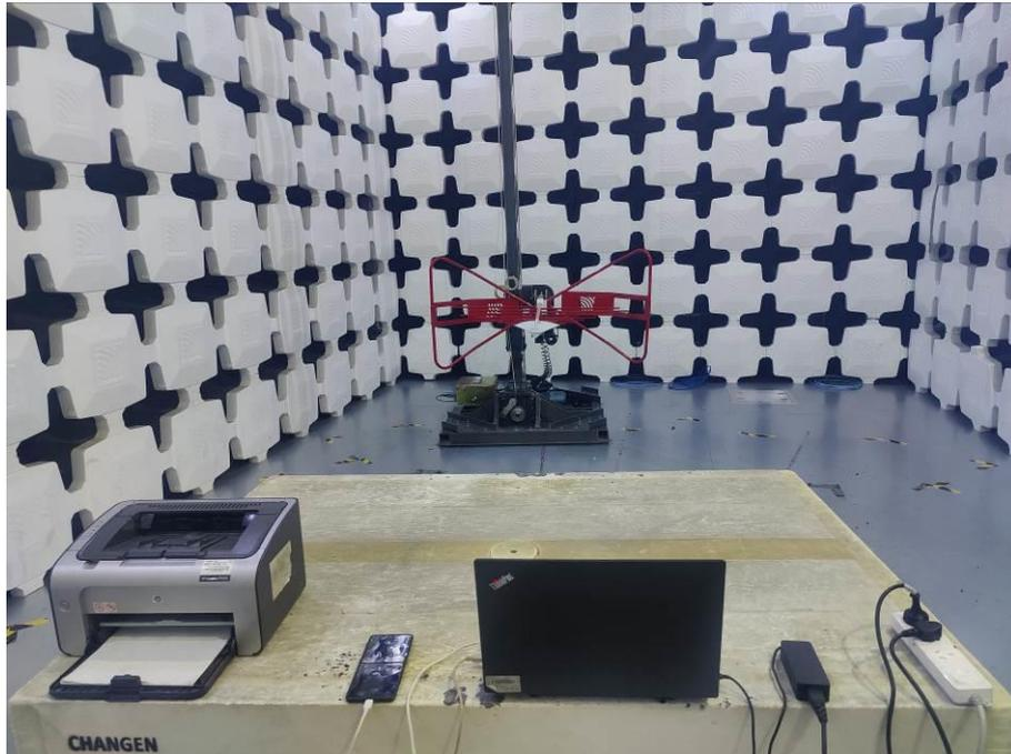
1. Radiated Emissions (Part 15B, Data Transfer, Open, 30MHz-1GHz)
