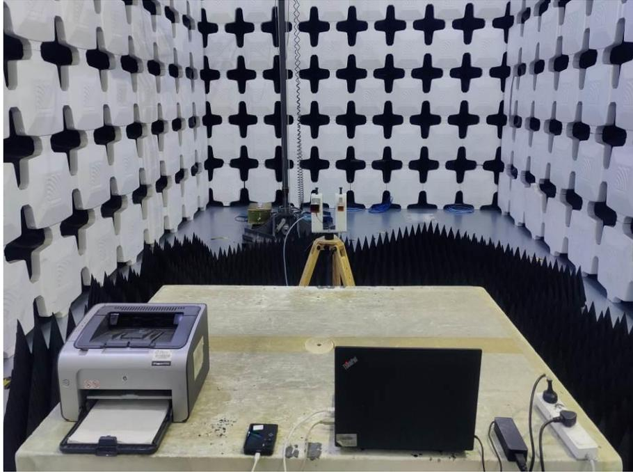
7. Radiated Emissions (Part 15B, Data Transfer, Closed, 18GHz-26.5GHz)
