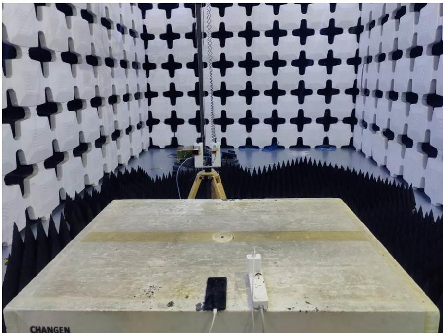
16. Radiated Emissions (Part 15B, Open, Camera/Video Player/GSM receiver/WCDMA receiver/LTE receiver/NR receiver, 26.5GHz-40GHz)
