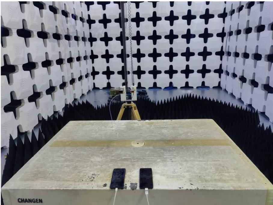
12. Radiated Emissions (Part 15B, EUT Transfer EUT, Open, 26.5GHz-40GHz)
