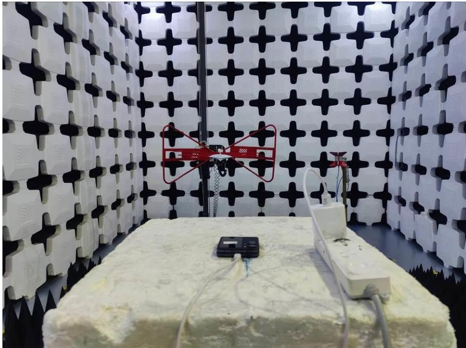
14. Radiated Emissions (Part 22/24/27/90, Closed, 30MHz-18GHz)
