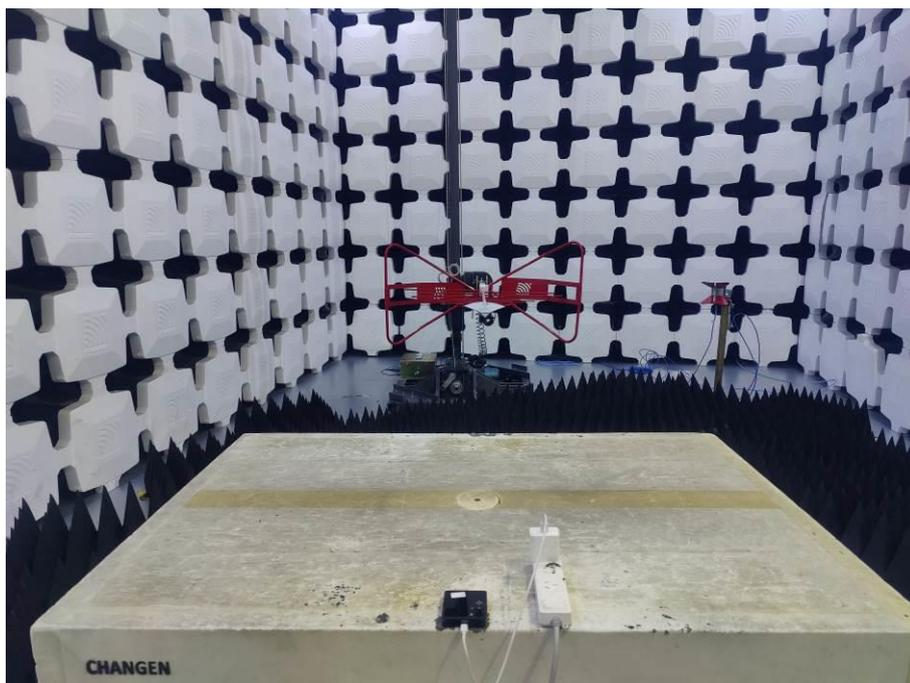
18. Radiated Emissions (Part 15B, Closed, Camera/Video Player/GSM receiver/WCDMA receiver/LTE receiver/NR receiver,1GHz-18GHz)
