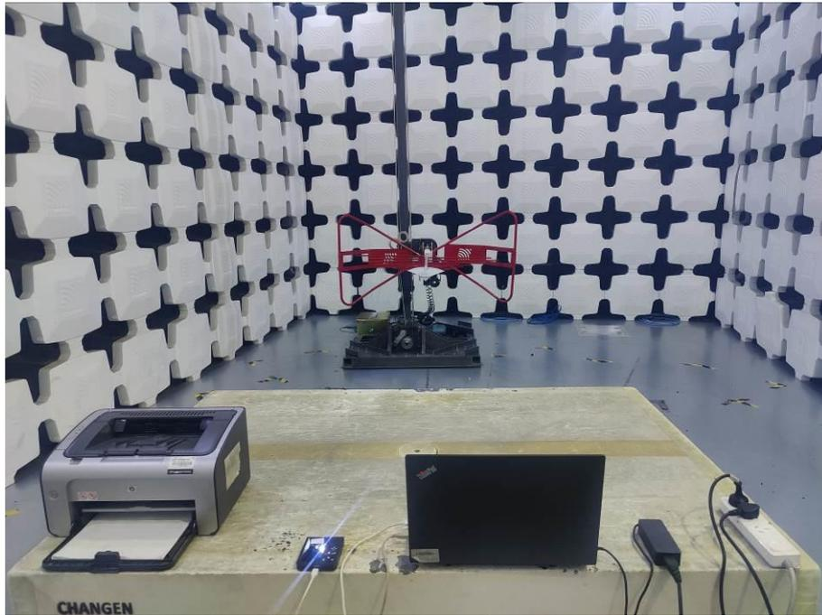
5. Radiated Emissions (Part 15B, Data Transfer, Closed, 30MHz-1GHz)
