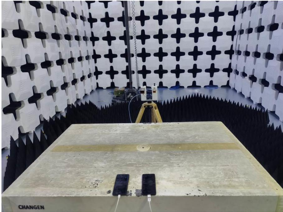
11. Radiated Emissions (Part 15B, EUT Transfer EUT, Open, 18GHz-26.5GHz)
