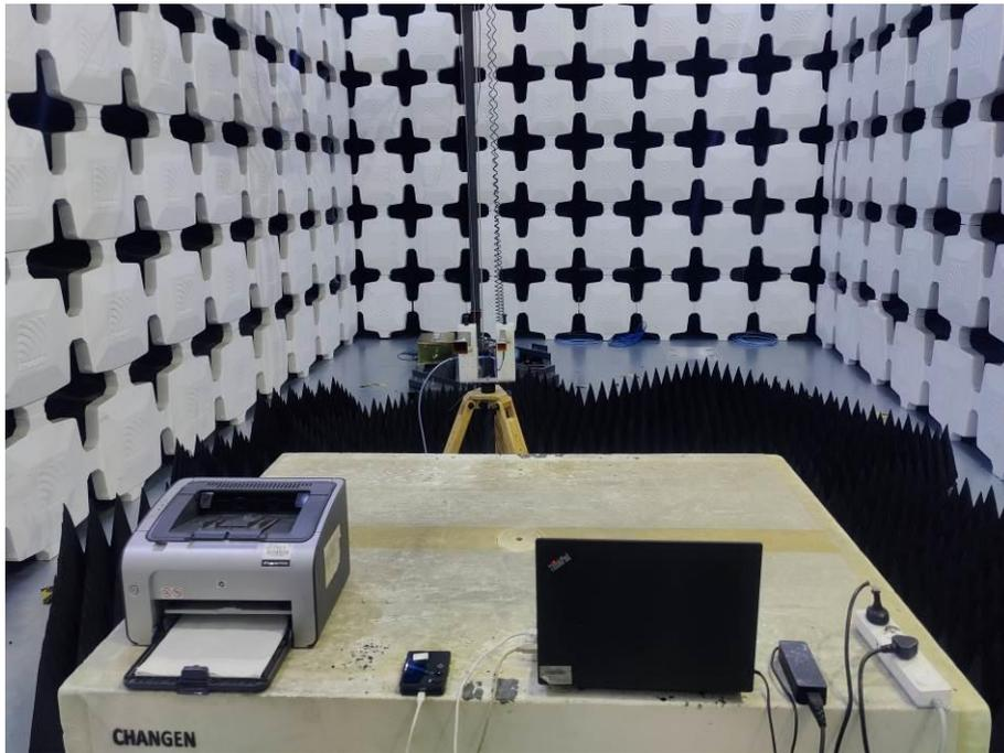
8. Radiated Emissions (Part 15B, Data Transfer, Closed, 26.5GHz-40GHz)
