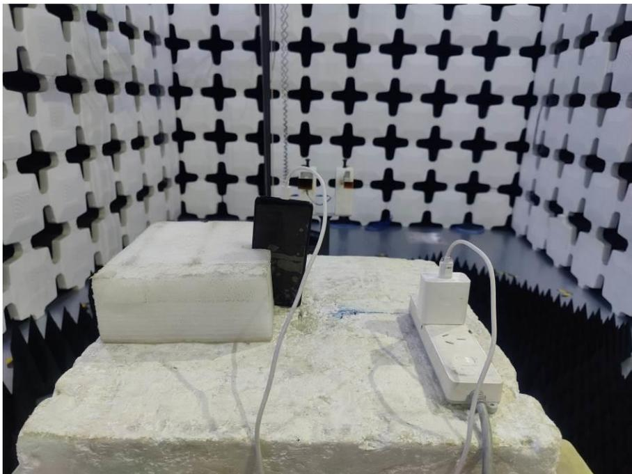
12. Radiated Emissions (Part 22/24/27/90, Open, 18GHz-26.5GHz)
