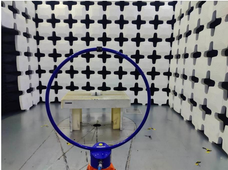
6. Radiated Emissions (Part 15C&Part 15E, Closed, 9kHz-30MHz)
