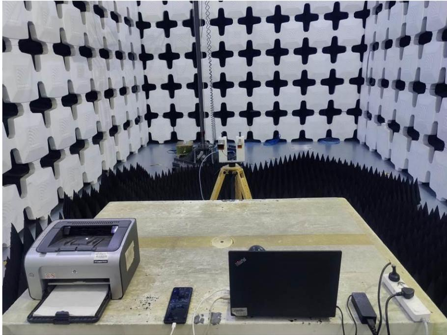
3. Radiated Emissions (Part 15B, Data Transfer, Open, 18GHz-26.5GHz)
