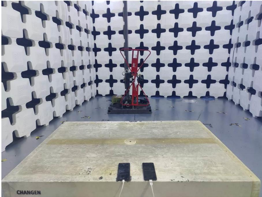
9. Radiated Emissions (Part 15B, EUT Transfer EUT, Open, 30MHz-1GHz)
