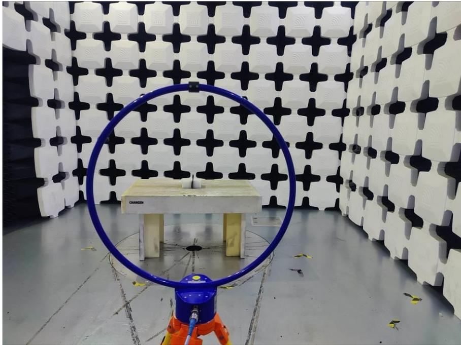
1. Radiated Emissions (Part 15C&Part 15E, Open, 9kHz-30MHz)
