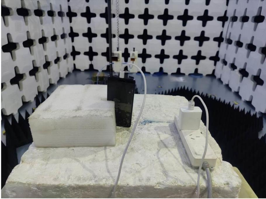
5. Radiated Emissions (Part 15C&Part 15E, Open, 26.5GHz -40GHz)
