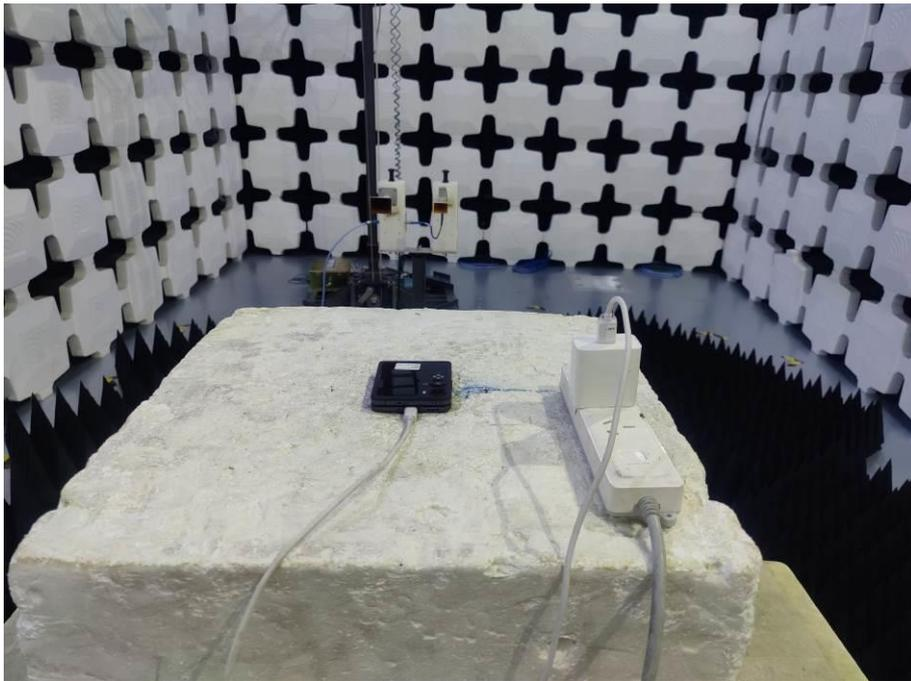
10. Radiated Emissions (Part 15C&Part 15E, Closed, 26.5GHz -40GHz)
