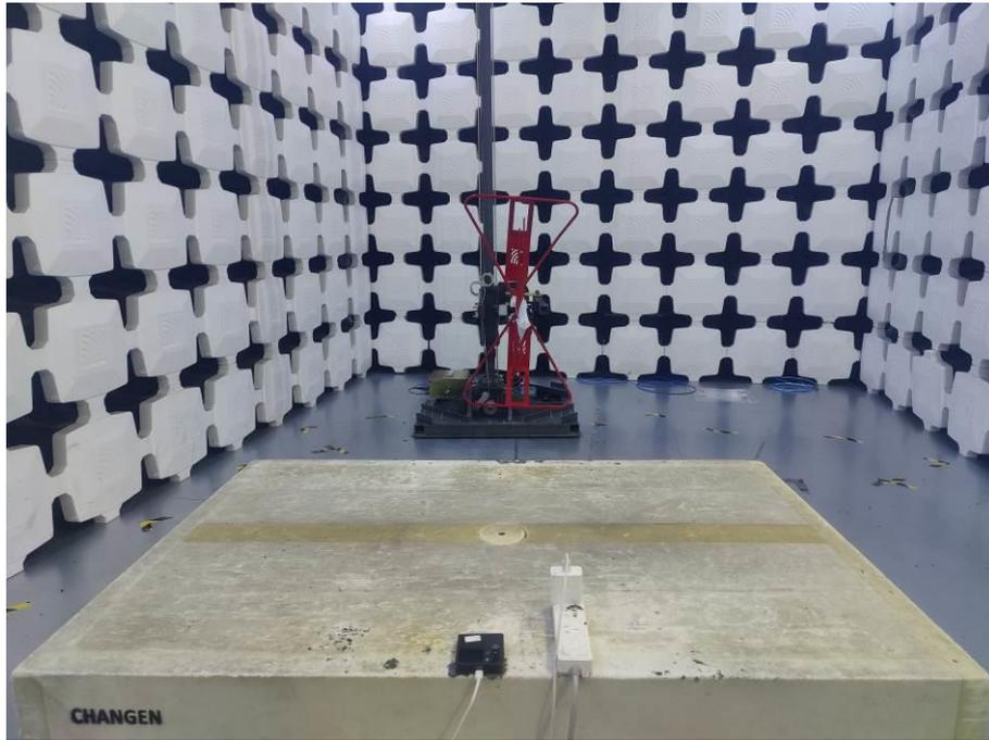
7. Radiated Emissions (Part 15C&Part 15E, Closed, 30MHz-1GHz)
