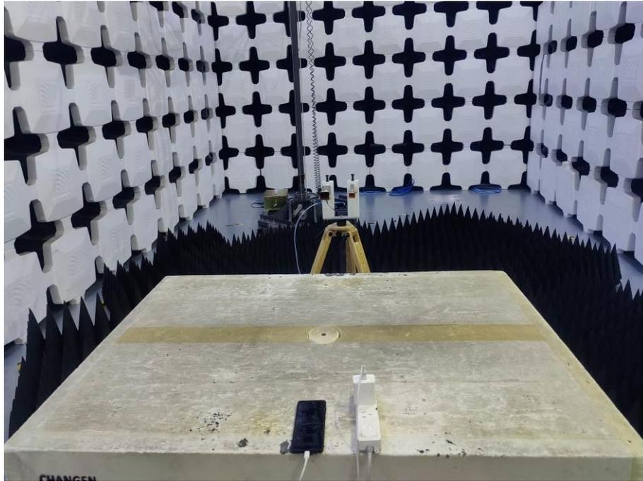
15. Radiated Emissions (Part 15B, Open, Camera/Video Player/GSM receiver/WCDMA receiver/LTE receiver/NR receiver, 18GHz-26.5GHz)
