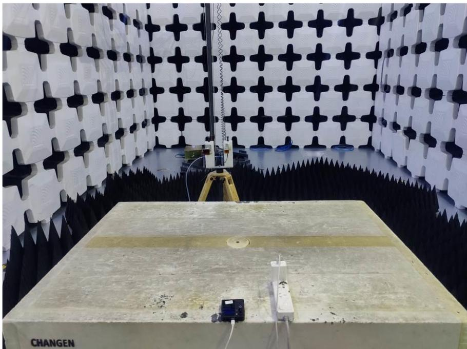
20. Radiated Emissions (Part 15B, Closed, Camera/Video Player/GSM receiver/WCDMA receiver/LTE receiver/NR receiver, 26.5GHz-40GHz)
