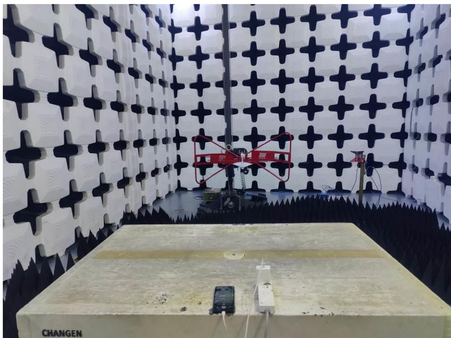
14. Radiated Emissions (Part 15B, Open, Camera/Video Player/GSM receiver/WCDMA receiver/LTE receiver/NR receiver,1GHz-18GHz)
