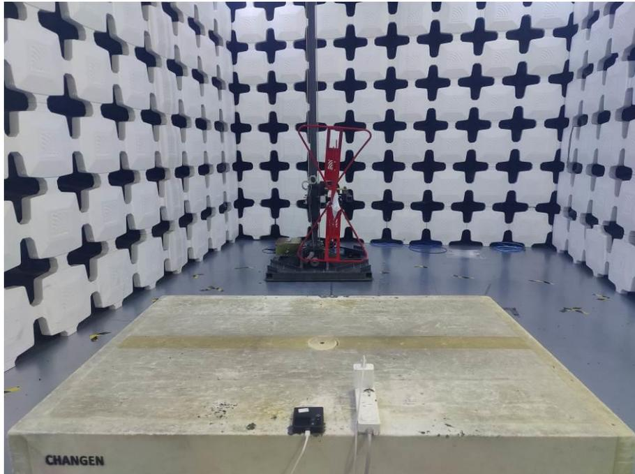
17. Radiated Emissions (Part 15B, Closed, Camera/Video Player/GSM receiver/WCDMA receiver/LTE receiver/NR receiver,30MHz-1GHz)
