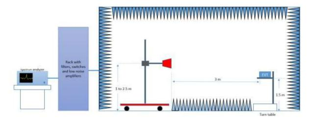
Radiated Setup 18 GHz - 26.5 GHz
