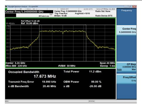
The test was performed on the worst case data rate for 802.11(n) - 20 MHz BW modulation. The worst case was deemed as the data rate which produced the highest level of conducted average power. This data rate was MCS7.
