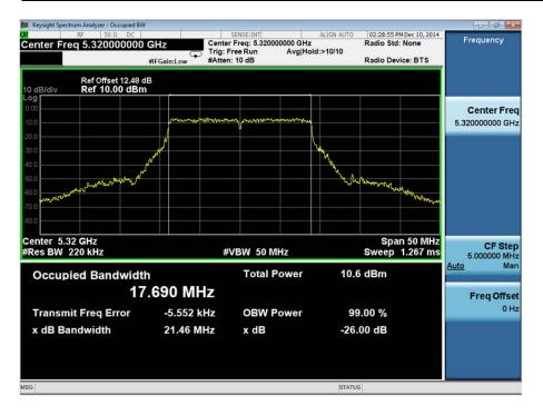
The test was performed on the worst case data rate for 802.11(ac) - 20 MHz BW modulation. The worst case was deemed as the data rate which produced the highest level of conducted average power. This data rate was MCS0.
