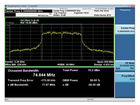
The test was performed on the worst case data rate for 802.11(ac) - 80 MHz BW modulation. The worst case was deemed as the data rate which produced the highest level of conducted average power. This data rate was MCS5.
