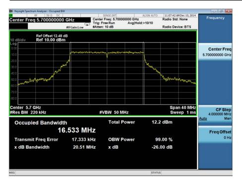
The test was performed on the worst case data rate for 802.11(a) modulation. The worst case was deemed as the data rate which produced the highest level of conducted average power. This data rate was 6 Mbps.
