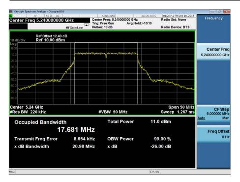
The test was performed on the worst case data rate for 802.11(ac) - 20 MHz BW modulation. The worst case was deemed as the data rate which produced the highest level of conducted average power. This data rate was MCS0.
