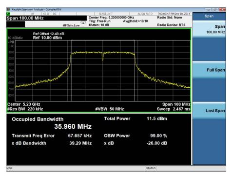
The test was performed on the worst case data rate for 802.11(ac) - 40 MHz BW modulation. The worst case was deemed as the data rate which produced the highest level of conducted average power. This data rate was MCS0.
