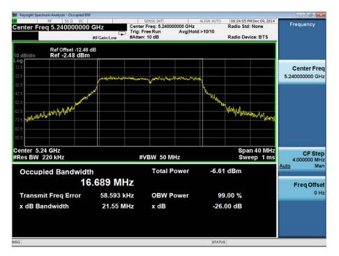
The test was performed on the worst case data rate for 802.11(a) modulation. The worst case was deemed as the data rate which produced the highest level of conducted average power. This data rate was 6 Mbps.
