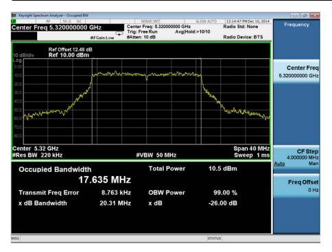
The test was performed on the worst case data rate for 802.11(n) - 20 MHz BW modulation. The worst case was deemed as the data rate which produced the highest level of conducted average power. This data rate was MCS7.
