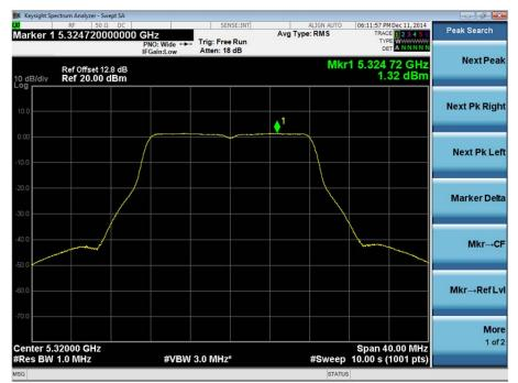
The test was performed on the worst case data rate for 802.11(a) modulation. The worst case was deemed as the data rate which produced the highest level of conducted average power. This data rate was 9 Mbps.
