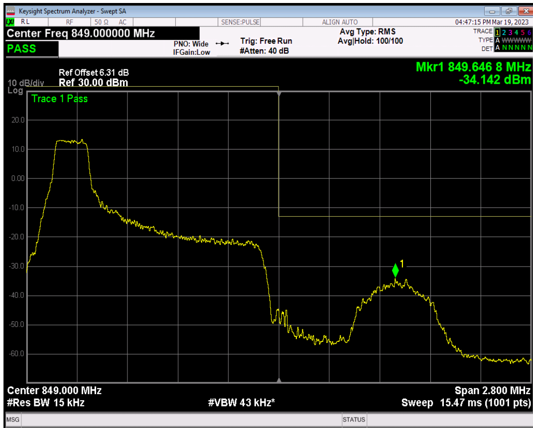
Band26(824-849) QAM16 BW=1.4MHz Channel=27033 RB Size=1 Position=#Max
