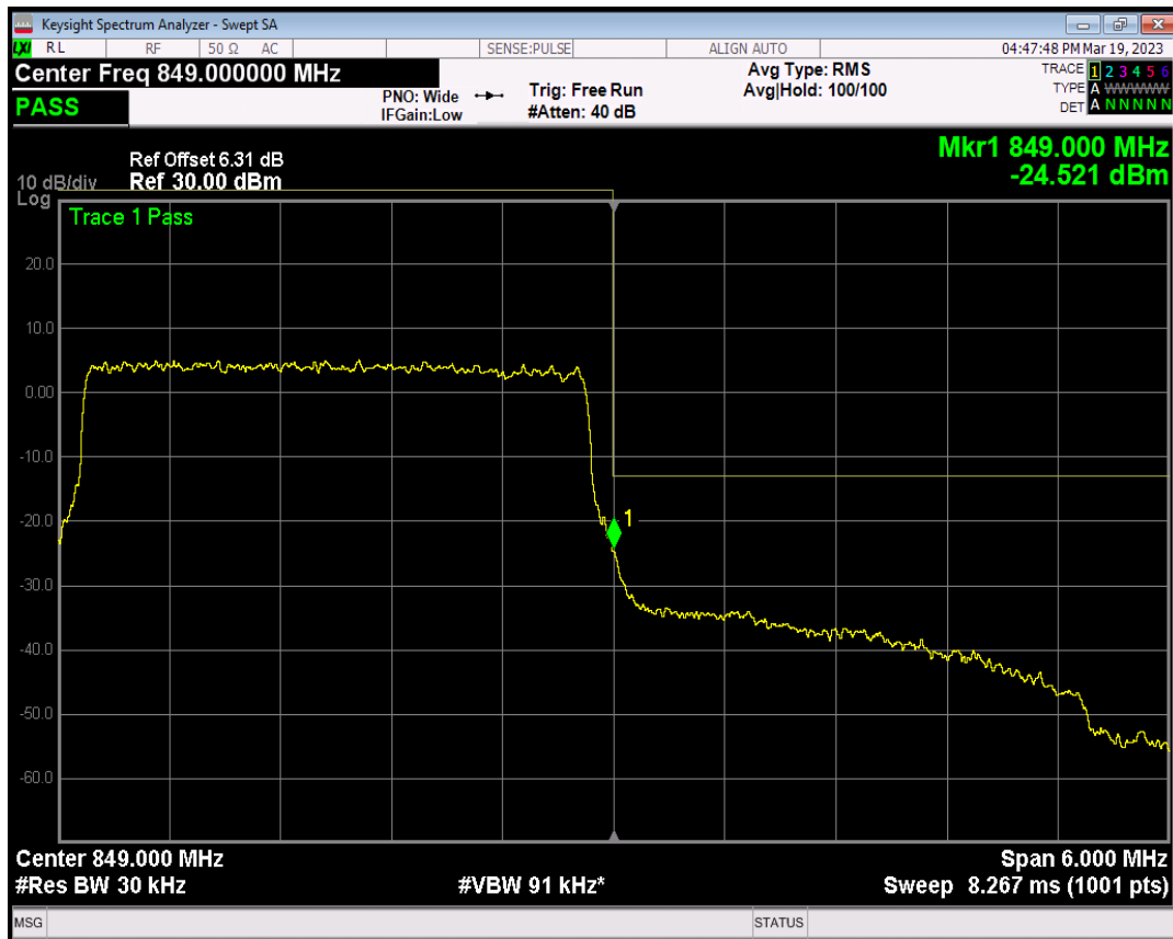
Band26(824-849) QAM16 BW=3MHz Channel=27025 RB Size=1 Position=#0
