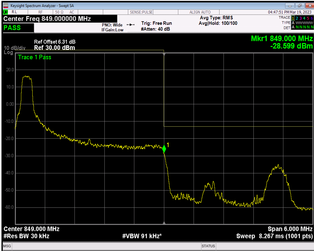
Band26(824-849) QAM16 BW=3MHz Channel=27025 RB Size=1 Position=#Max
