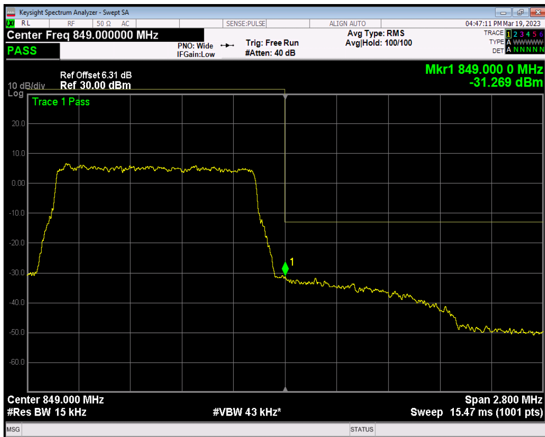
Band26(824-849) QAM16 BW=1.4MHz Channel=27033 RB Size=1 Position=#0
