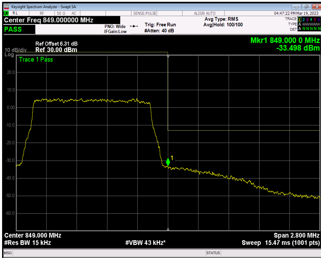
Band26(824-849) QPSK BW=3MHz Channel=26805 RB Size=1 Position=#0
