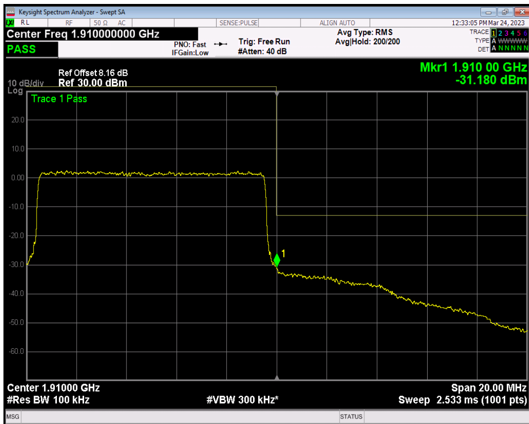
Band2 QAM16 BW=10MHz Channel=19150 RB Size=1 Position=#0
