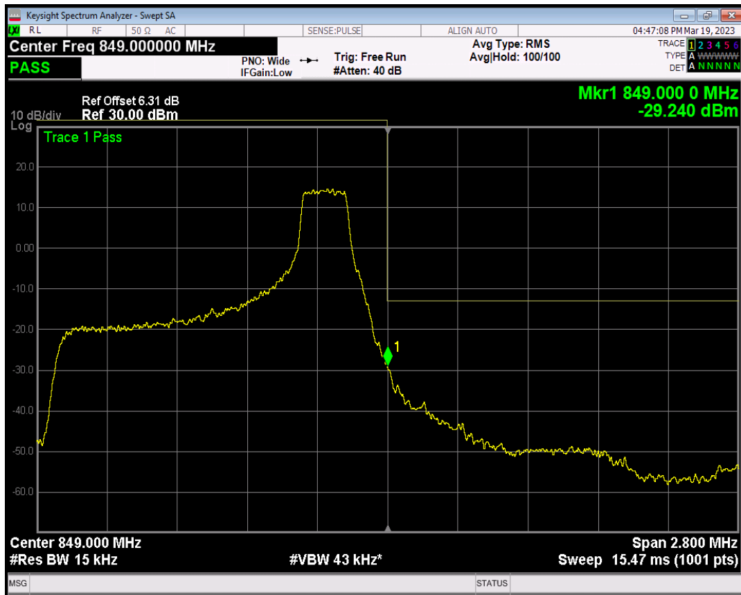
Band26(824-849) QPSK BW=1.4MHz Channel=27033 RB Size=6 Position=#0
