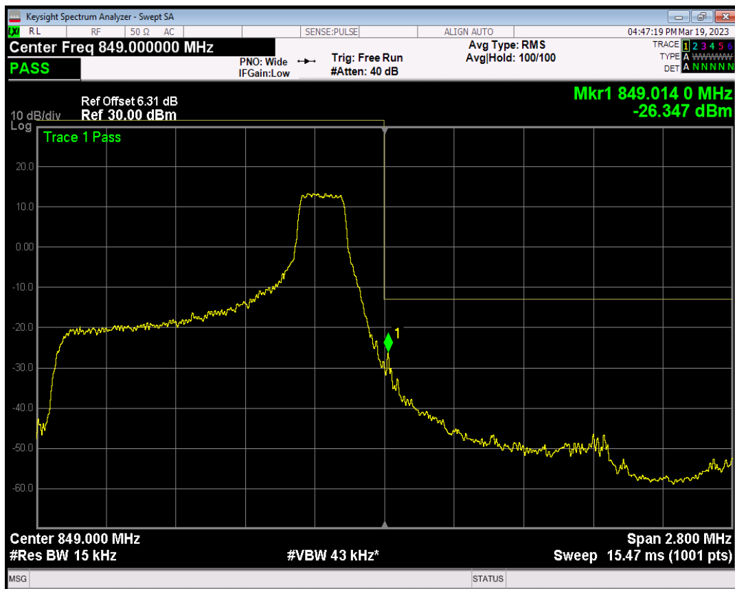
Band26(824-849) QAM16 BW=1.4MHz Channel=27033 RB Size=6 Position=#0
