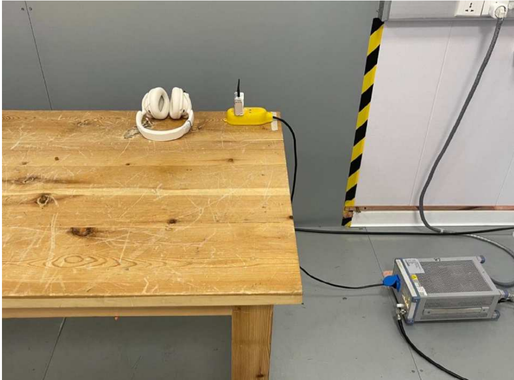
Photograph 1: Set-up for Conducted Emission on AC Mains
