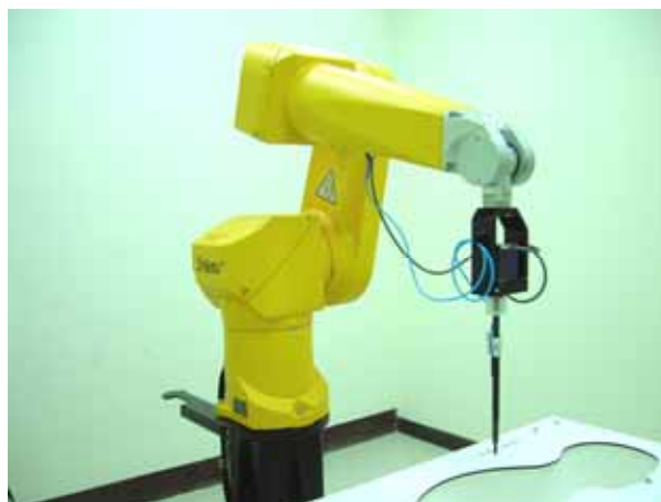
Fig. 5.2 Probe setup on robot
