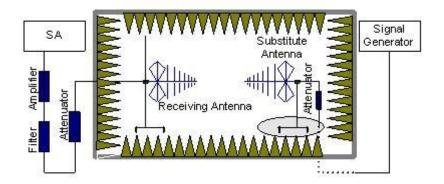
In the chamber, an substitution antenna for the frequency band of interest is placed at the reference point of the chamber. An RF Signal source for the frequency band of interest is connected to the substitution antenna with a cable that has been constructed to not interfere with the radiation pattern of the antenna. A power  $(P_{Mea})$  is applied to the input of the substitution antenna, and adjusts the level of the signal generator output until the value of the
