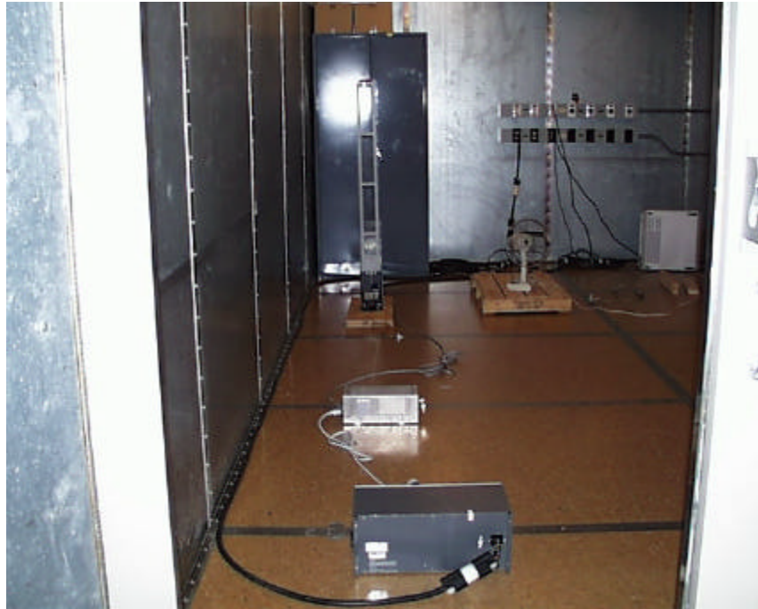
Photo 6 – Strata SX Conducted Emissions Test Setup
