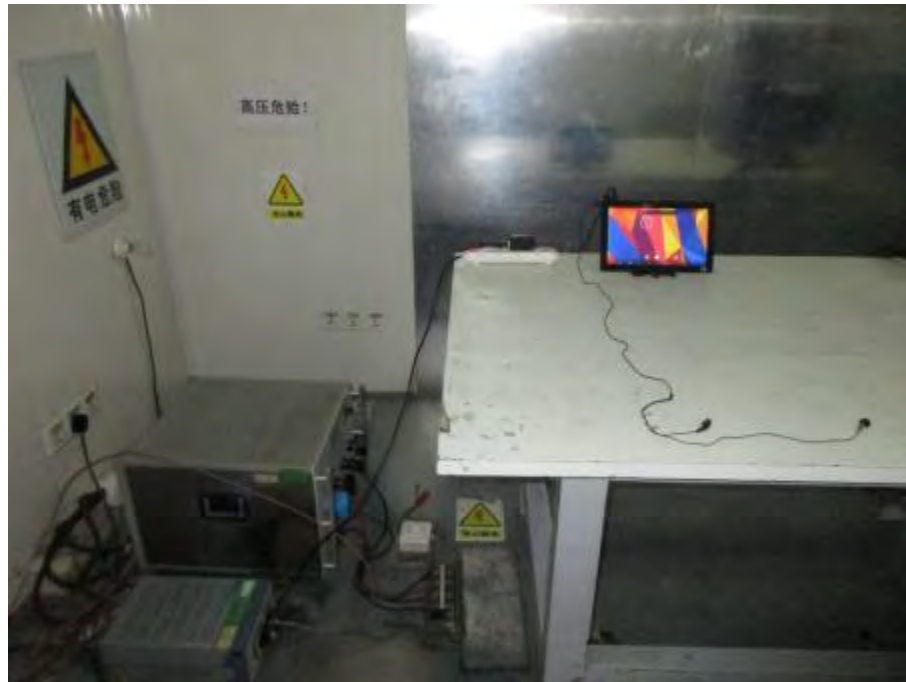
Photograph 5: Set-up for Conducted Emission
