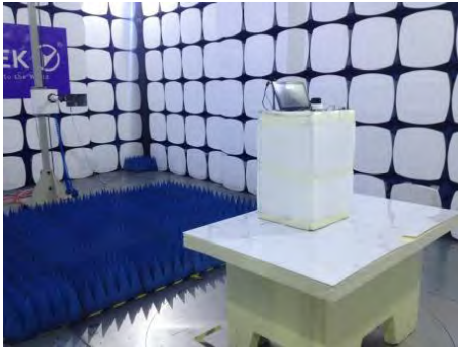
Photograph 4: Set-up for Radiated Spurious Emission (18GHz ~ 26GHz)
