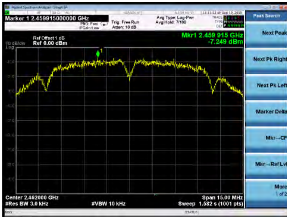
Test Plot of Power Spectral Density, 802.11g
