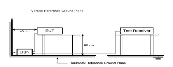
The LISN edge is arranged parallel to the edge of the test table
