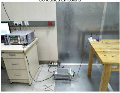
Radiated Spurious Emissions Test Frequency From 30MHz-1000MHz
