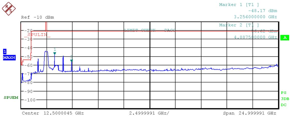
Figure 59: Chart of emissions test from 9 kHz to 25 GHz on middle channel, PK-detector, IEEE 802.11 g
