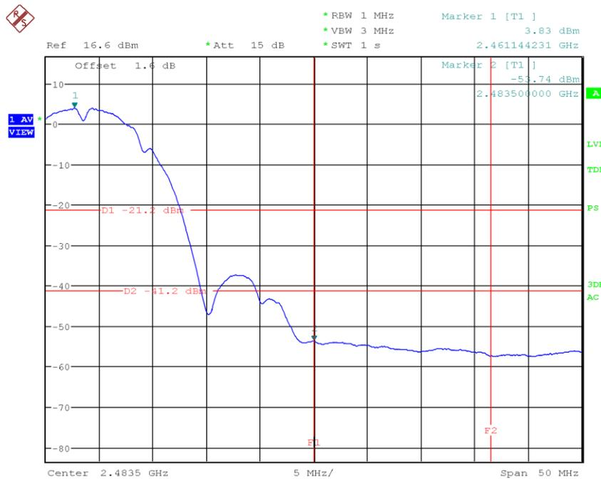
Figure 44: Chart of band-edge measurement on highest channel (AV), IEEE 802.11 b
