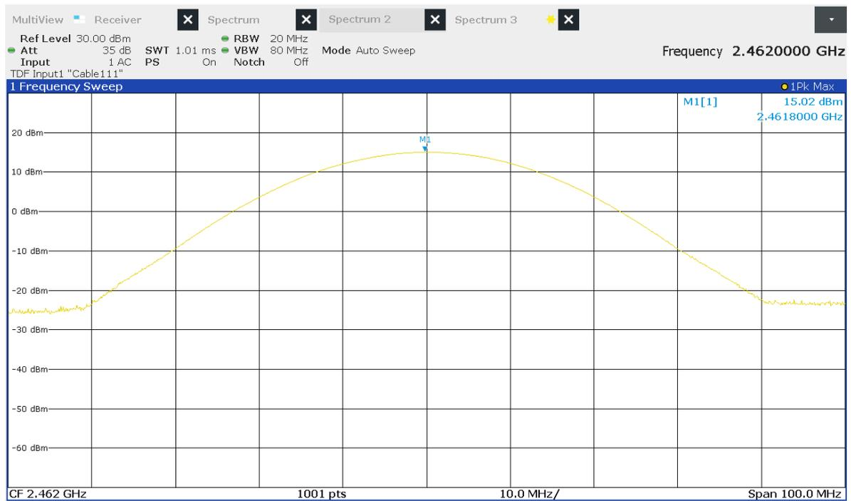
Figure 26: Chart of conducted output power on highest channel, IEEE 802.11 b
