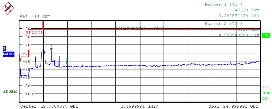
Figure 61: Chart of emissions test from 9 kHz to 25 GHz on highest channel, PK-detector, IEEE 802.11 g
