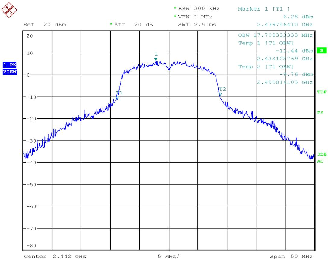
Figure 19: Chart of occupied bandwidth test on middle channel, IEEE 802.11 g
