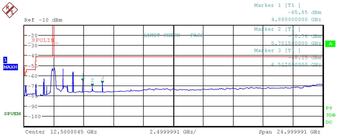
Figure 60: Chart of emissions test from 9 kHz to 25 GHz on middle channel, RMS-detector, IEEE 802.11 g
