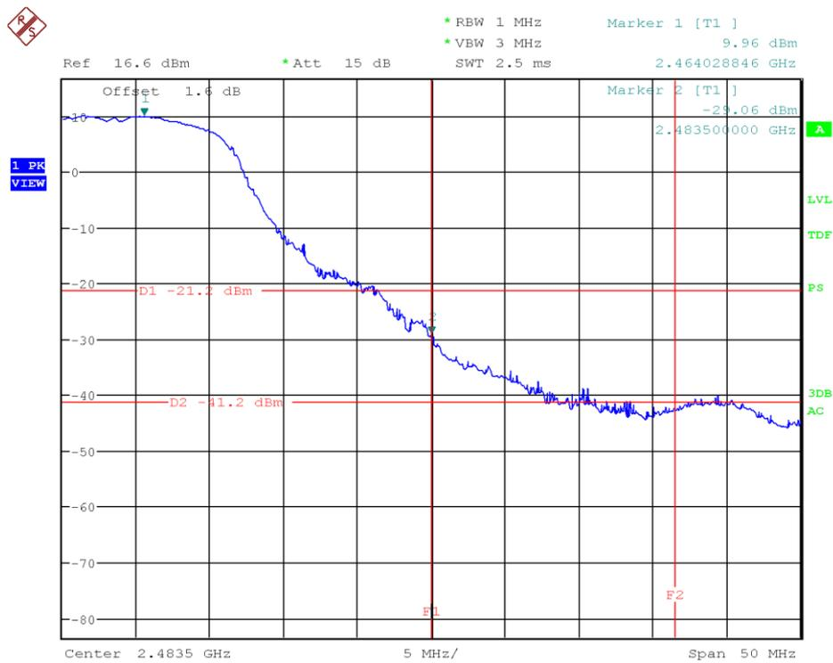
Figure 46: Chart of band-edge measurement on highest channel (PK), IEEE 802.11 g
