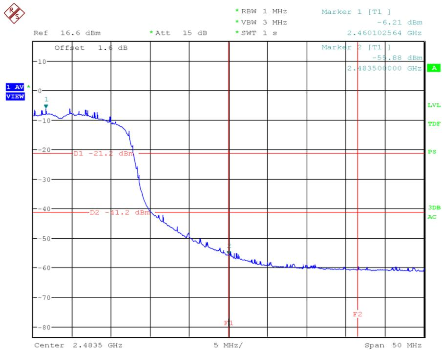
Figure 50: Chart of band-edge measurement on highest channel (AV), IEEE 802.11 n (HT20)
