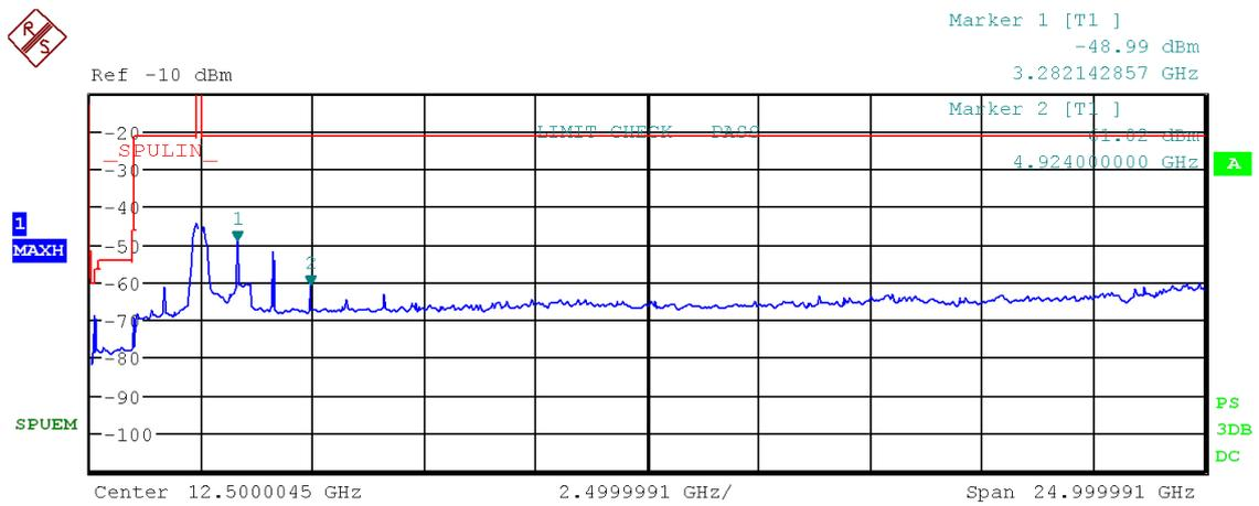
Figure 55: Chart of emissions test from 9 kHz to 25 GHz on highest channel, PK-detector, IEEE 802.11 b
