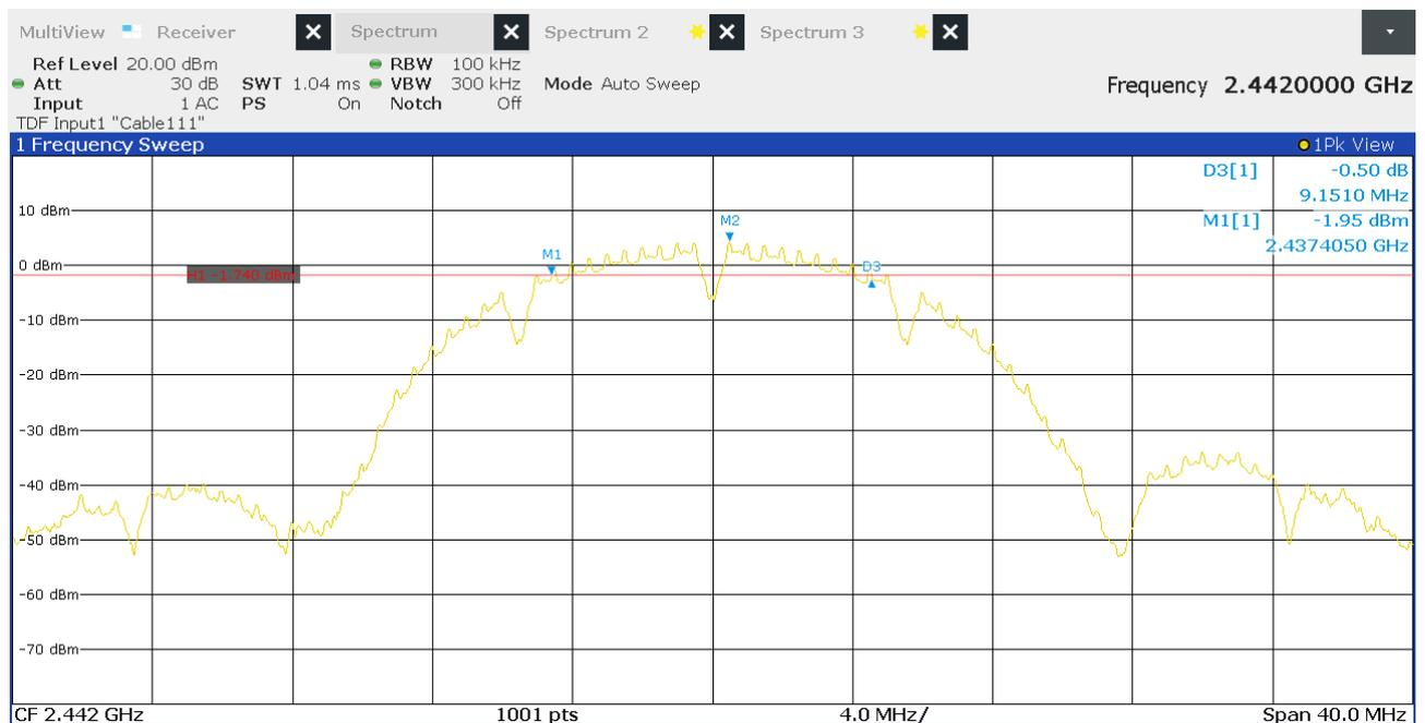
Figure 7: Chart of 6 dB bandwidth test on middle channel, IEEE 802.11 b
