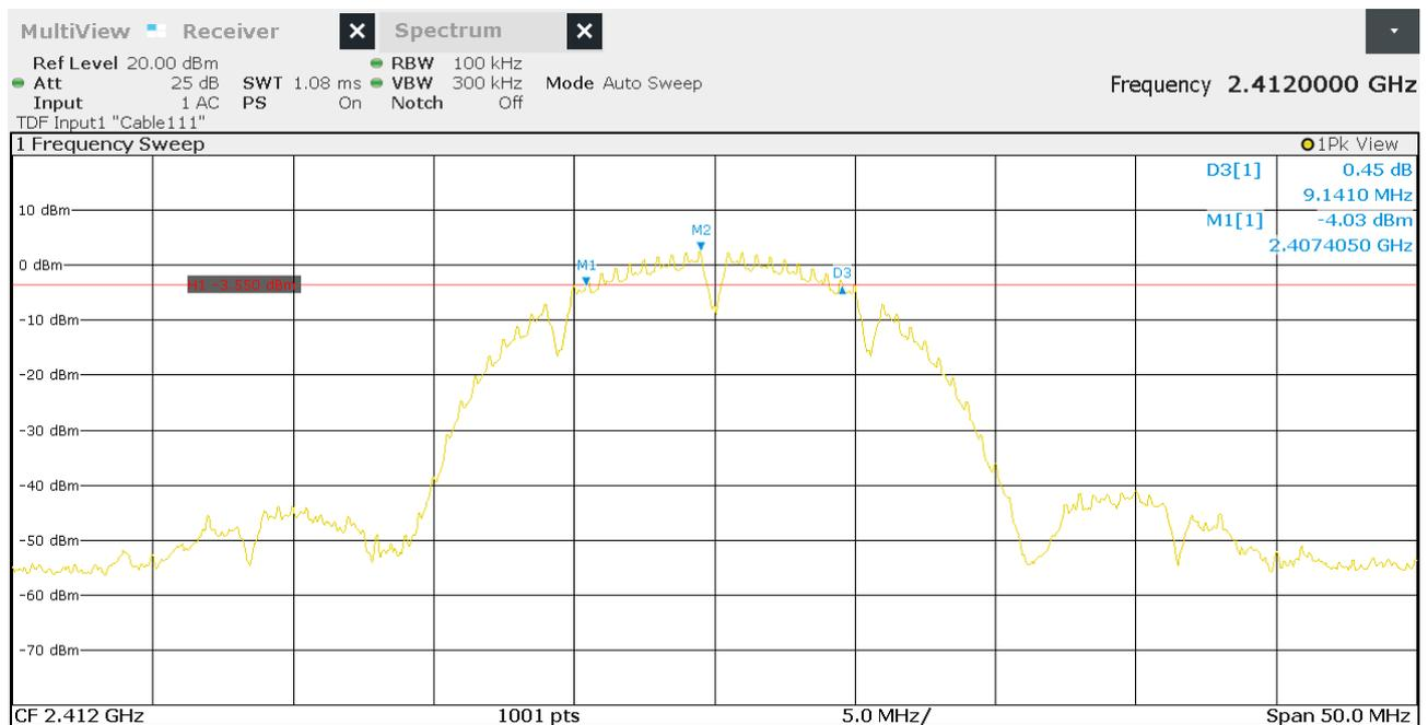
Figure 6: Chart of 6 dB bandwidth test on lowest channel, IEEE 802.11 b
