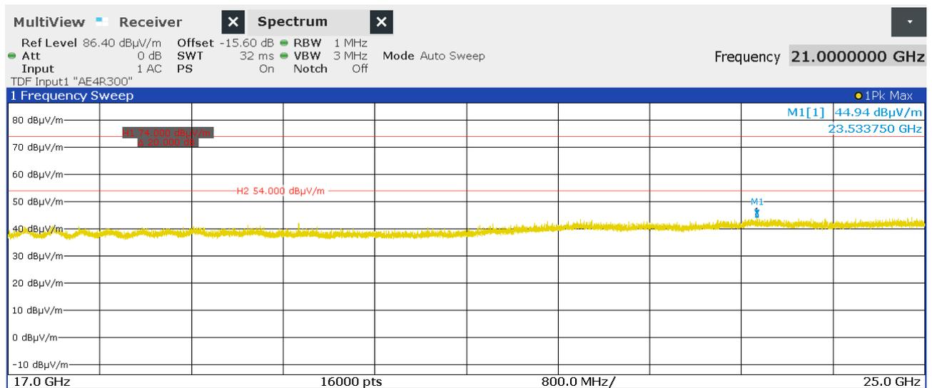
Figure 74: Chart of exploratory emission test from 17 GHz to 25 GHz on middle channel at 0.5 m
