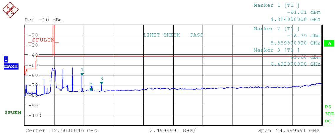
Figure 52: Chart of emissions test from 9 kHz to 25 GHz on lowest channel, RMS-detector, IEEE 802.11 b
