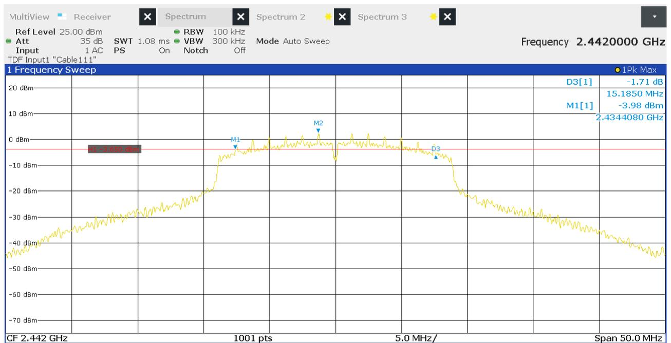
Figure 13: Chart of 6 dB bandwidth test on middle channel, IEEE 802.11 n (HT20)
