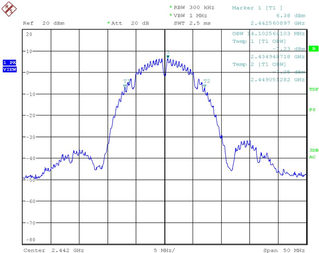
Figure 16: Chart of occupied bandwidth test on middle channel, IEEE 802.11 b
