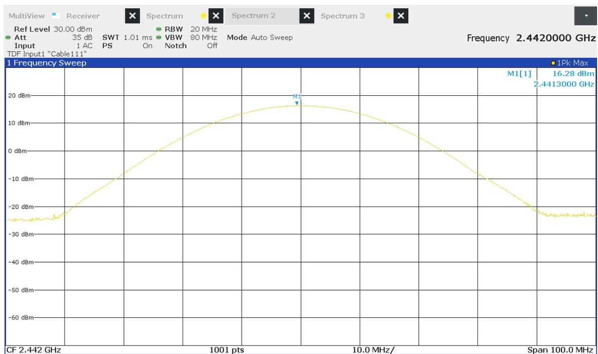
Figure 25: Chart of conducted output power on middle channel, IEEE 802.11 b
