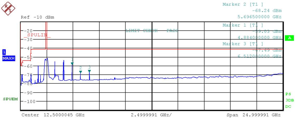
Figure 54: Chart of emissions test from 9 kHz to 25 GHz on middle channel, RMS-detector, IEEE 802.11 b
