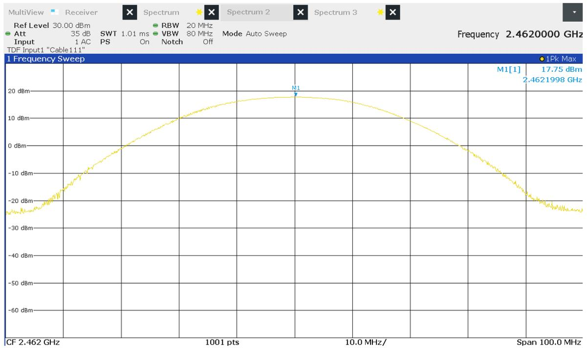
Figure 29: Chart of conducted output power on highest channel, IEEE 802.11 g
