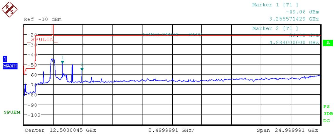
Figure 53: Chart of emissions test from 9 kHz to 25 GHz on middle channel, PK-detector, IEEE 802.11 b
