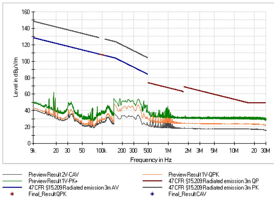
Figure 69: Chart of emissions test below 30 MHz on highest channel, EUT position X, antenna parallel to the EUT
