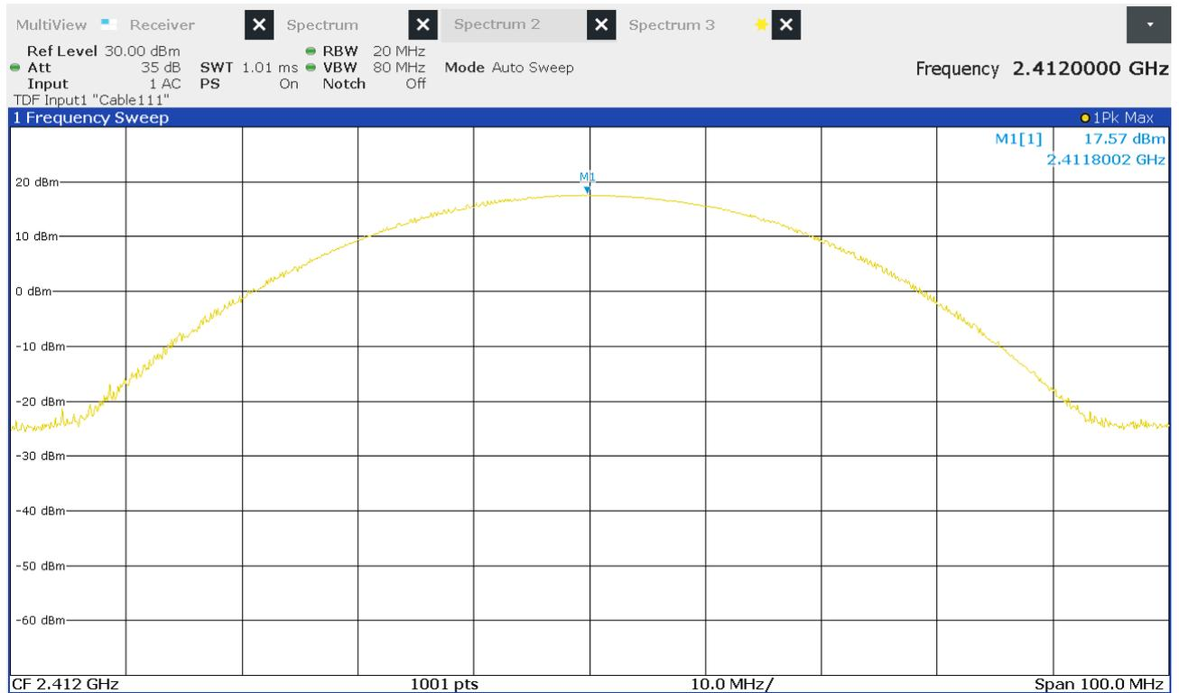
Figure 30: Chart of conducted output power on lowest channel, IEEE 802.11 n (HT20)
