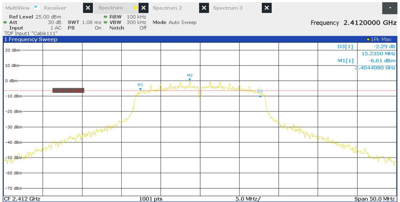
Figure 9: Chart of 6 dB bandwidth test on lowest channel, IEEE 802.11 g
