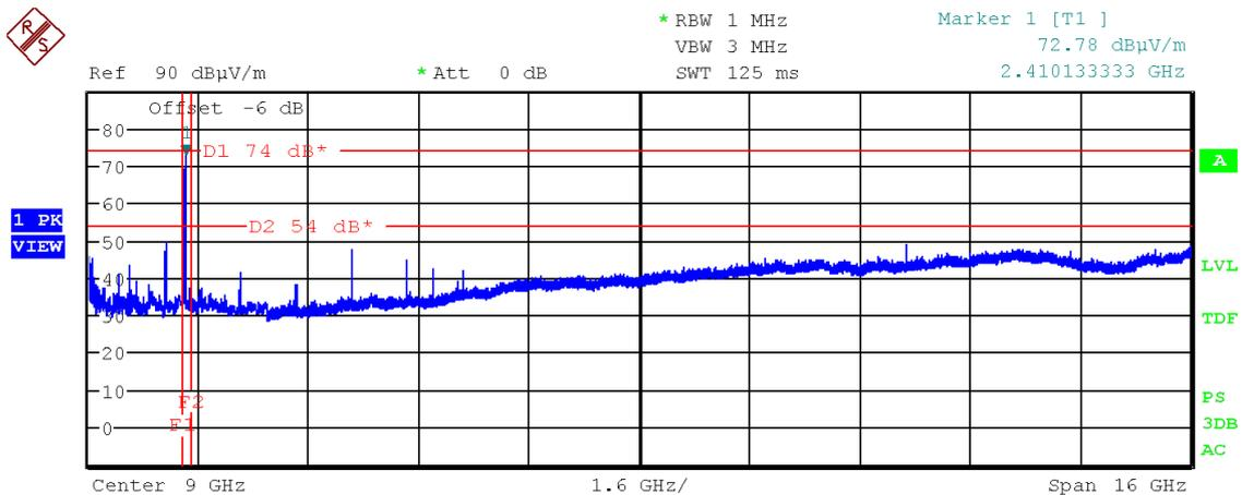
Figure 71: Chart of emissions test from 1 GHz to 17 GHz on lowest channel, EUT position Z, antenna polarization horizontal
