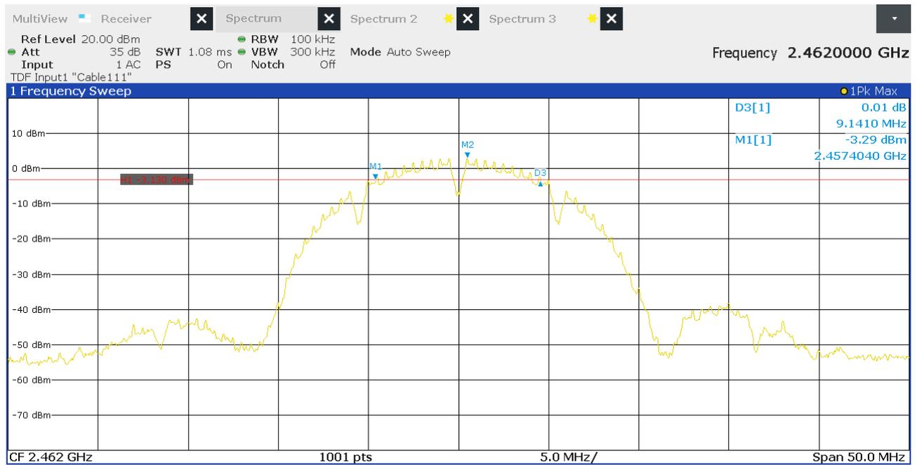
Figure 8: Chart of 6 dB bandwidth test on highest channel, IEEE 802.11 b
