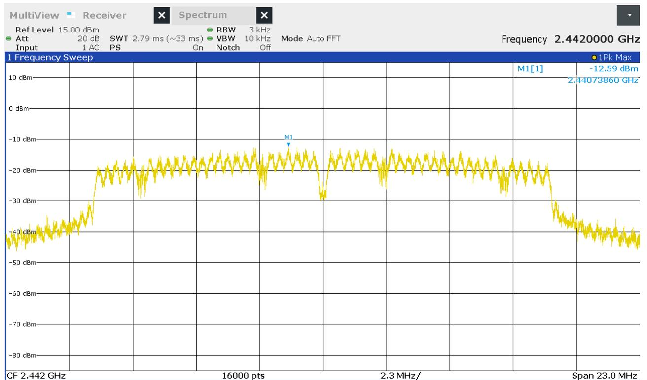
Figure 37: Chart of power spectral density on middle channel, IEEE 802.11 g
