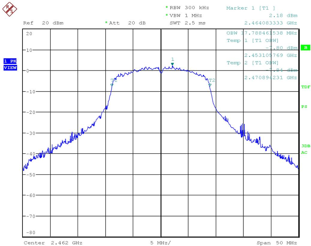
Figure 23: Chart of occupied bandwidth test on highest channel, IEEE 802.11 n (HT20)
