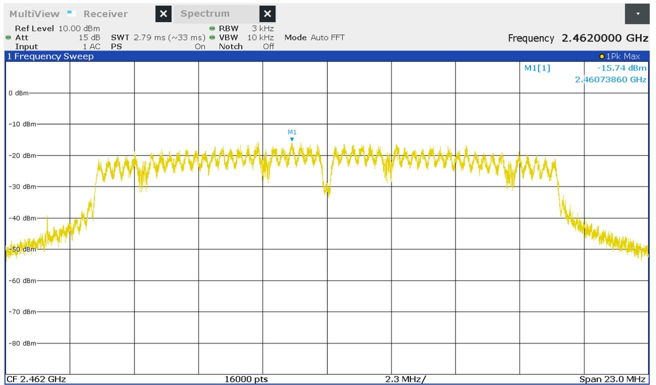
Figure 38: Chart of power spectral density on highest channel, IEEE 802.11 g
