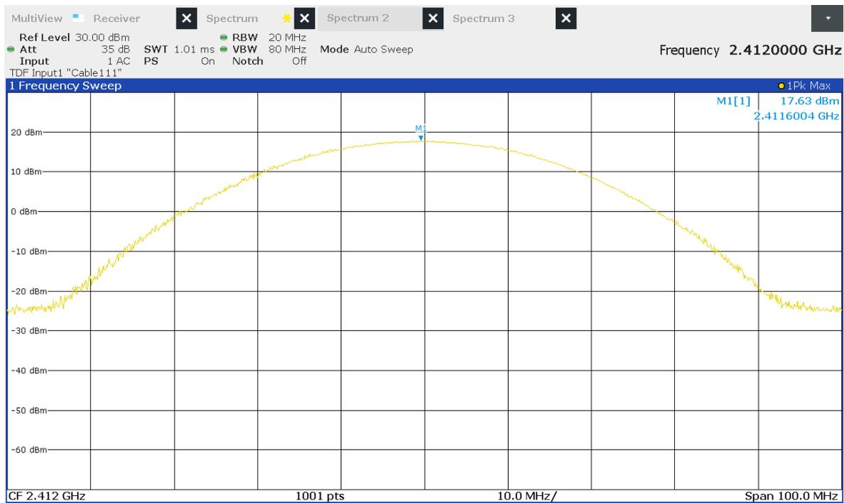
Figure 27: Chart of conducted output power on lowest channel, IEEE 802.11 g
