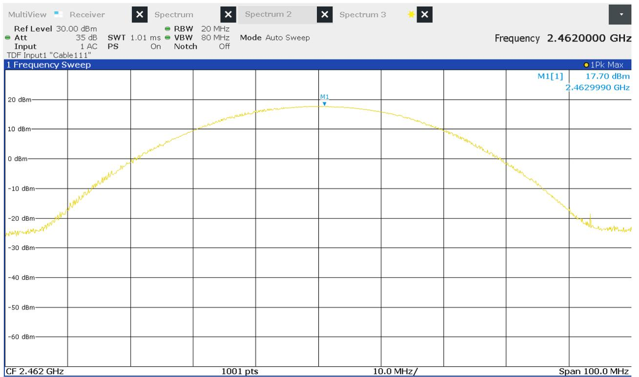
Figure 32: Chart of conducted output power on highest channel, IEEE 802.11 n (HT20)
