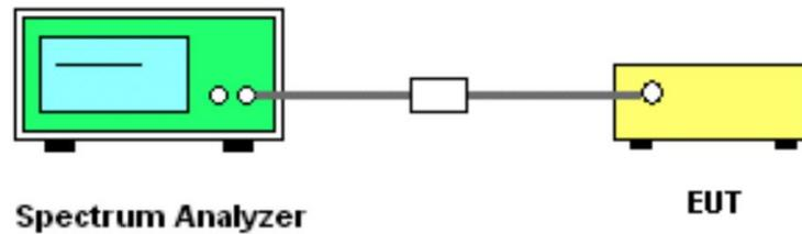
Figure 1: Setup for antenna-port conducted measurements
