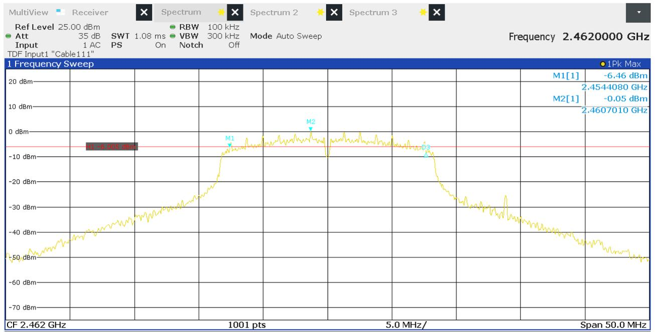
Figure 11: Chart of 6 dB bandwidth test on highest channel, IEEE 802.11 g
