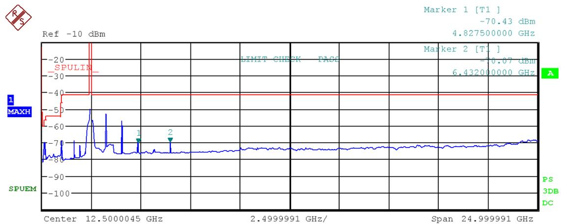
Figure 64: Chart of emissions test from 9 kHz to 25 GHz on lowest channel, RMS-detector, IEEE 802.11 n (HT20)
