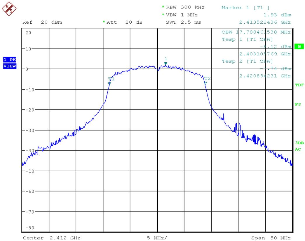
Figure 21: Chart of occupied bandwidth test on lowest channel, IEEE 802.11 n (HT20)
