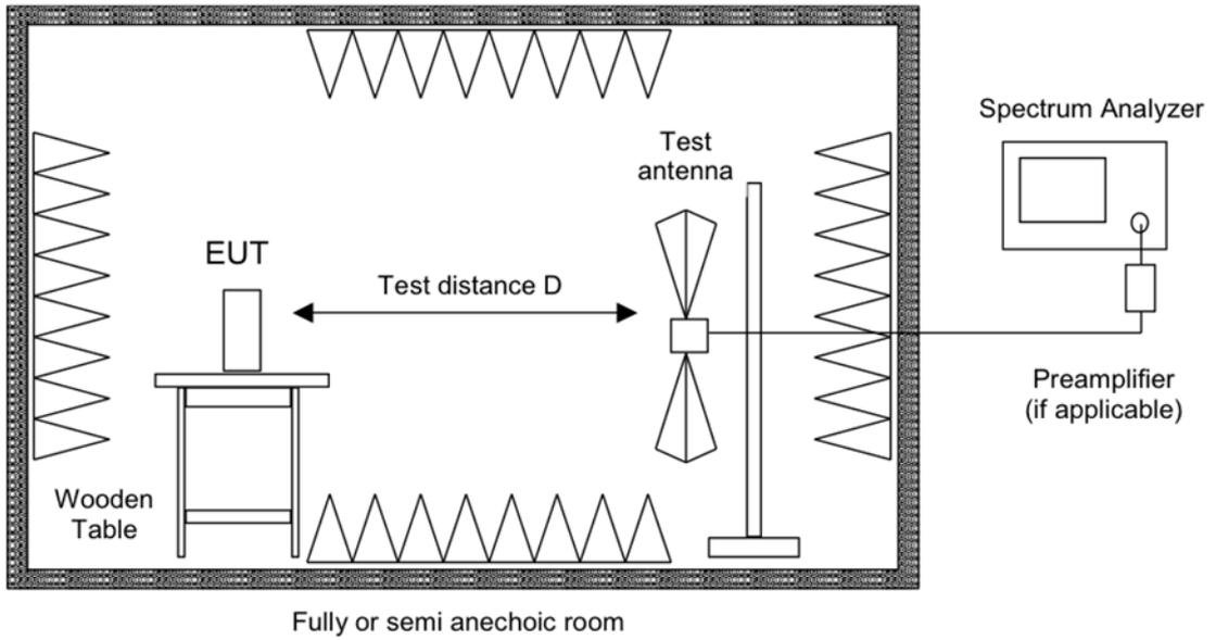
Figure 5: Setup for radiated emissions test above 1 GHz
