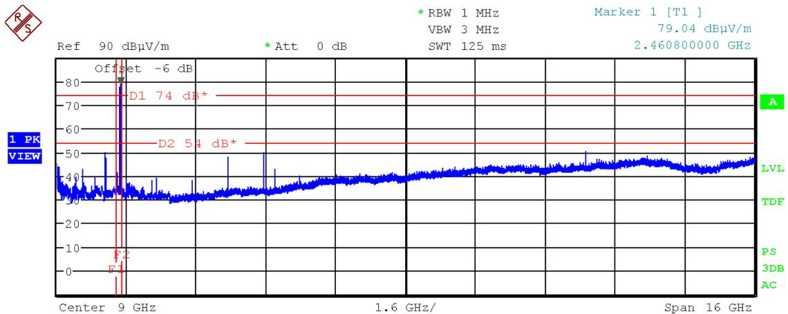
Figure 75: Chart of emissions test from 1 GHz to 17 GHz on highest channel, EUT position Z, antenna polarization horizontal
