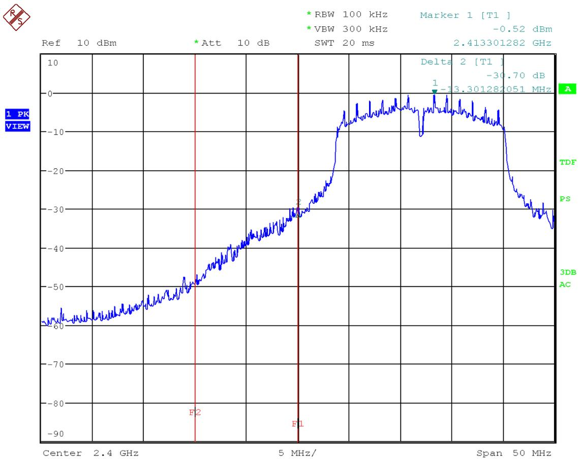
Figure 45: Chart of band-edge measurement on lowest channel, IEEE 802.11 g
