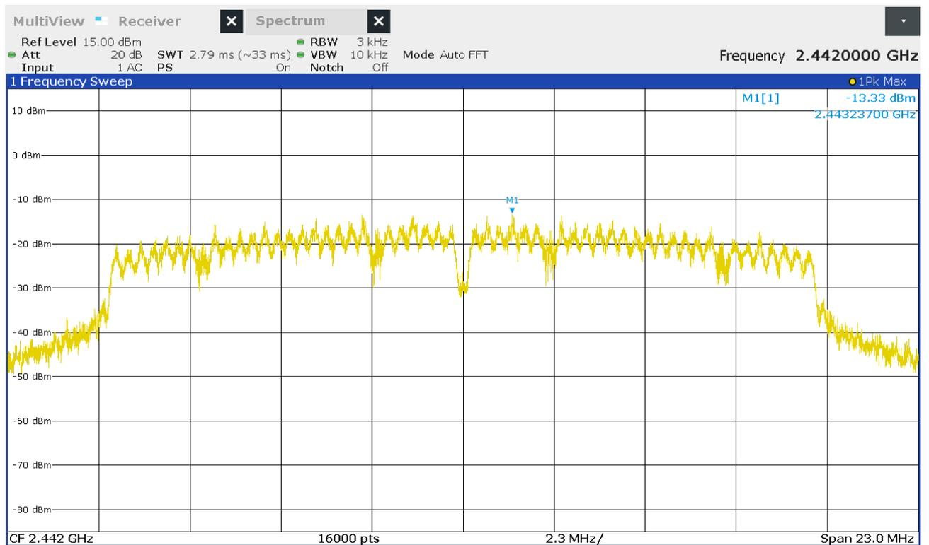
Figure 40: Chart of power spectral density on middle channel, IEEE 802.11 n (HT20)
