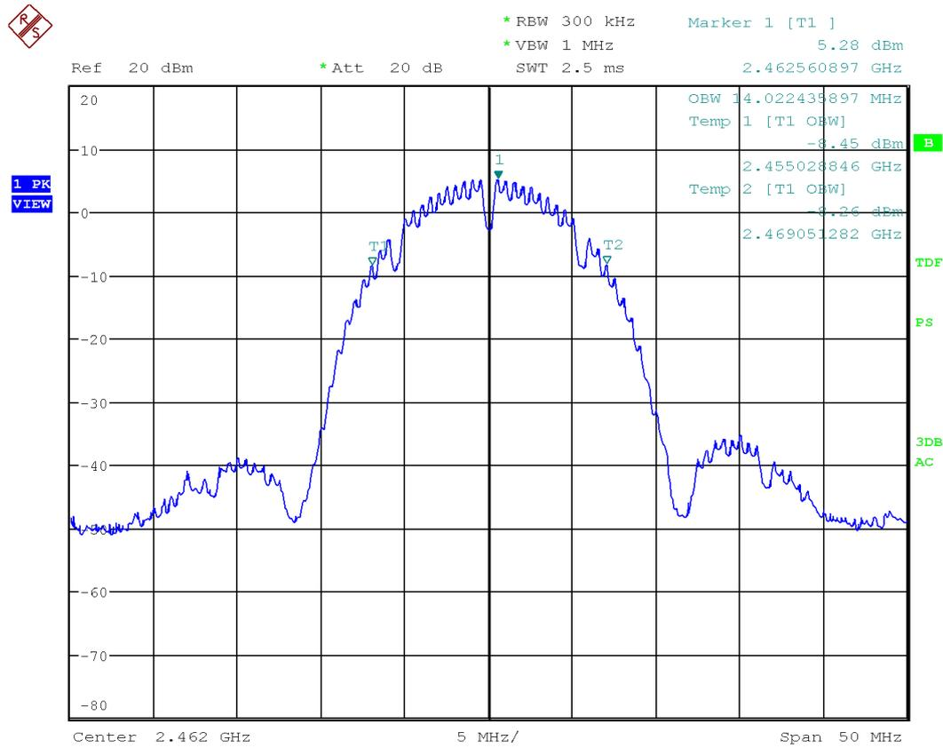
Figure 17: Chart of occupied bandwidth test on highest channel, IEEE 802.11 b
