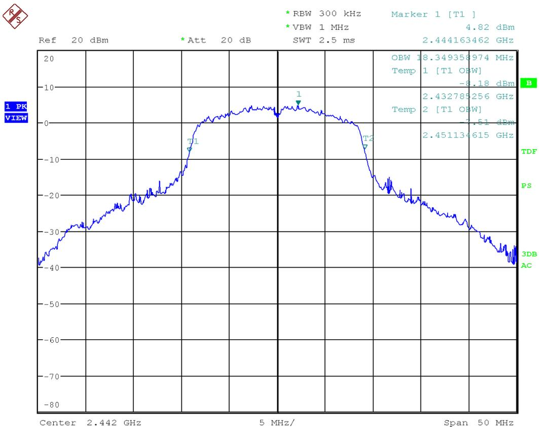
Figure 22: Chart of occupied bandwidth test on middle channel, IEEE 802.11 n (HT20)
