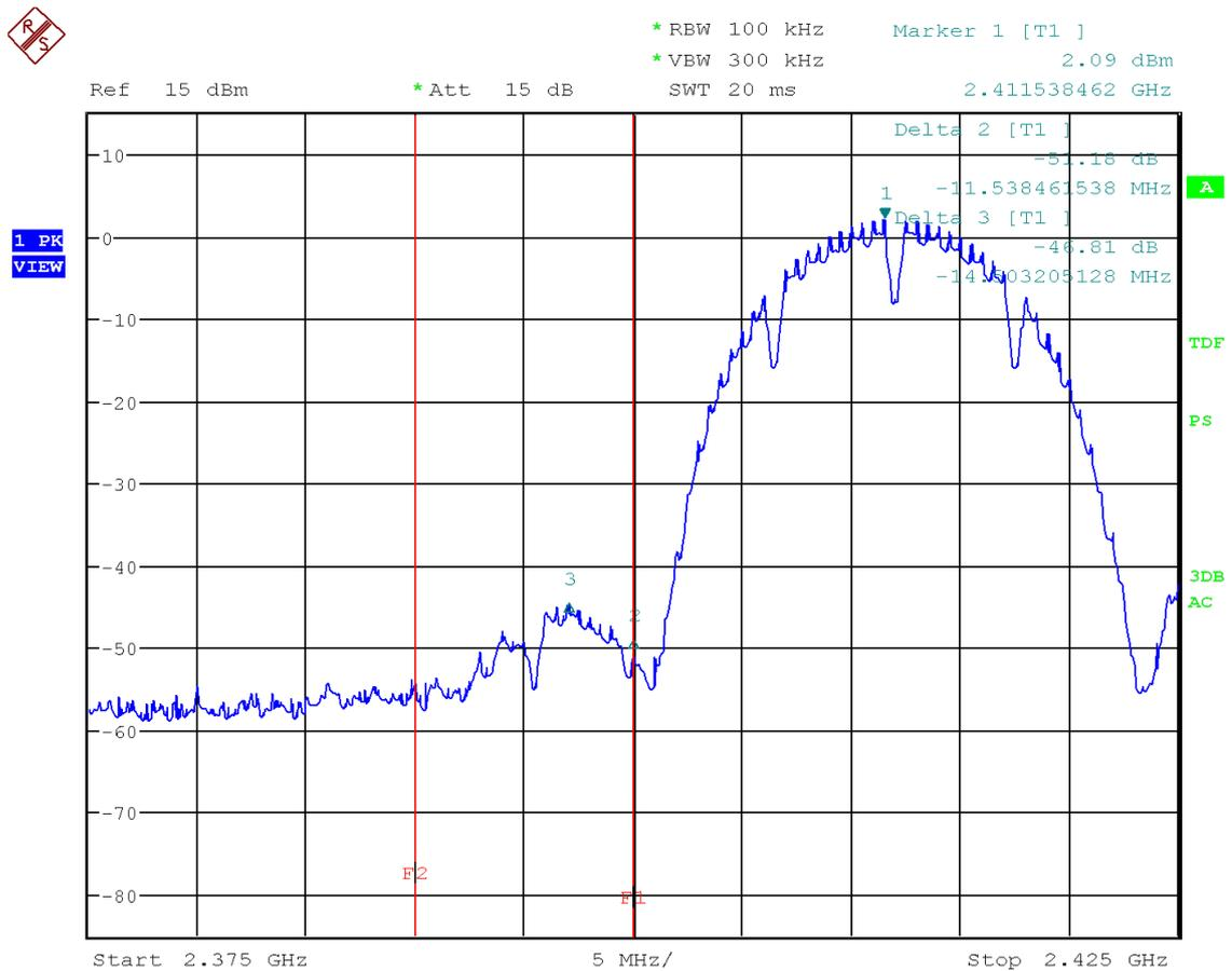
Figure 42: Chart of band-edge measurement on lowest channel, IEEE 802.11 b
