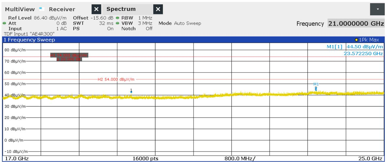
Figure 76: Chart of exploratory emission test from 17 GHz to 25 GHz on highest channel at 0.5 m
