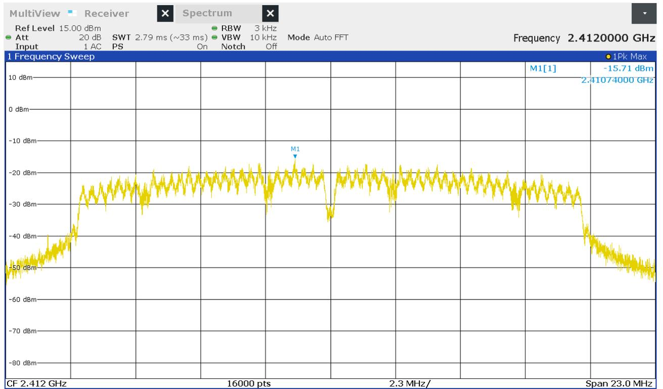
Figure 39: Chart of power spectral density on lowest channel, IEEE 802.11 n (HT20)
