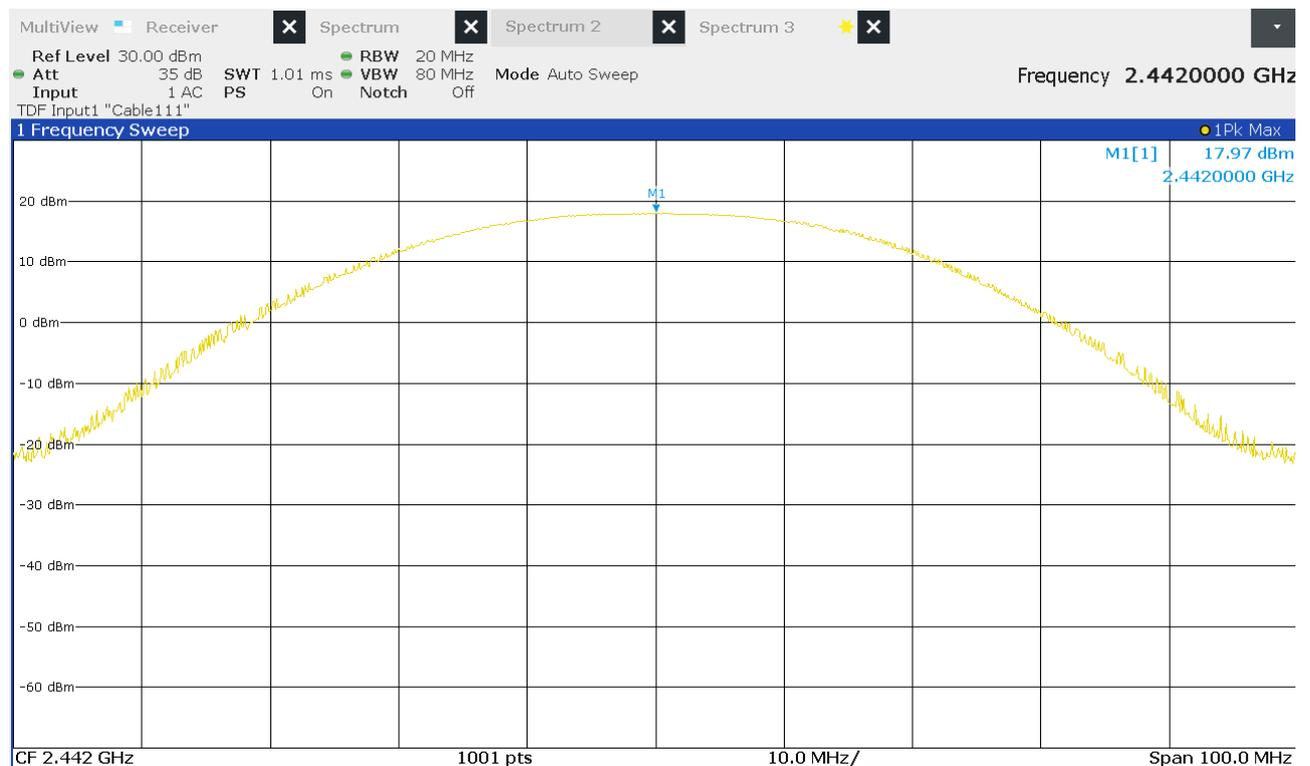
Figure 31: Chart of conducted output power on middle channel, IEEE 802.11 n (HT20)
