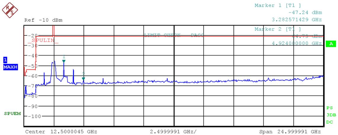
Figure 67: Chart of emissions test from 9 kHz to 25 GHz on highest channel, PK-detector, IEEE 802.11 n (HT20)
