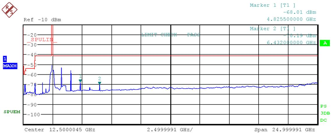
Figure 58: Chart of emissions test from 9 kHz to 25 GHz on lowest channel, RMS-detector, IEEE 802.11 g
