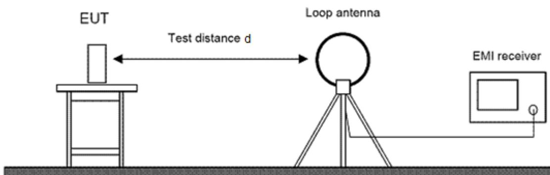
Figure 3: Setup for radiated emissions test below 30 MHz
