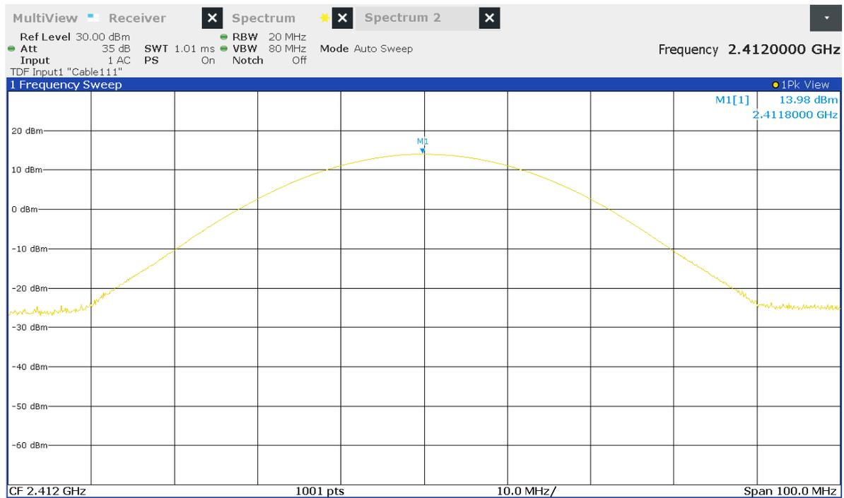
Figure 24: Chart of conducted output power on lowest channel, IEEE 802.11 b
