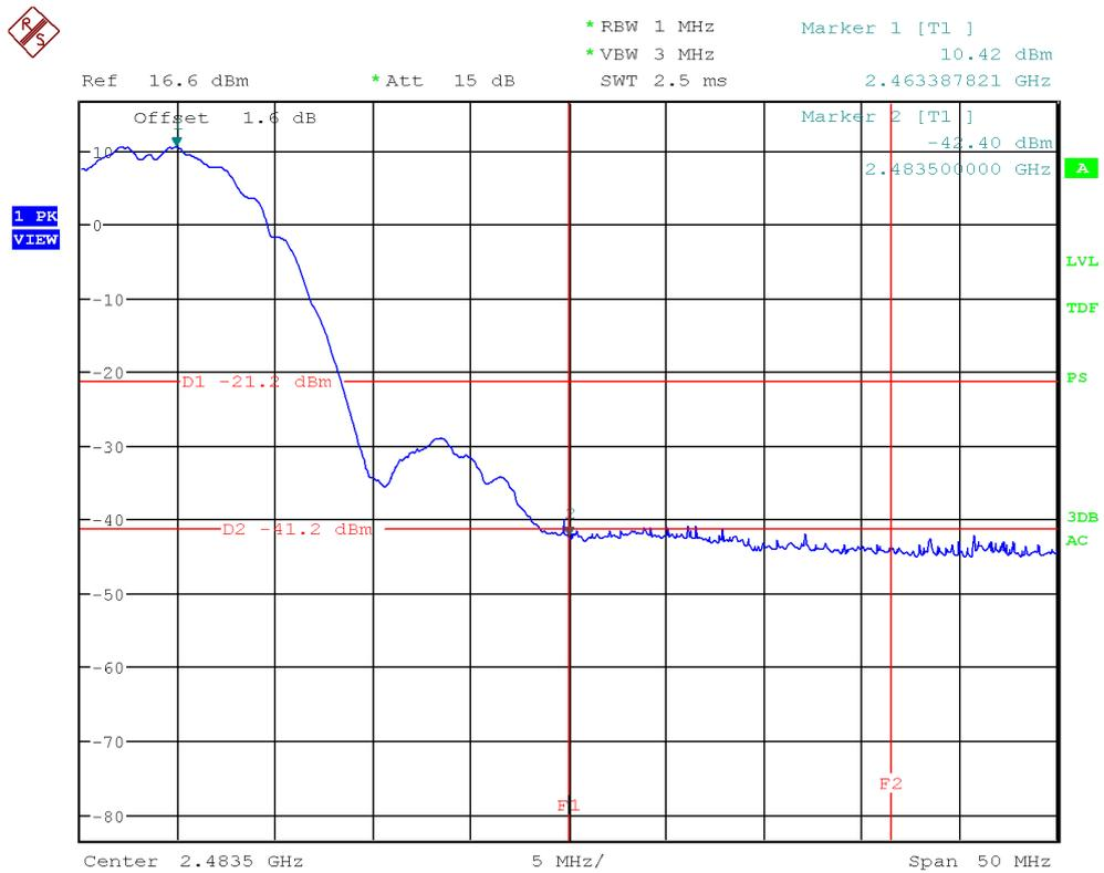
Figure 43: Chart of band-edge measurement on highest channel (PK), IEEE 802.11 b
