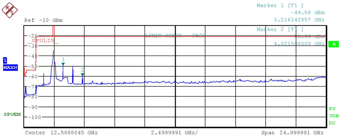
Figure 57: Chart of emissions test from 9 kHz to 25 GHz on lowest channel, PK-detector, IEEE 802.11 g
