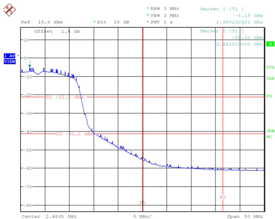
Figure 47: Chart of band-edge measurement on highest channel (AV), IEEE 802.11 g
