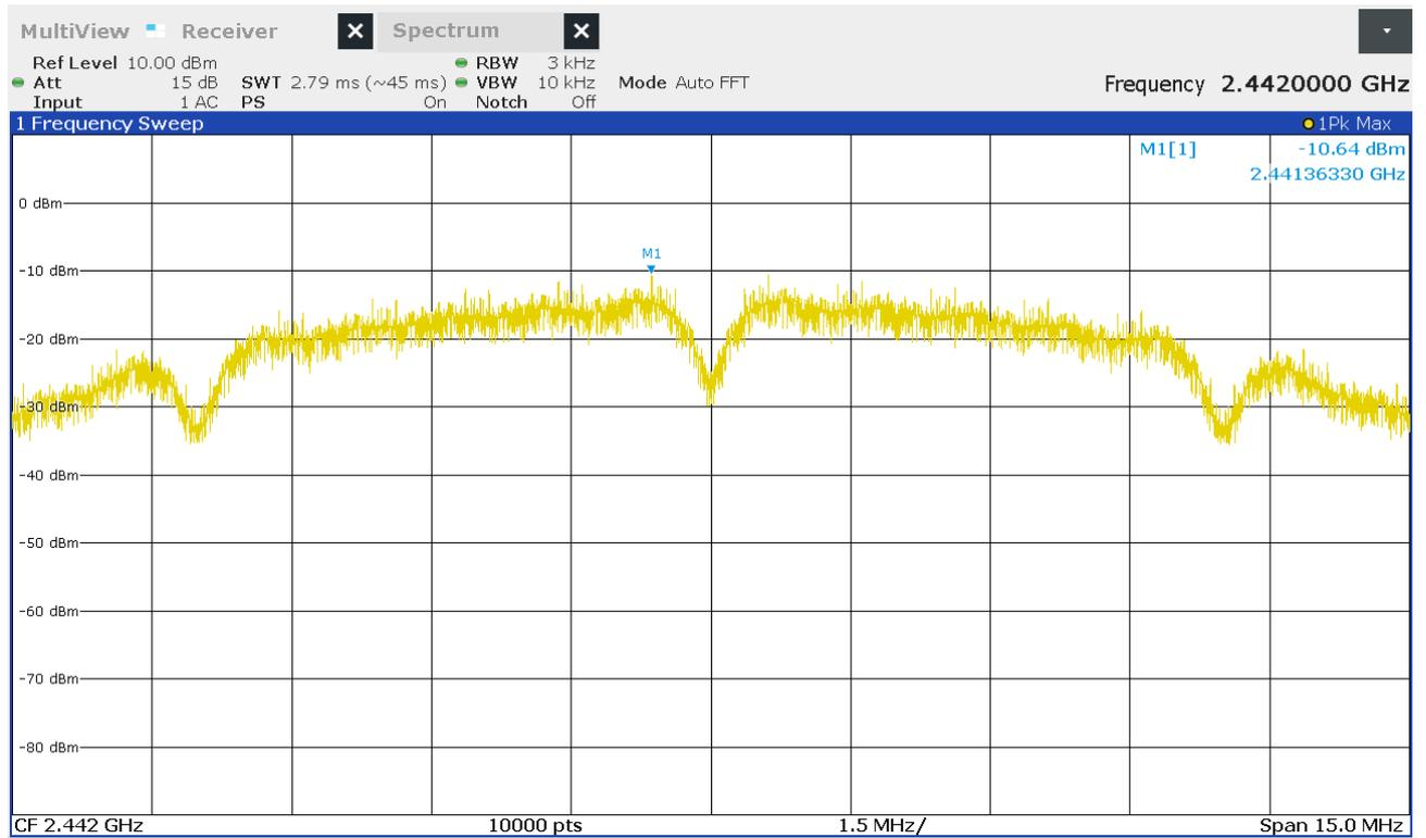
Figure 34: Chart of power spectral density on middle channel, IEEE 802.11 b
