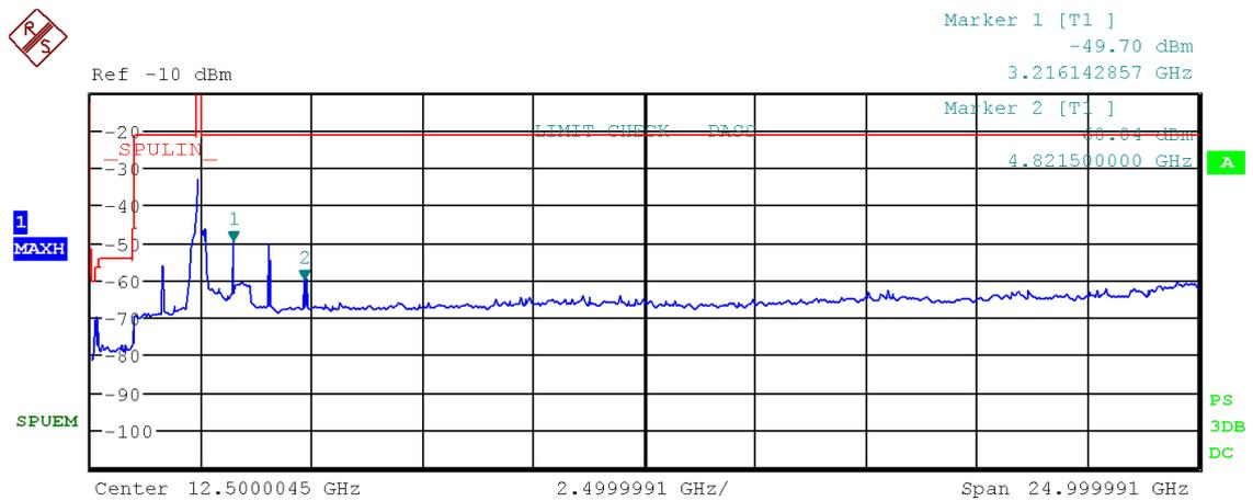
Figure 63: Chart of emissions test from 9 kHz to 25 GHz on lowest channel, PK-detector, IEEE 802.11 n (HT20)
