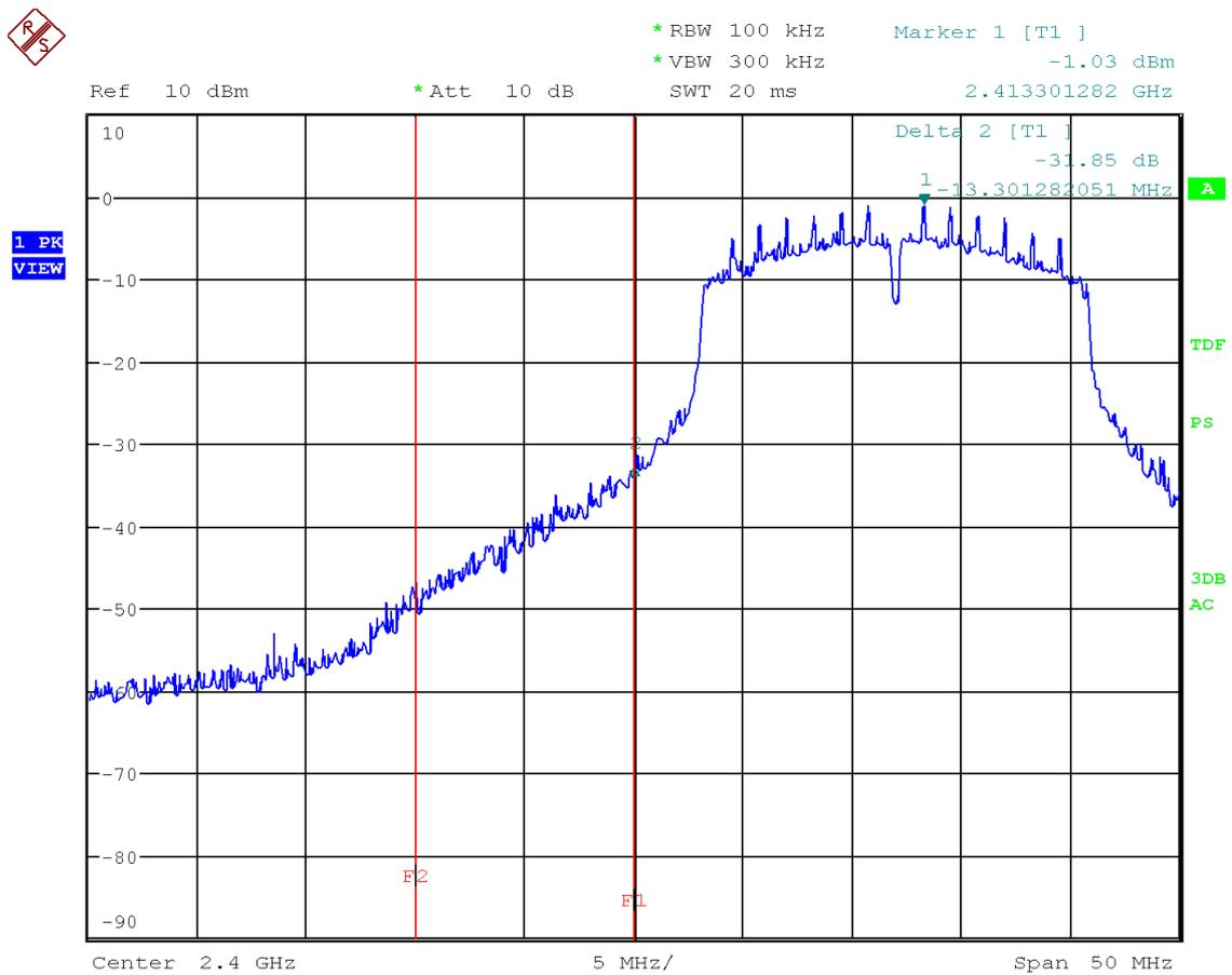
Figure 48: Chart of band-edge measurement on lowest channel, IEEE 802.11 n (HT20)
