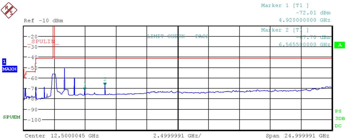
Figure 62: Chart of emissions test from 9 kHz to 25 GHz on highest channel, RMS-detector, IEEE 802.11 g
