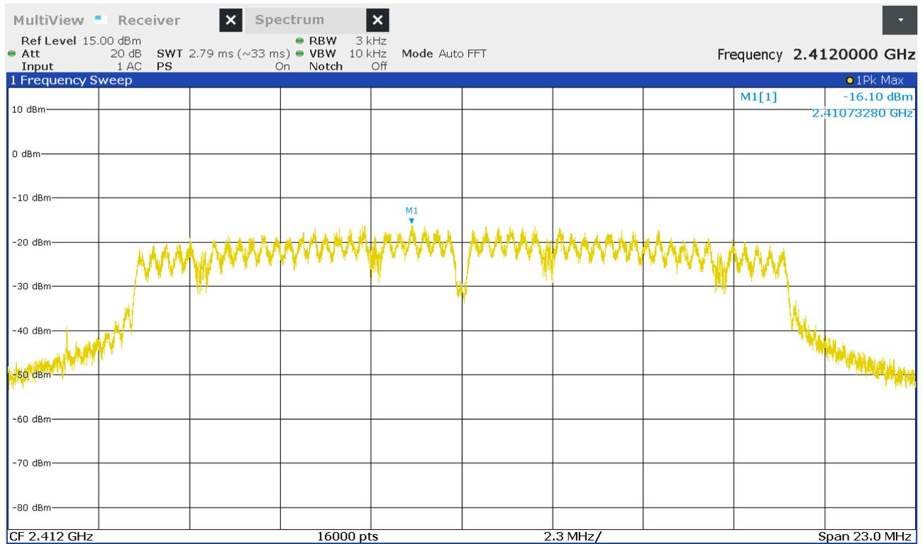
Figure 36: Chart of power spectral density on lowest channel, IEEE 802.11 g
