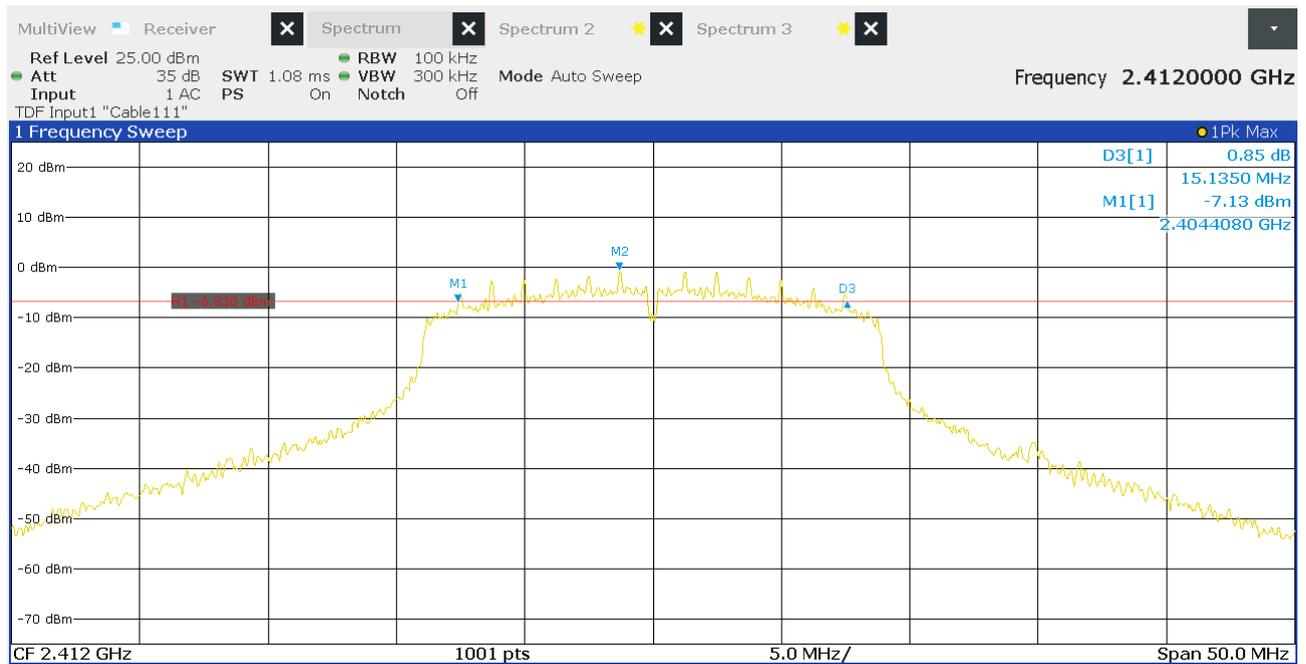
Figure 12: Chart of 6 dB bandwidth test on lowest channel, IEEE 802.11 n (HT20)
