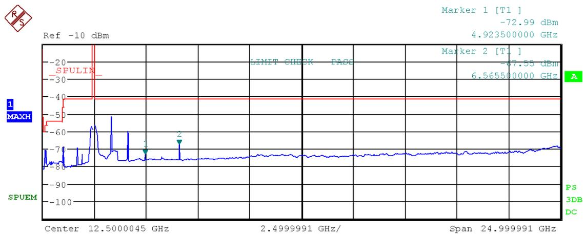
Figure 68: Chart of emissions test from 9 kHz to 25 GHz on highest channel, RMS-detector, IEEE 802.11 n (HT20)
