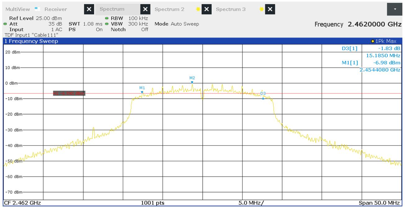
Figure 14: Chart of 6 dB bandwidth test on highest channel, IEEE 802.11 n (HT20)
