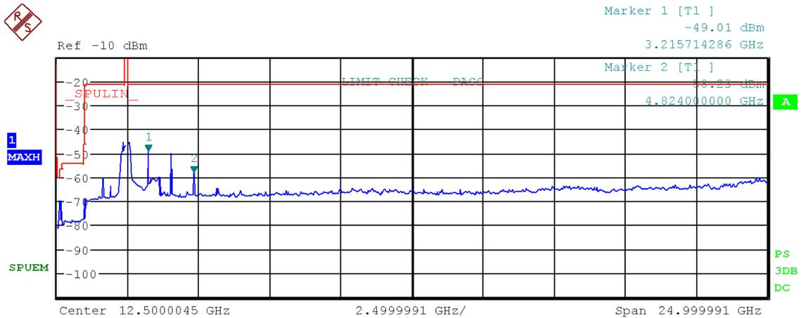
Figure 51: Chart of emissions test from 9 kHz to 25 GHz on lowest channel, PK-detector, IEEE 802.11 b
