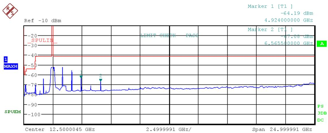
Figure 56: Chart of emissions test from 9 kHz to 25 GHz on highest channel, RMS-detector, IEEE 802.11 b
