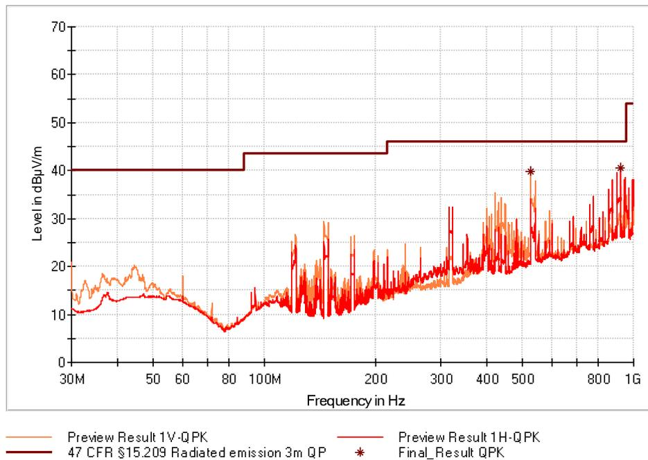
Figure 70: Chart of emissions test from 30 MHz to 1 GHz on lowest channel, EUT position Y
