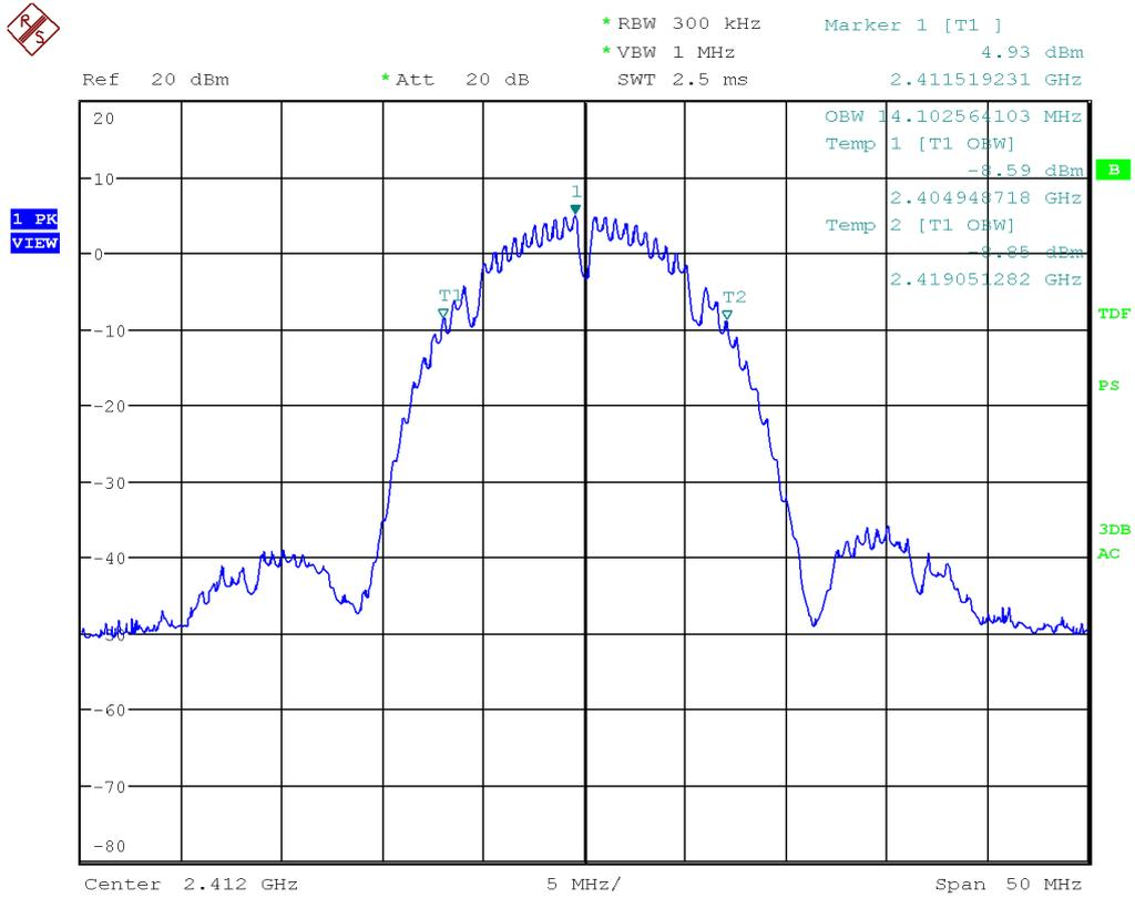
Figure 15: Chart of occupied bandwidth test on lowest channel, IEEE 802.11 b
