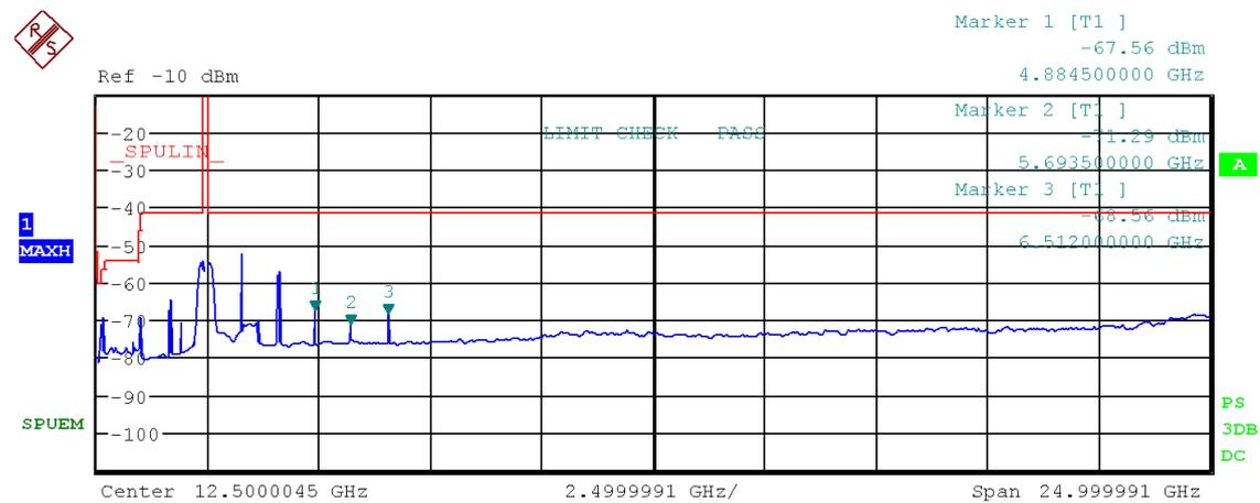
Figure 66: Chart of emissions test from 9 kHz to 25 GHz on middle channel, RMS-detector, IEEE 802.11 n (HT20)
