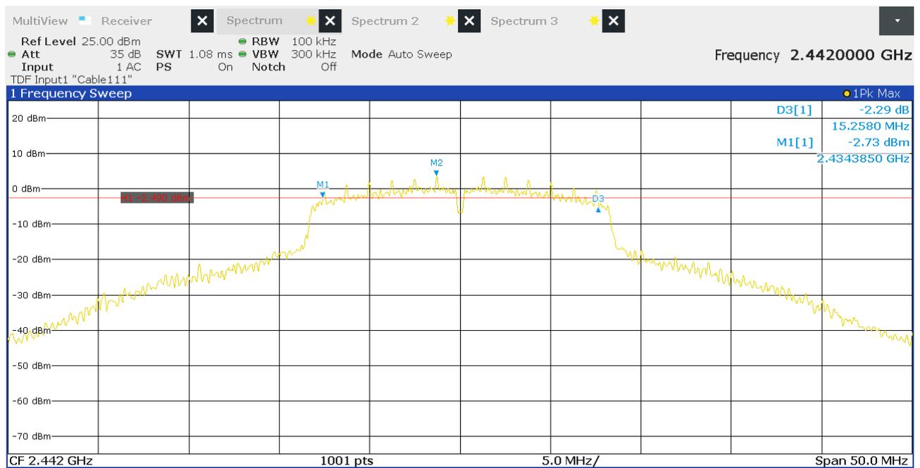
Figure 10: Chart of 6 dB bandwidth test on middle channel, IEEE 802.11 g
