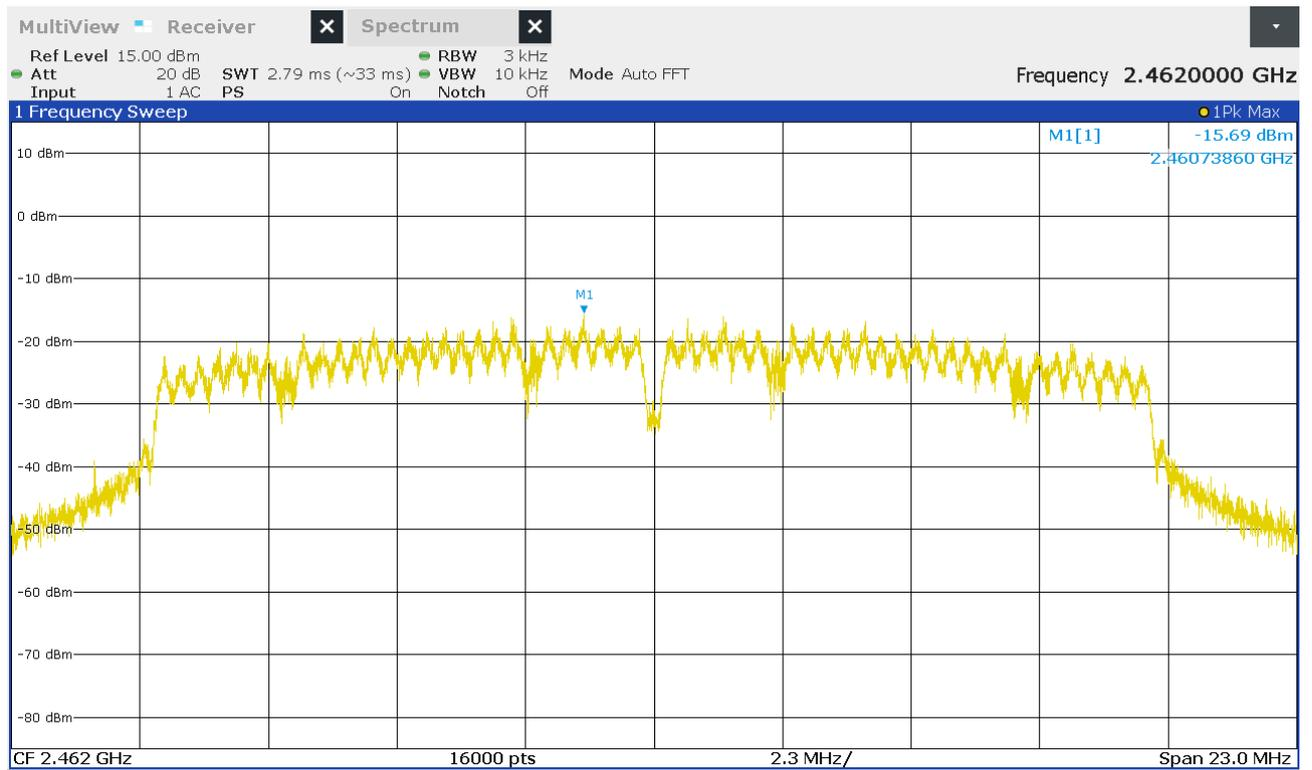
Figure 41: Chart of power spectral density on highest channel, IEEE 802.11 n (HT20)
