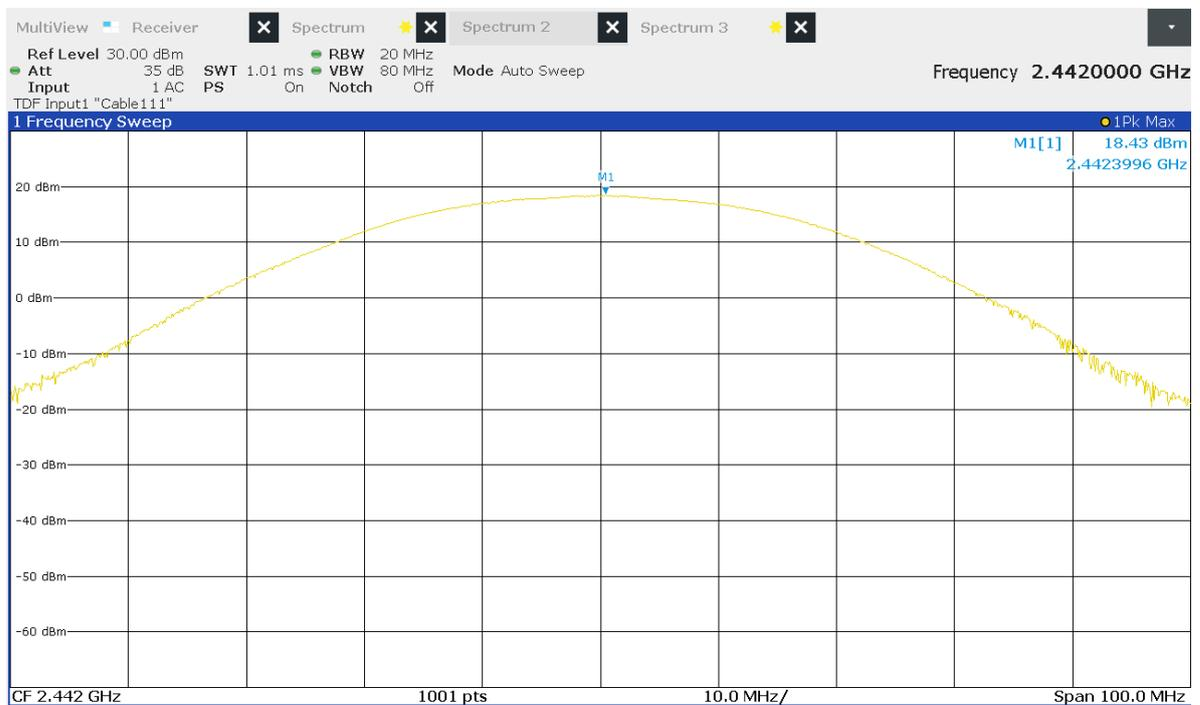
Figure 28: Chart of conducted output power on middle channel, IEEE 802.11 g
