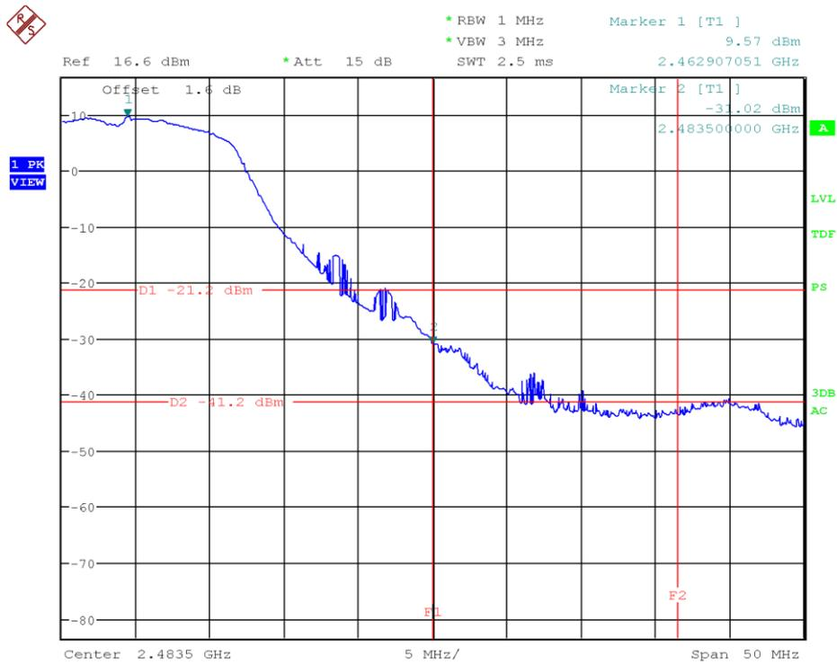
Figure 49: Chart of band-edge measurement on highest channel (PK), IEEE 802.11 n (HT20)
