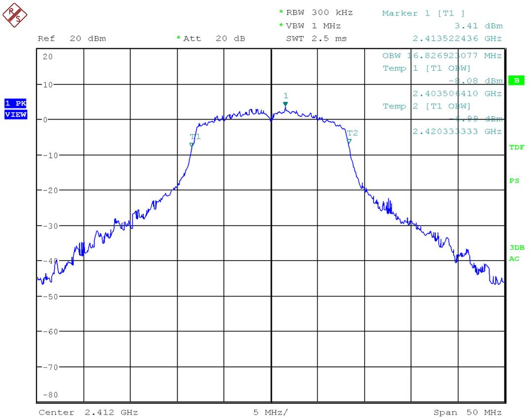
Figure 18: Chart of occupied bandwidth test on lowest channel, IEEE 802.11 g
