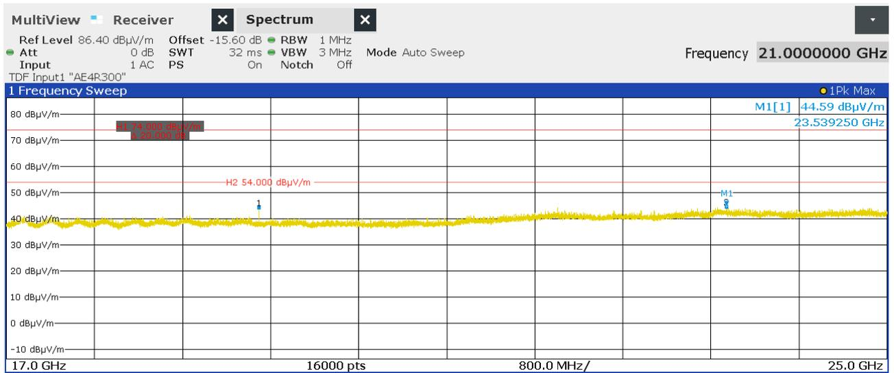
Figure 72: Chart of exploratory emission test from 17 GHz to 25 GHz on lowest channel at 0.5 m
