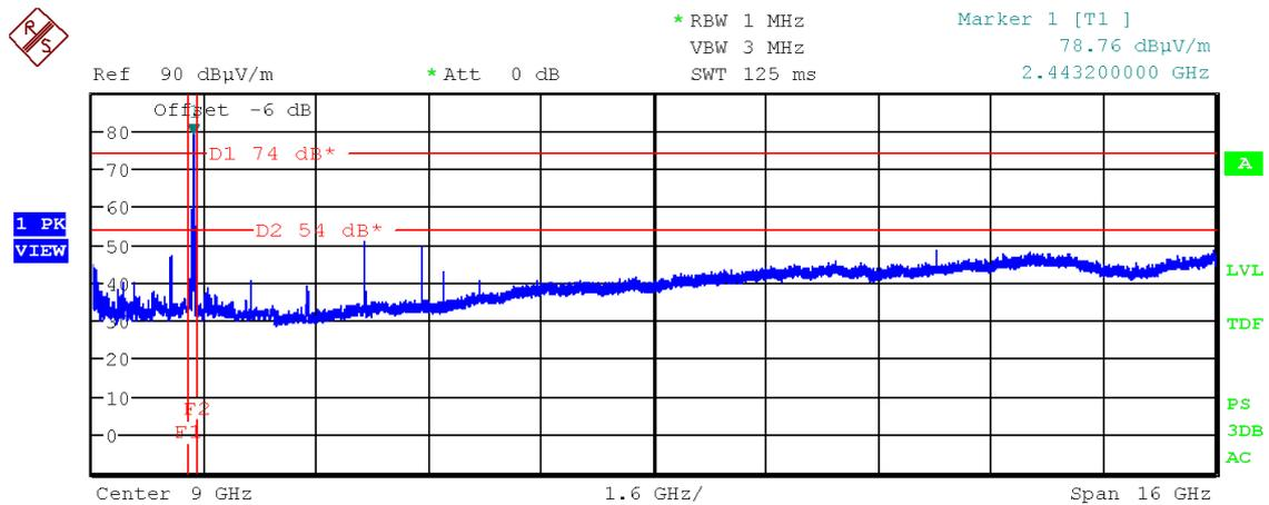
Figure 73: Chart of emissions test from 1 GHz to 17 GHz on middle channel, EUT position Z, antenna polarization horizontal
