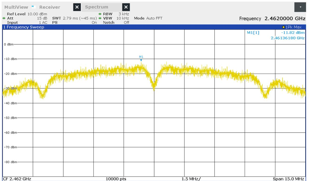
Figure 35: Chart of power spectral density on highest channel, IEEE 802.11 b
