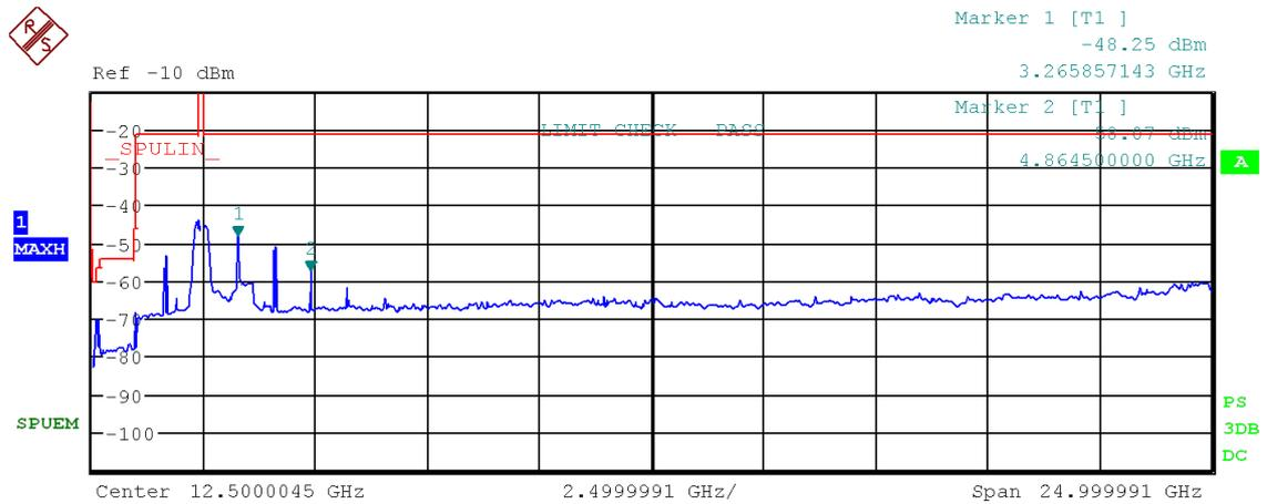
Figure 65: Chart of emissions test from 9 kHz to 25 GHz on middle channel, PK-detector, IEEE 802.11 n (HT20)
