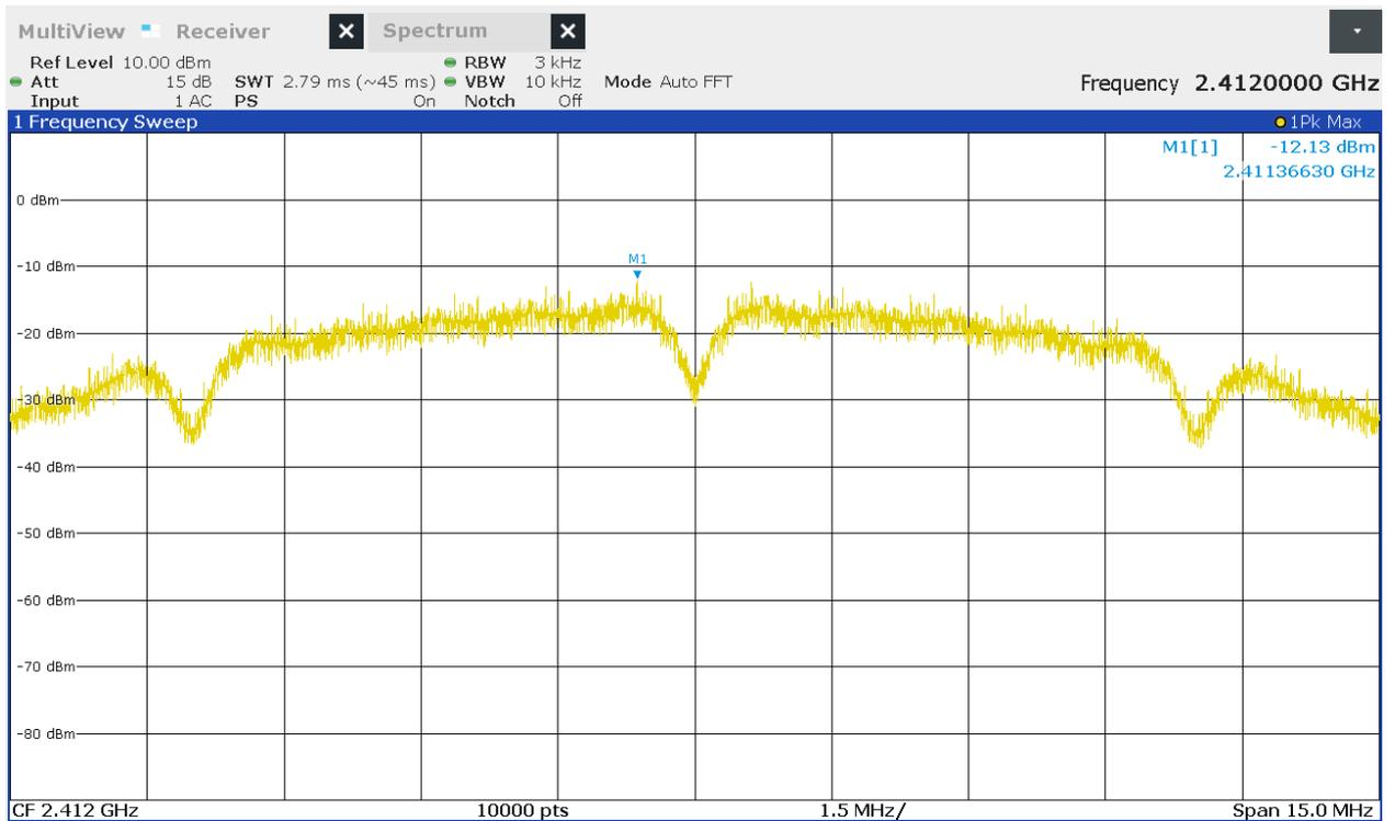
Figure 33: Chart of power spectral density on lowest channel, IEEE 802.11 b
