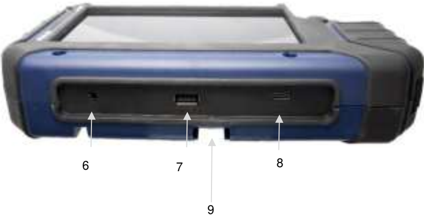
Fig. 8: Monitor bottom with connector strip
