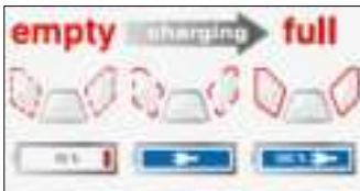
Fig. 19: Keys and charge level indicated when charging
