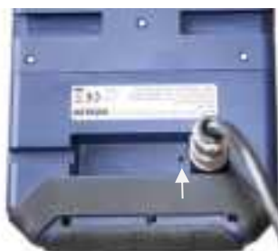
Fig. 69: Reset hole indicated by an arrow
