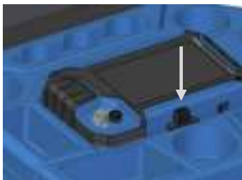
Fig. 11: Press down on the catch from above to lower the monitor into the case.
