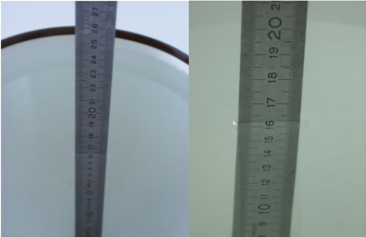
Fig. 28: Liquid depth for PCS 1900 Head and Body measurements.
