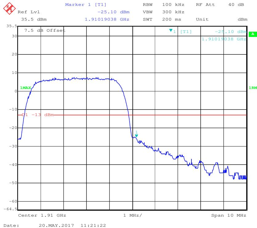
**PCS Band, Left Band Edge for HSUPA (BPSK) Mode**
