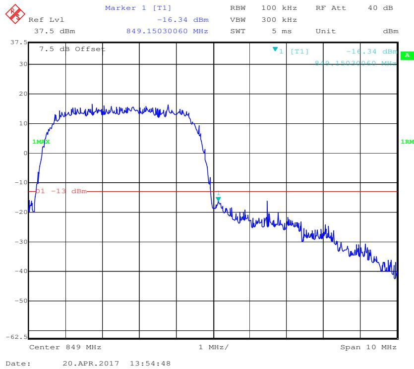
**PCS Band, Left Band Edge for GSM (GMSK) Mode**
