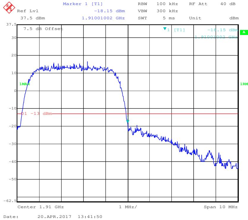
**PCS Band, Left Band Edge for HSDPA (16QAM) Mode**
