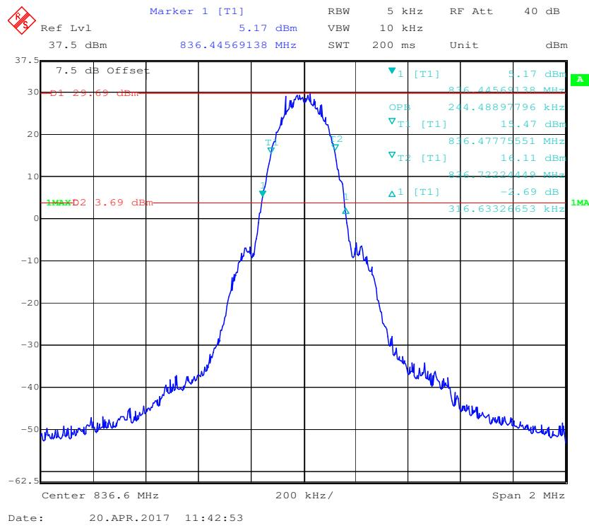
**99% Occupied Bandwidth & 26 dB Emissions Bandwidth for RMC (BPSK) Mode**
