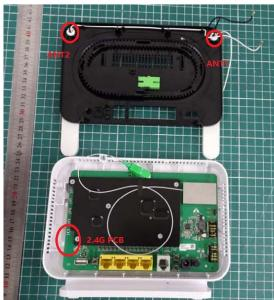
ANT1 with two short feeders ANT2 with two long feeders The white feeder is 2.4G, while the black feeder is 5G
