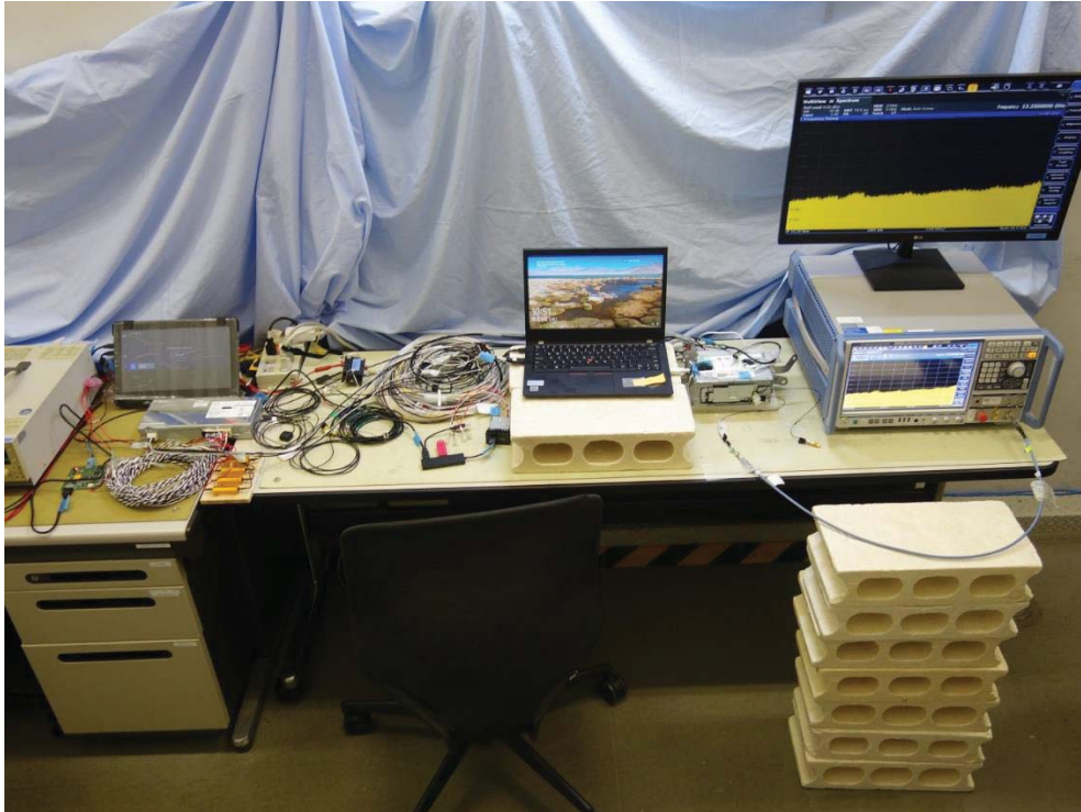
Photograph 5: Set-up for Antenna Port Connected Test
