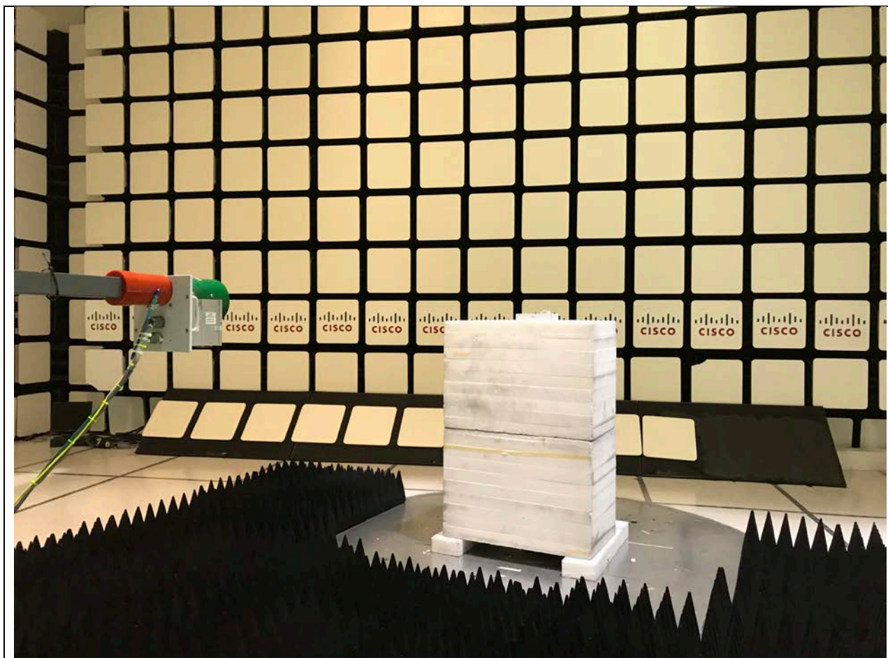
Title: Radiated Emissions 18-40GHz Configuration Photograph
