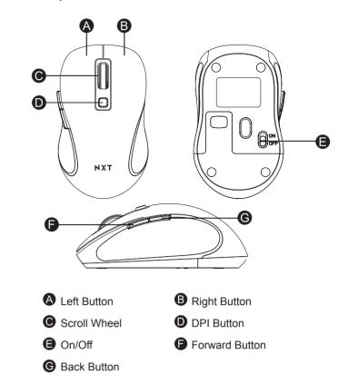
Click the DPI button to switch the DPI, the LED beneath the scroll wheel will flash once twice and three times to show this 3 levels DPI.
