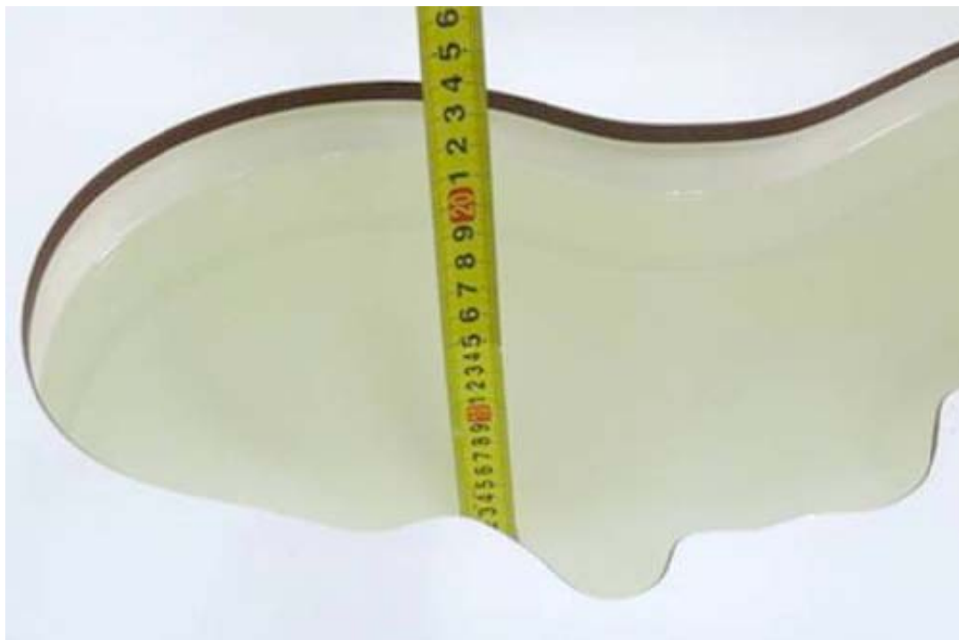
Picture 3: liquid depth in the head Phantom
