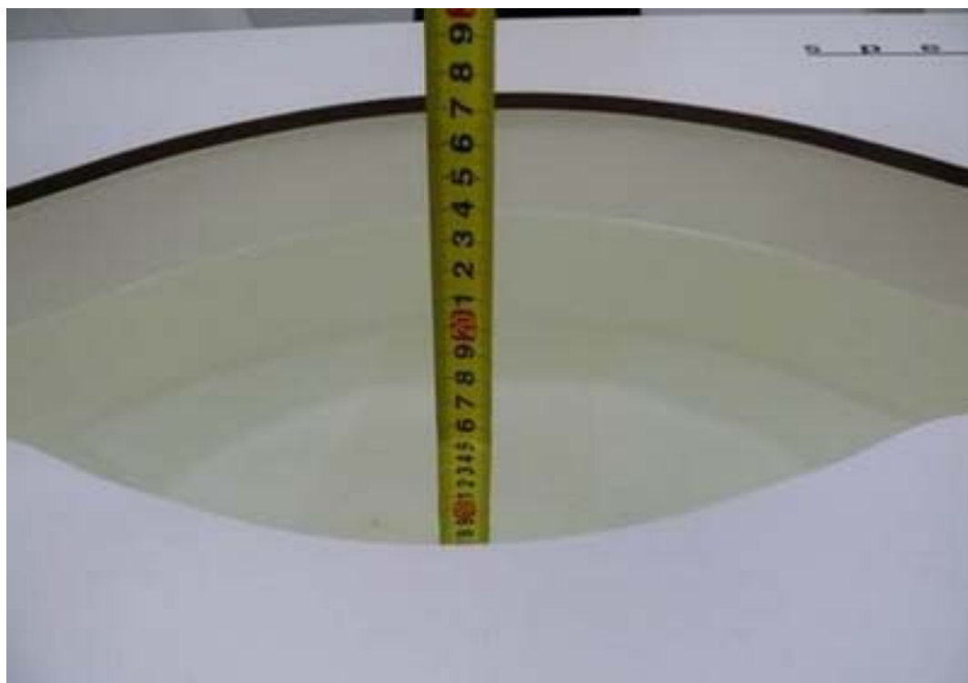
Picture 4: Liquid depth in the flat Phantom
