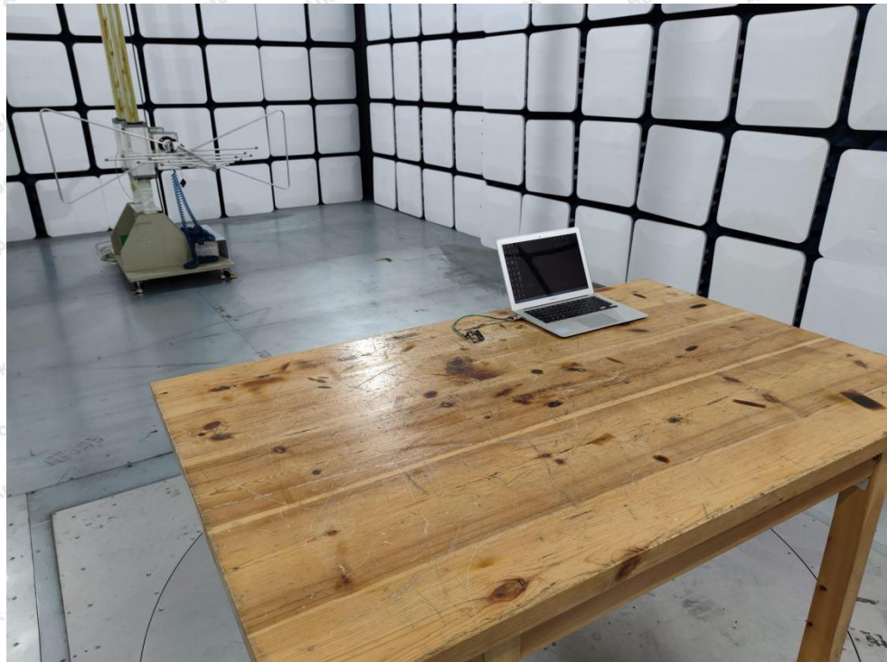
Photo of Radiation Emission Test
