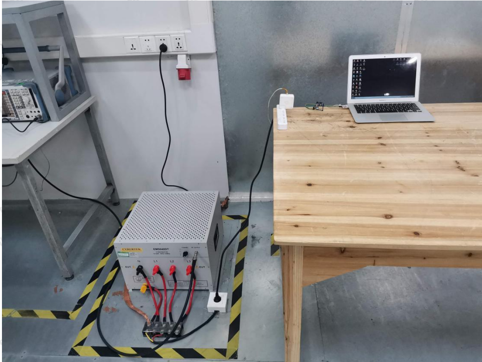
Photo of Power Line Conducted Emission Test
