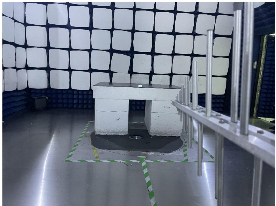
Radiation Emission Test Setup (30MHz to 1GHz)
