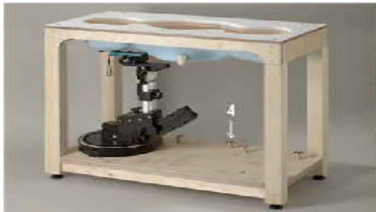
Figure 4 SAM Twin Phantom
