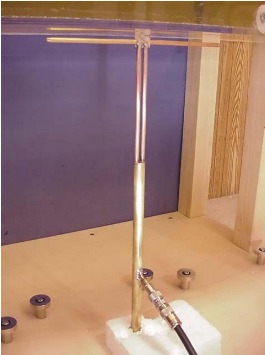
450MHz Dipole Calibration Photo
