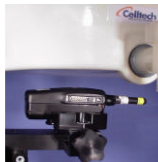
Face-held SAR Test Setup 2.5cm Separation Distance
