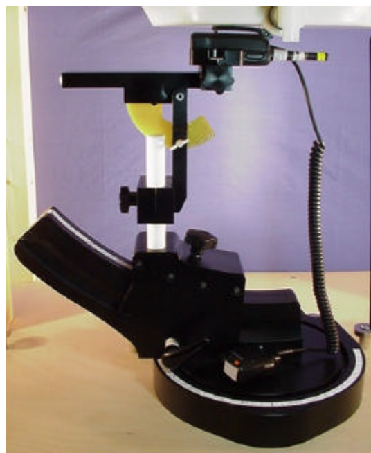
Body SAR Test Setup with SAM Planar Phantom
