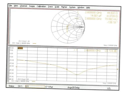
Impedance Measurement Plot for Body TSL
