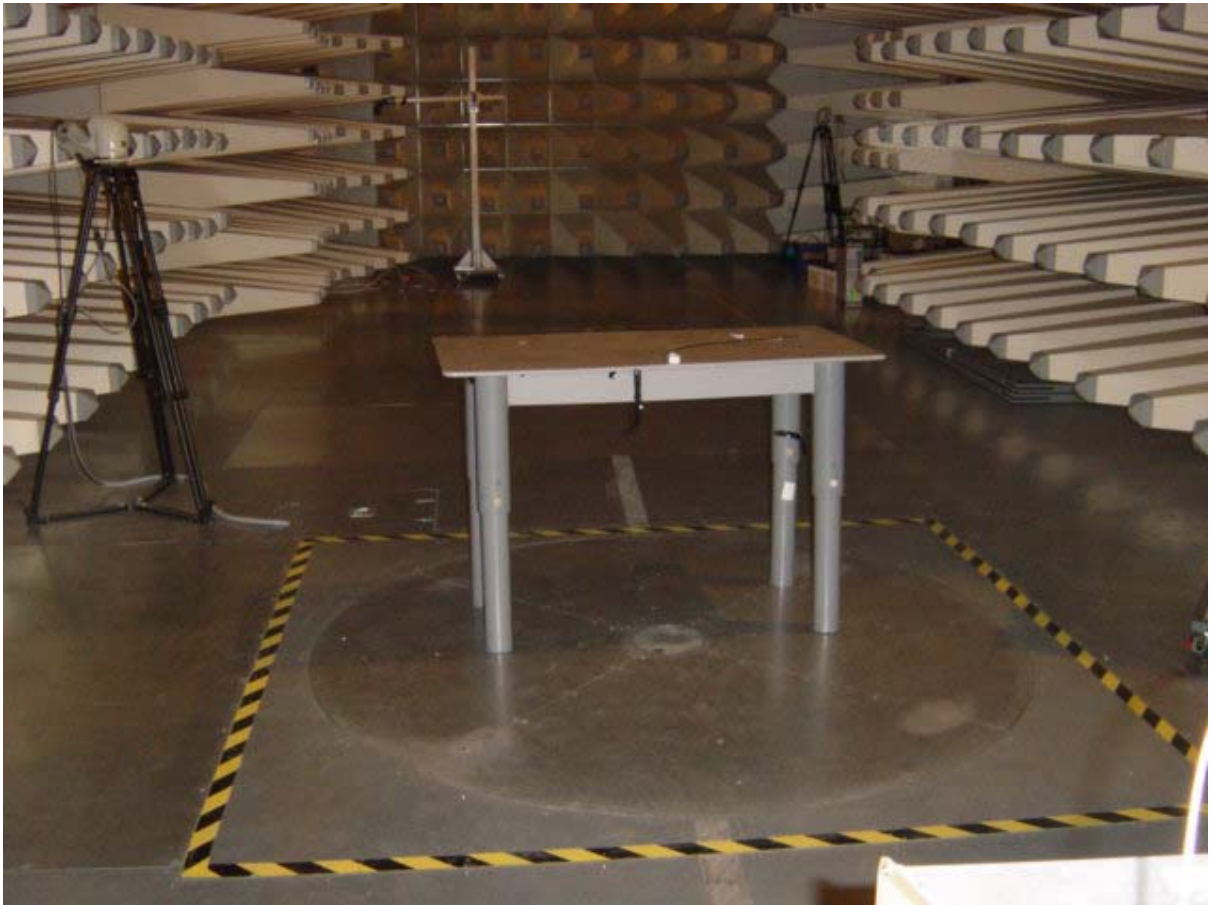
Set-up for Radiation Emission (Transceiver)
