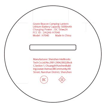
The label shown shall be permanently affixed at a conspicuous location on the device and be readily visible to the user at the time purchase (Labeling requirements per 2.925)
