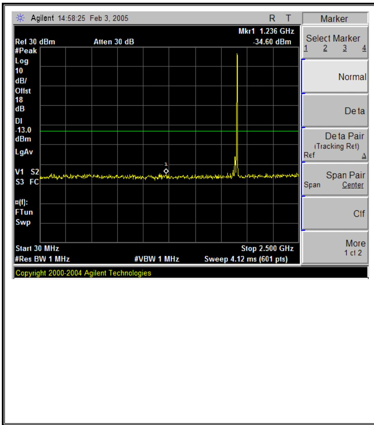
**PCS CDMA Modulation: High Channel Out-Of-Band Emissions**
