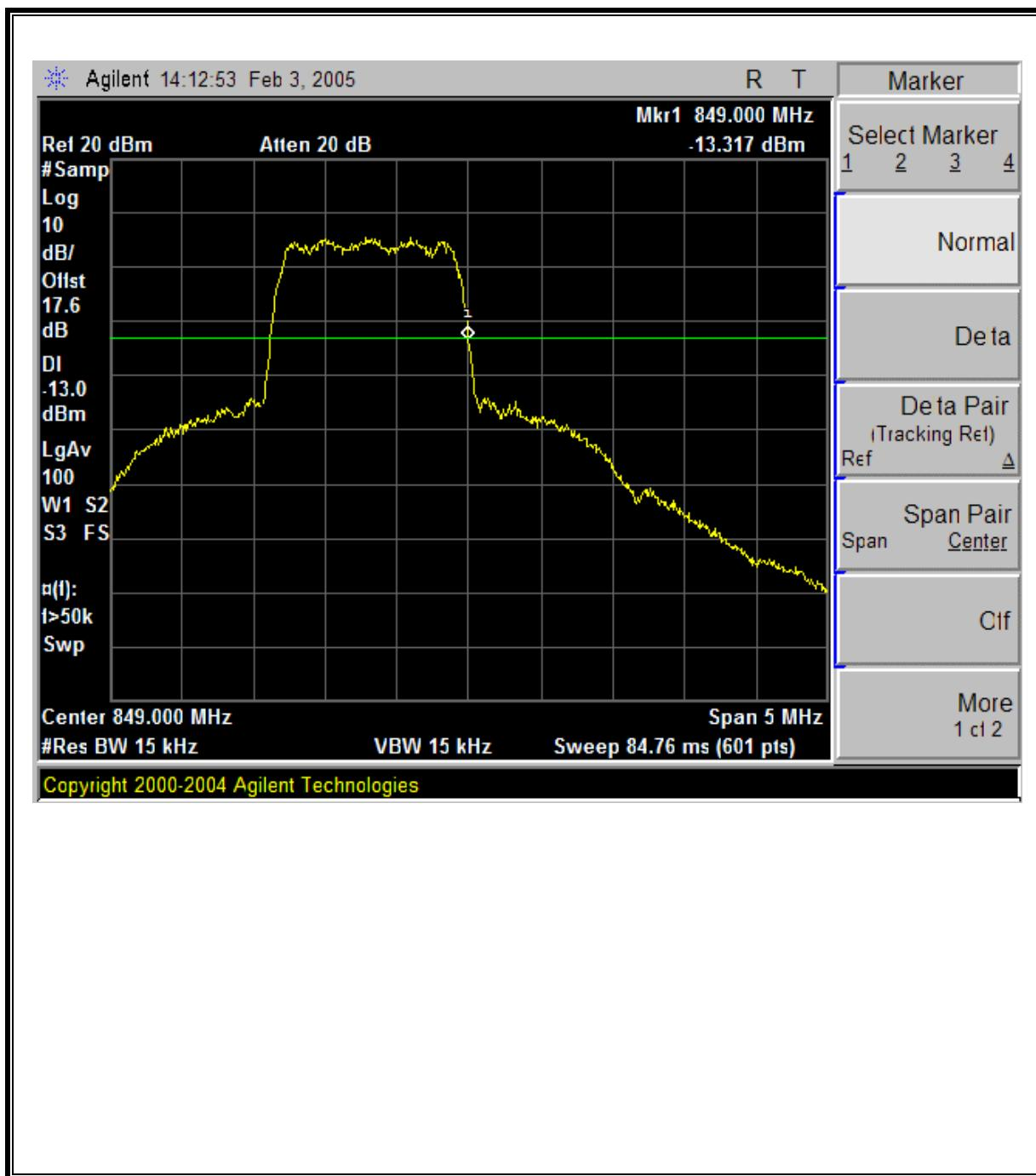
**800MHZ CELL CDMA Mobile Emissions in Base Frequency Range**
