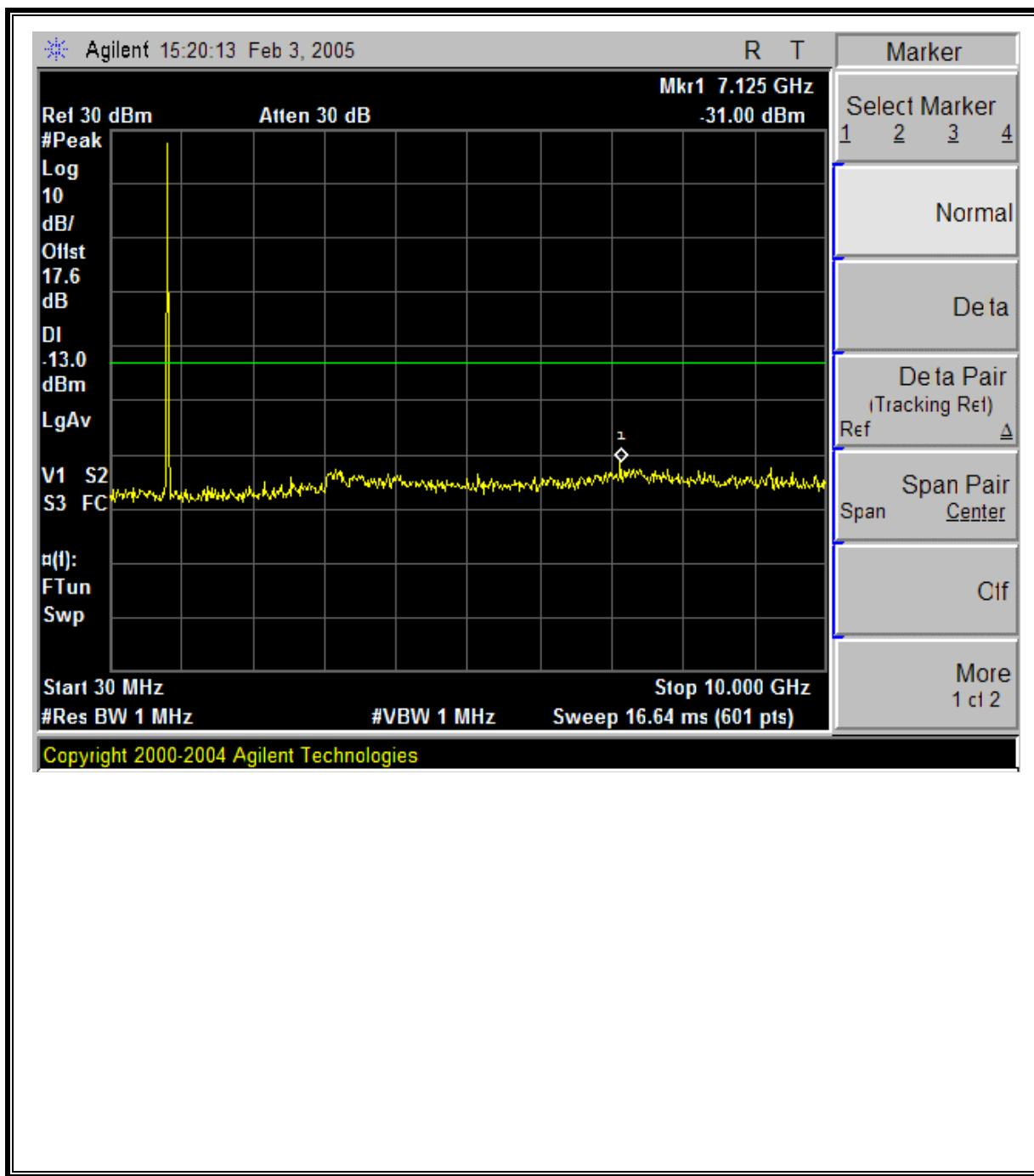
**CDMA Modulation: High Channel, Out-Of-Band Emissions**
