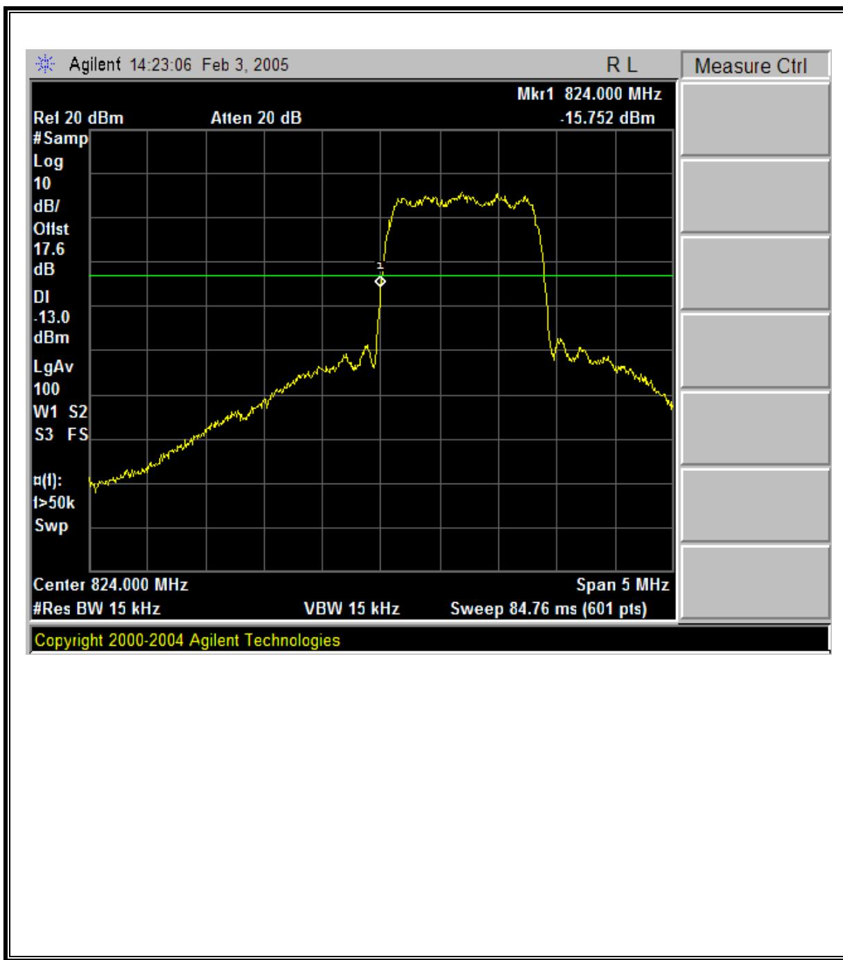
**800MHZ CELL CDMA Modulation: High Channel Band Edge**
