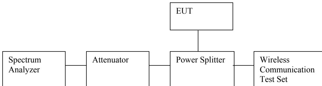
**RADIATED TEST SETUP DIAGRAM**
