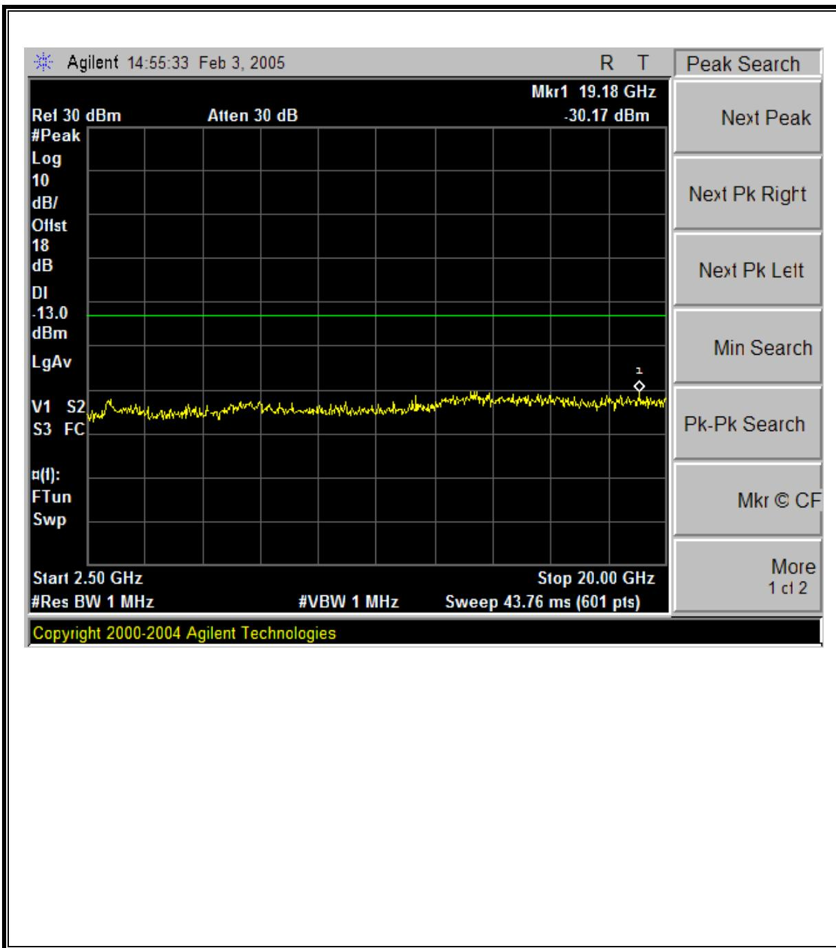
**PCS CDMA Modulation: High Channel Out-Of-Band Emissions #1**
