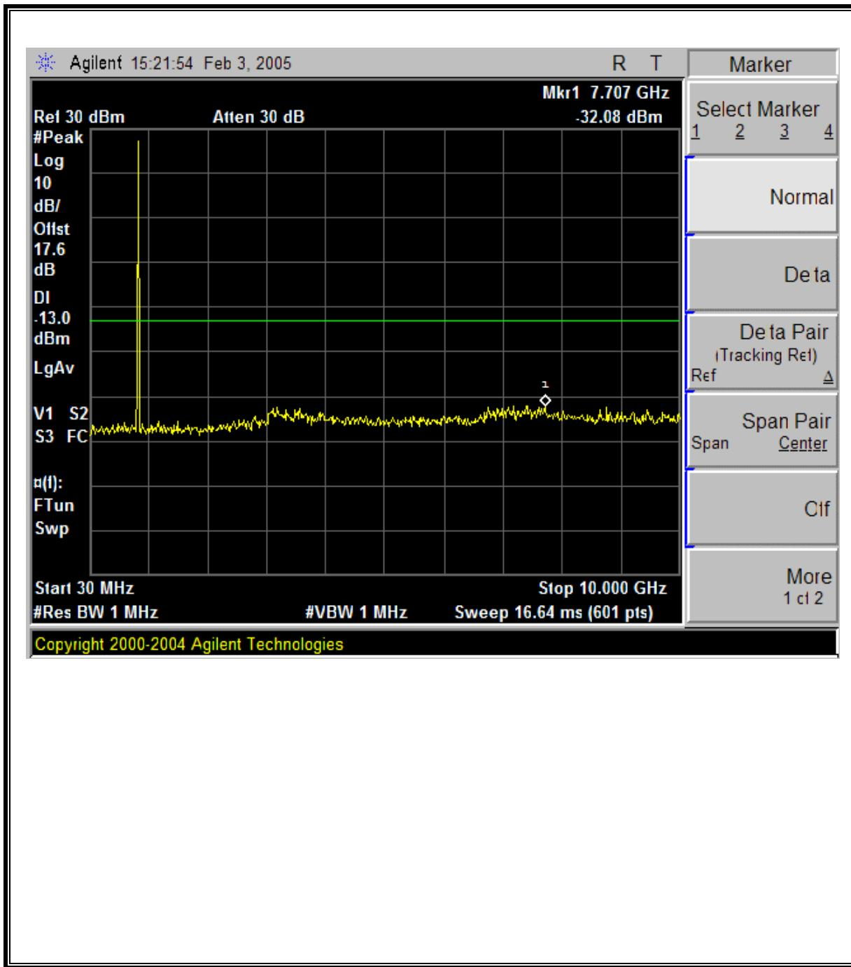
**800MHz CELL CDMA Modulation: Low Channel Band Edge**
