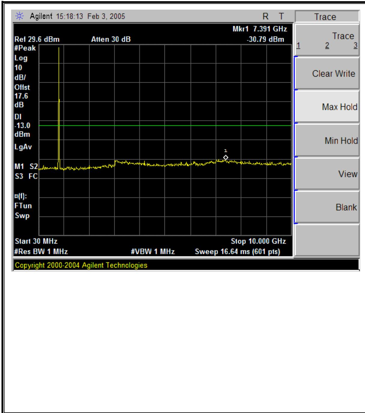
**CDMA Modulation: Mid Channel, Out-Of-Band Emissions**
