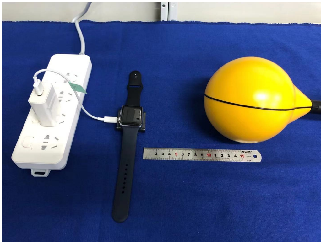
Photograph 4: Set-up for RF Exposure
