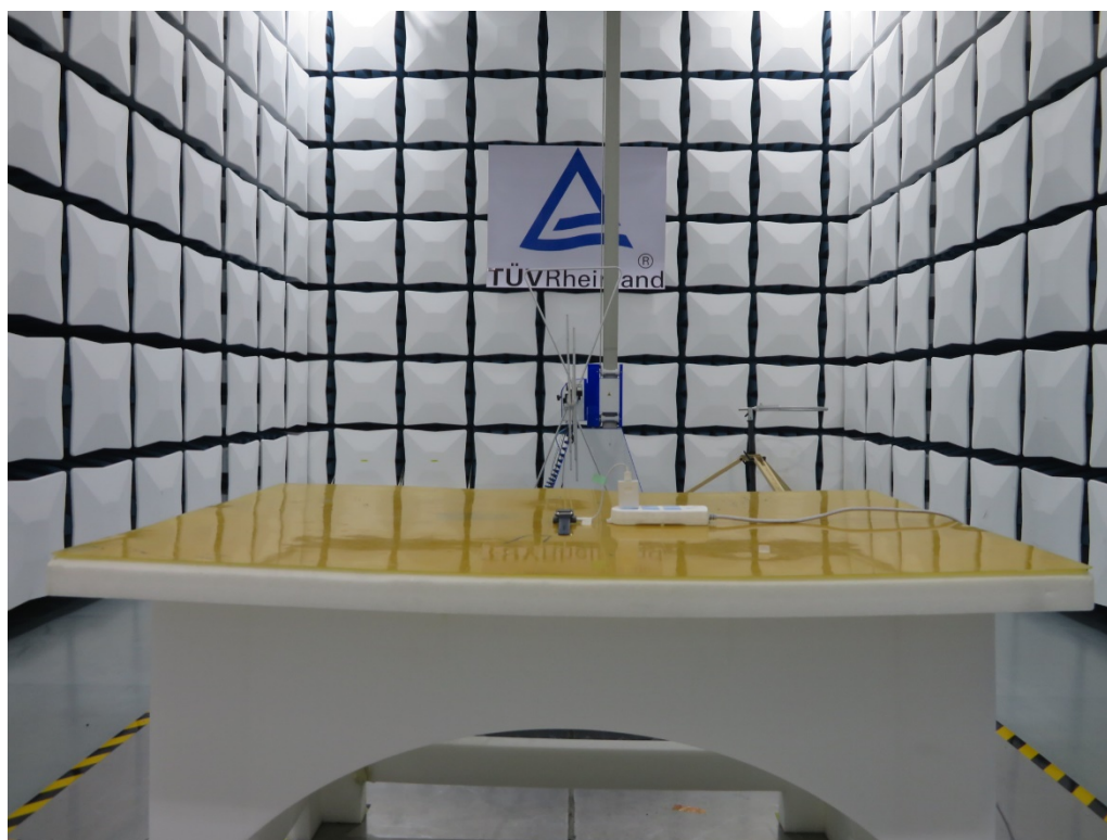
Photograph 2: Set-up for Radiated Spurious Emission, Above 1GHz
