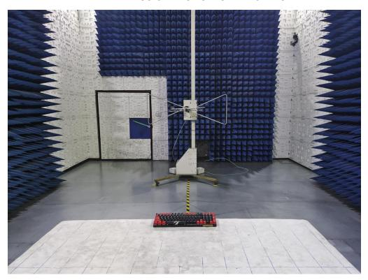
RADIATED EMISSION TEST SETUP ABOVE 1GHz
