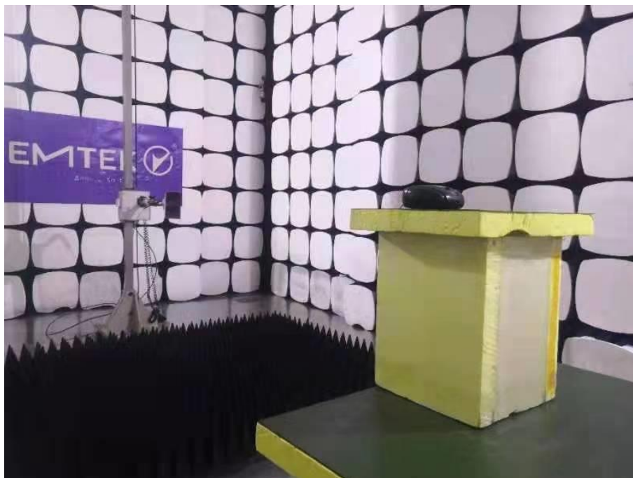
Spurious Emission Test Setup (Above 1GHz)
