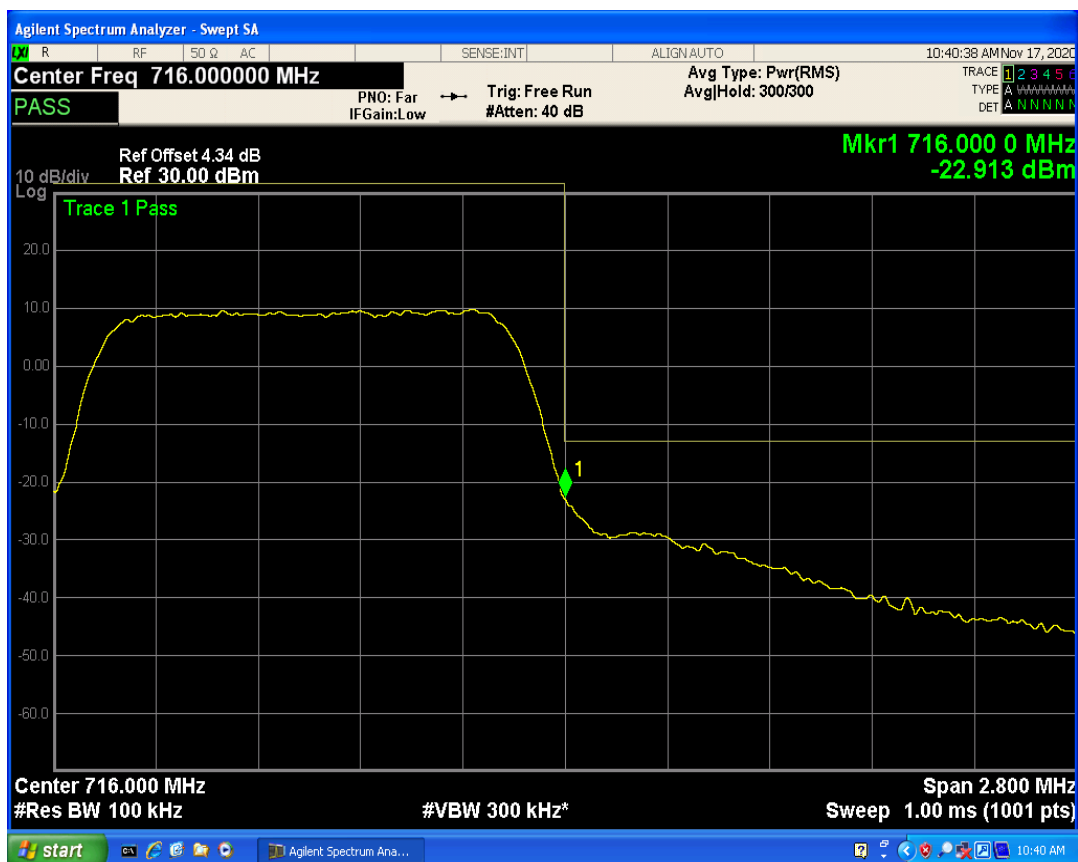
LTE Band12 QPSK BW=10MHz Channel=23060 RB Size=1 Position=#0
