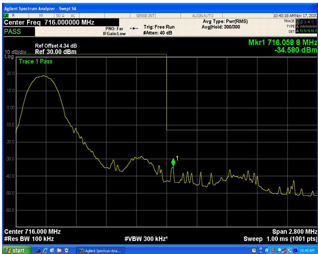
LTE Band12 QPSK BW=1.4MHz Channel=23173 RB Size=1 Position=#Max
