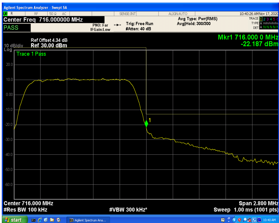
LTE Band12 QAM16 BW=1.4MHz Channel=23173 RB Size=1 Position=#0
