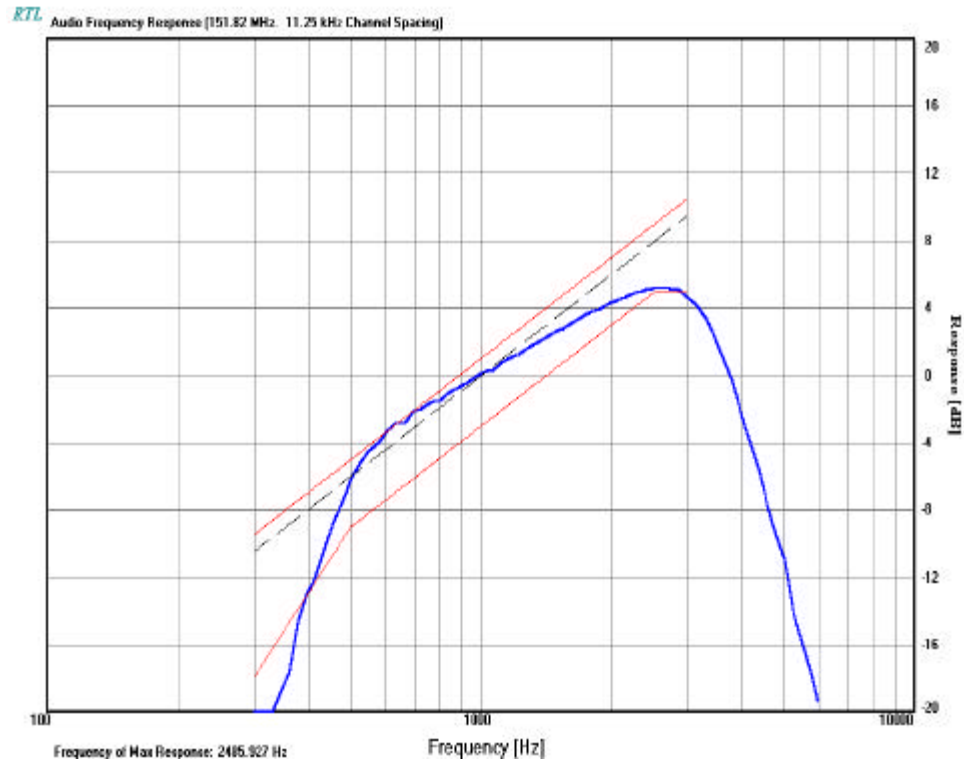
PLOT 13-1: CHANNEL 1 – 11.25 KHZ AUDIO FREQUENCY RESPONSE (MURS-22)
