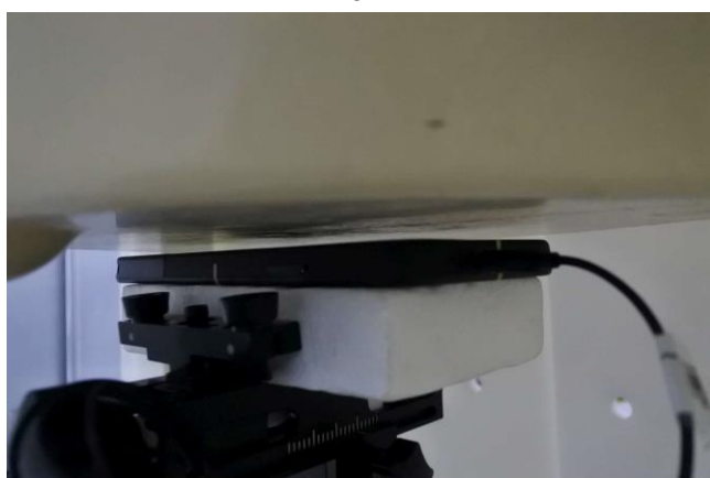
Back with handset, Test Separation 5 mm
