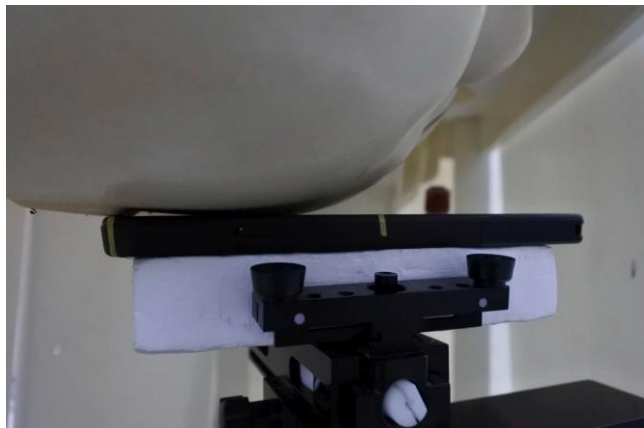
Right Cheek, Test Separation 0 mm
