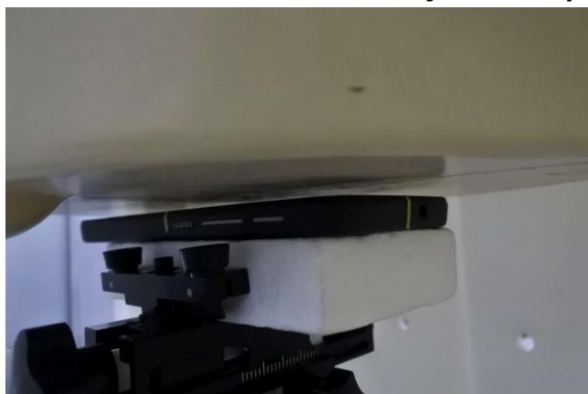
Front, Test Separation 5 mm
