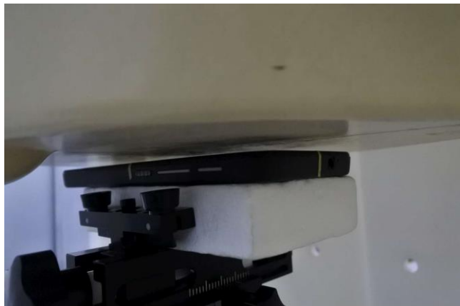
Front, Test Separation 5 mm
