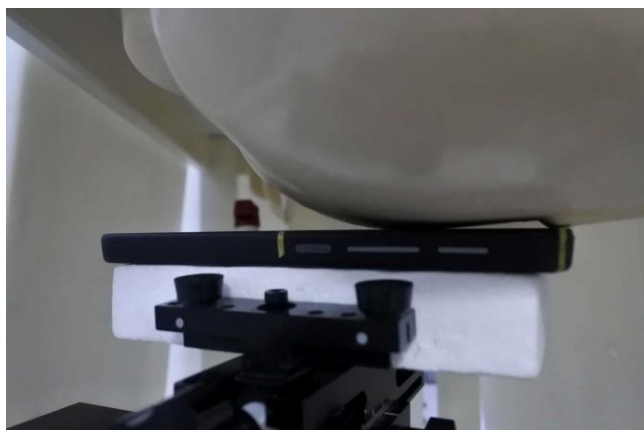
Left Cheek, Test Separation 0 mm
