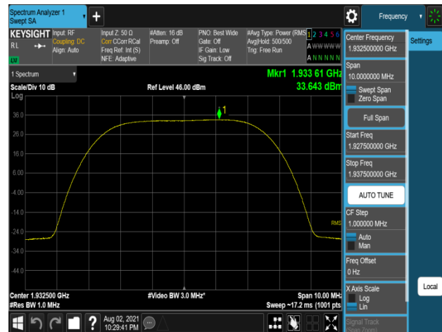
Plot 7-538. Peak Power Spectral Density Plot (B2_5M_1C_16QAM – High Channel, Port 1)
