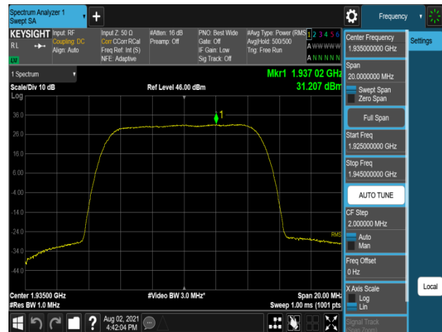
Plot 7-544. Peak Power Spectral Density Plot (B2_10M_1C_16QAM - Low Channel, Port 3)
