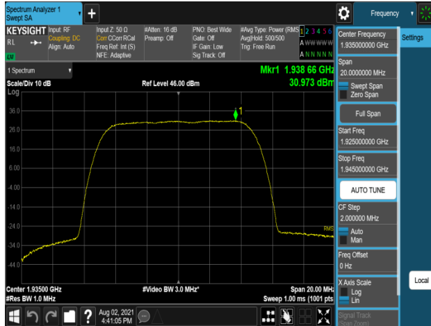
Plot 7-541. Peak Power Spectral Density Plot (B2_10M_1C_16QAM - Low Channel, Port 0)
