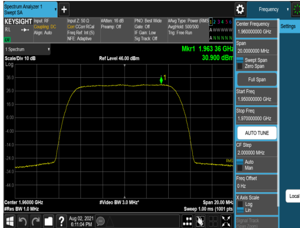
Plot 7-547. Peak Power Spectral Density Plot (B2_10M_1C_16QAM – Mid Channel, Port 2)
