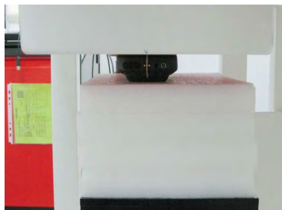
Fig.3 EUT Front side to flat phantom
