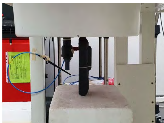
Fig.7 EUT Bottom side to flat phantom
