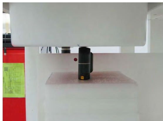
Fig.9 EUT Left side to flat phantom
