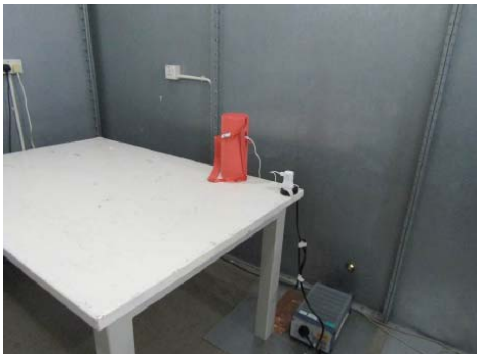
Measurement of Conducted Emission Test Set Up
