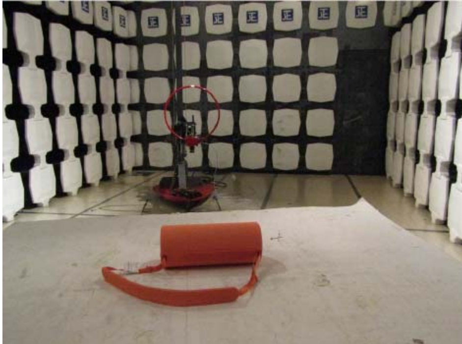
Measurement of Radiated Emission Test Set Up
