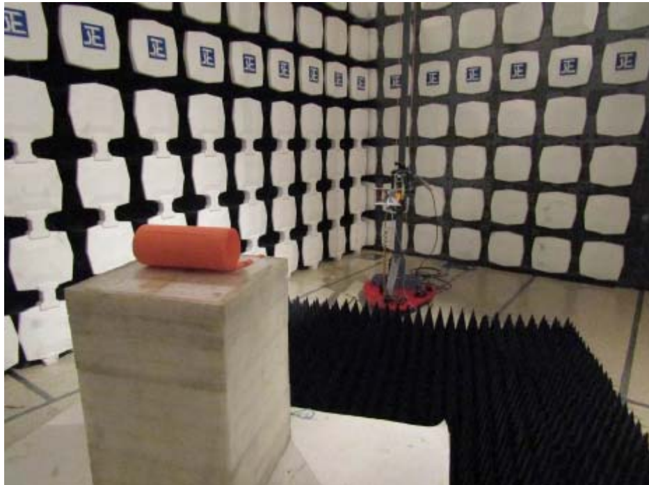
Measurement of Radiated Emission Test Set Up
