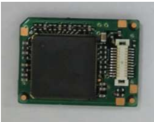
IC-F7520 AES/DES UNIT (UT-125 FIPS) SIDE B
