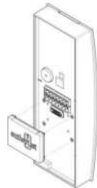
**5** Position the SABRE module (with logo up), onto the Hirose connector and press firmly to make a connection.
