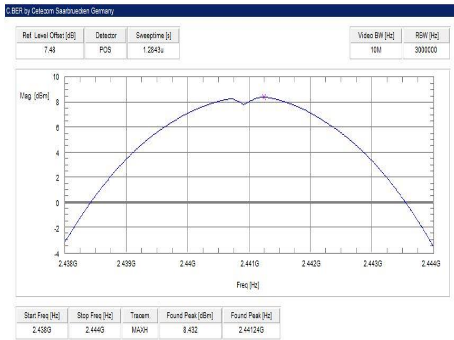
Plot 8: middle channel – 2441 MHz, 8 DPSK modulation
