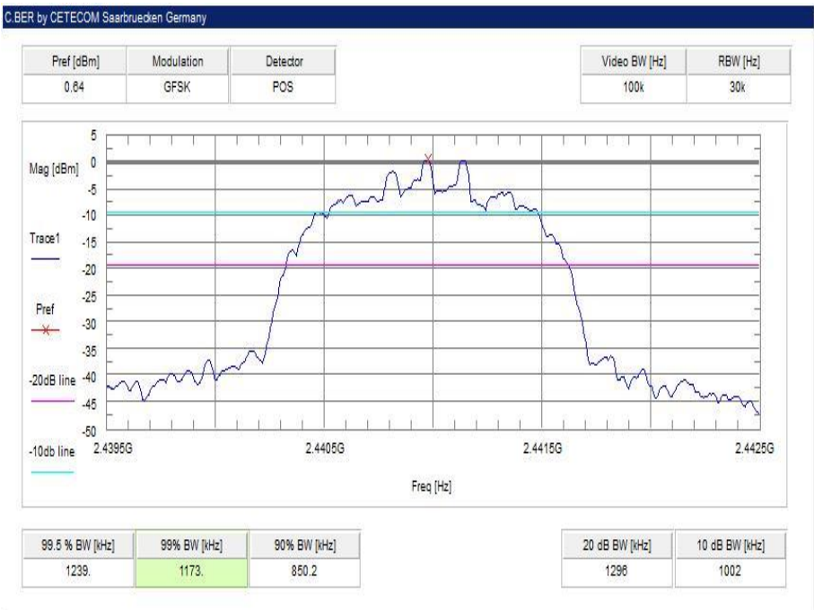
Plot 8: middle channel – 2441 MHz, 8 DPSK modulation
