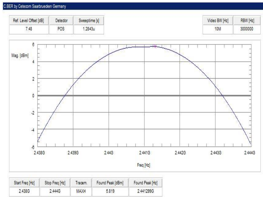
Plot 2: middle channel – 2441 MHz, GFSK modulation
