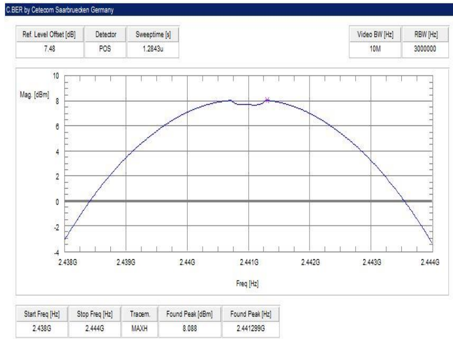
Plot 5: middle channel – 2441 MHz, Pi / DQPSK modulation
