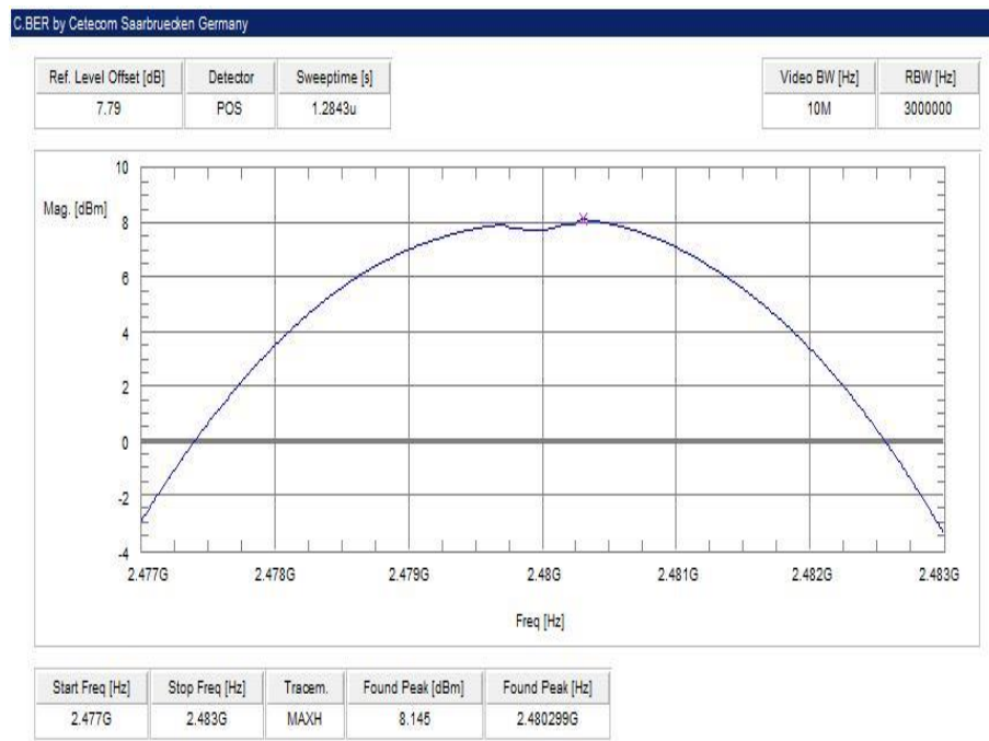
Plot 6: highest channel – 2480 MHz, Pi / DQPSK modulation
