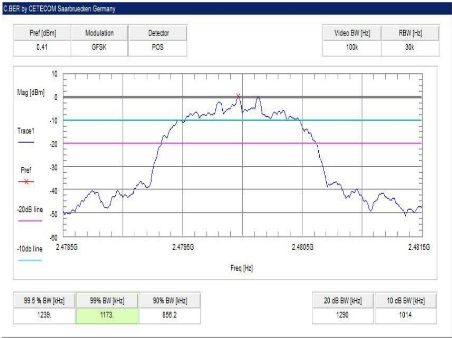
Plot 9: highest channel – 2480 MHz, 8 DPSK modulation
