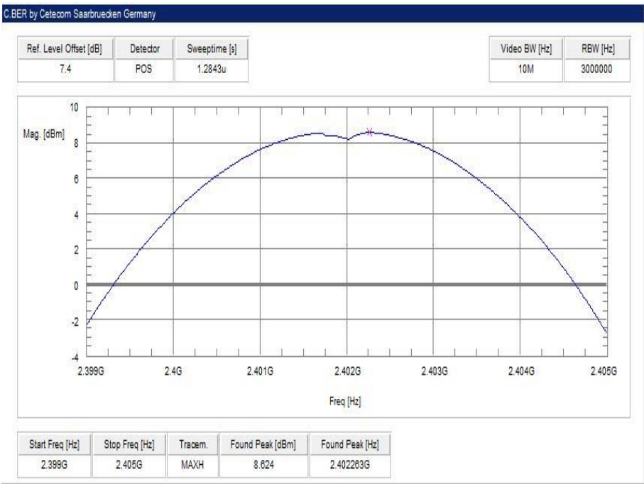
Plot 4: lowest channel – 2402 MHz, Pi / DQPSK modulation
