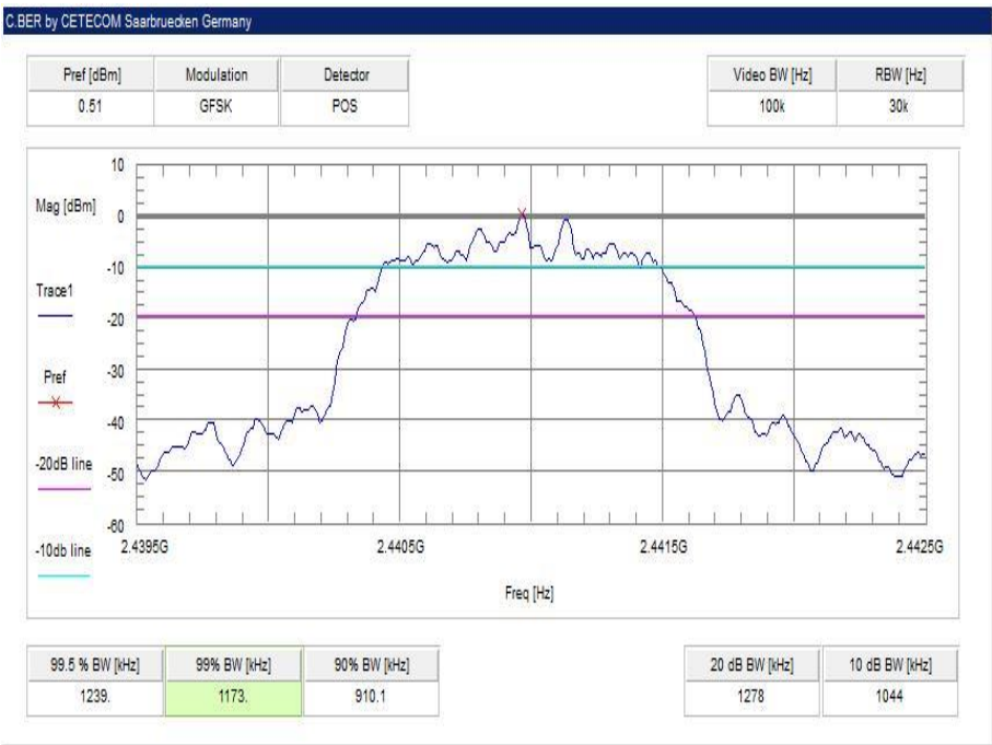
Plot 5: middle channel – 2441 MHz, Pi / DQPSK modulation
