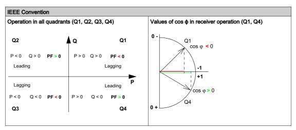
**NOTE:** For a device, a part of an installation which is only a receiver (or generator), the advantage of the IEEE convention is that it adds the type of reactive component to the PF and  $\cos \phi$  indicators:
