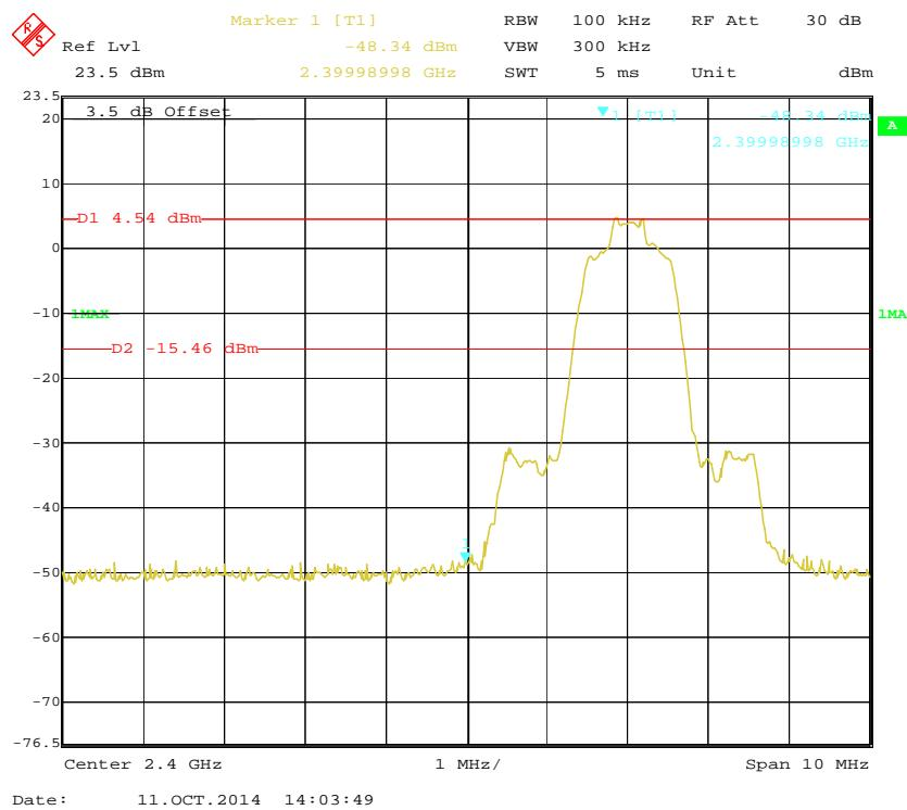
**EDR ( $\pi/4$ -DQPSK): Band Edge-Right Side**
