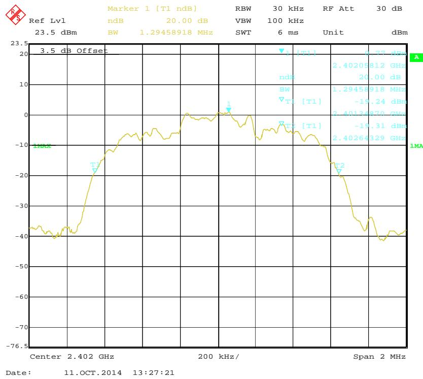
**EDR ( $\pi/4$ -DQPSK): Middle Channel**
