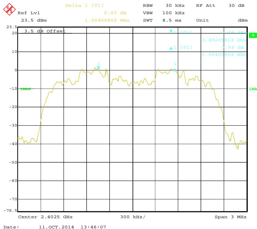
**EDR ( $\pi/4$ -DQPSK): Middle Channel**
