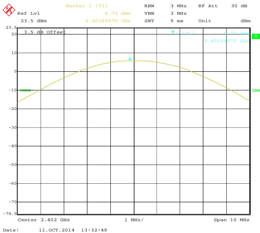
**BDR (GFSK): Middle Channel**
