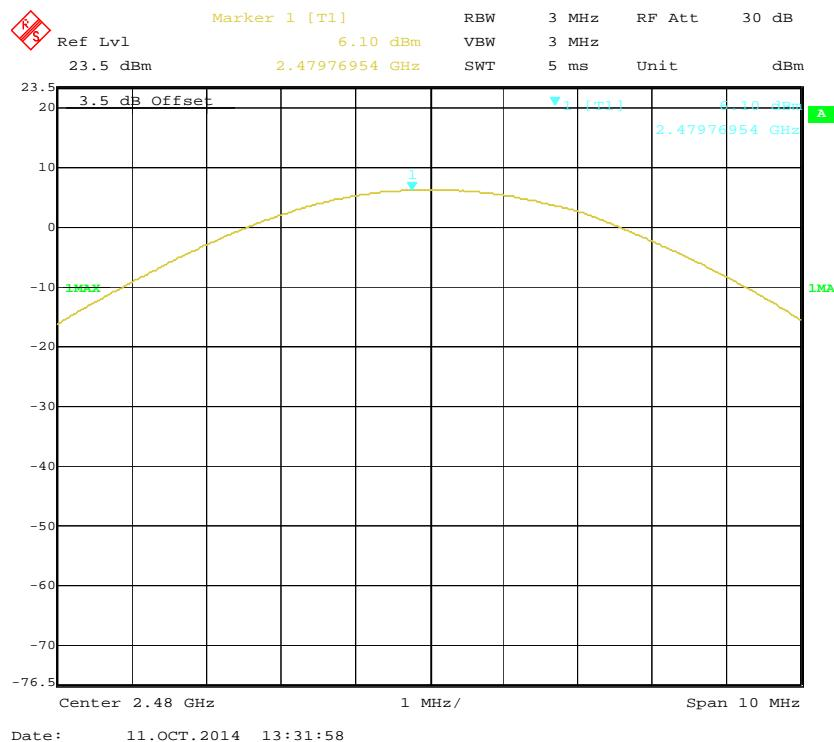
**EDR( $\pi/4$ -DQPSK): Low Channel**
