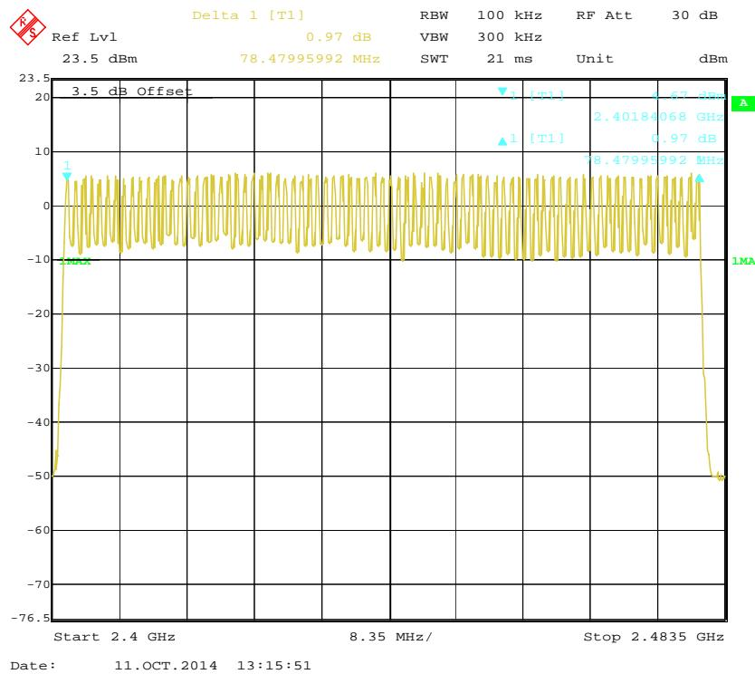
**EDR ( $\pi/4$ -DQPSK): Number of Hopping Channels**
