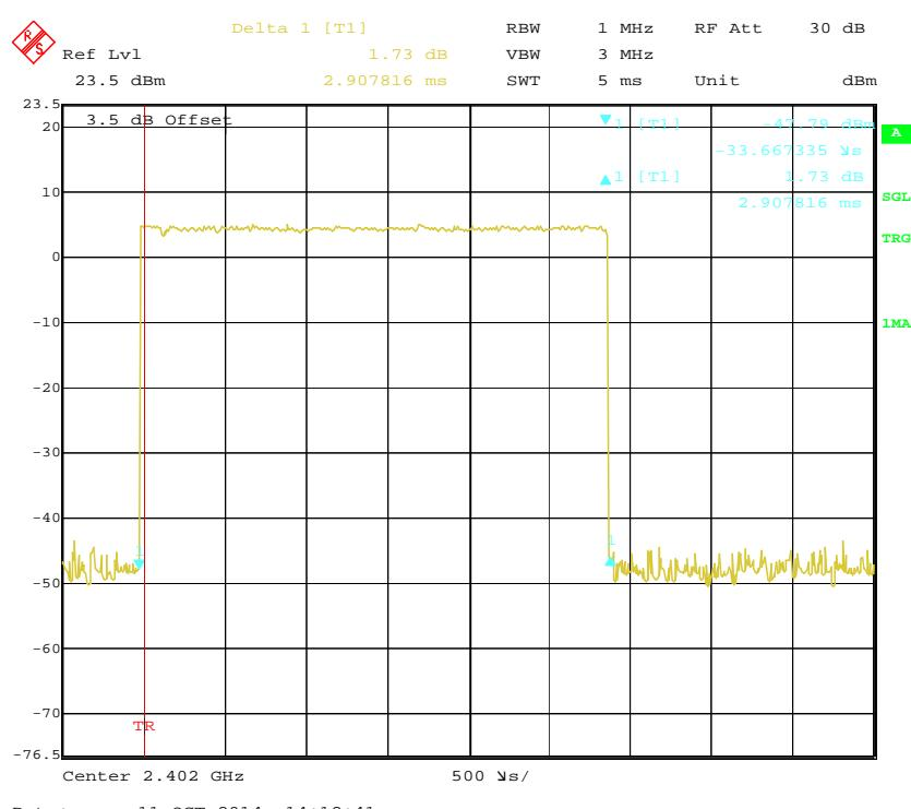
**Pulse time, Middle Channel, DH5**
