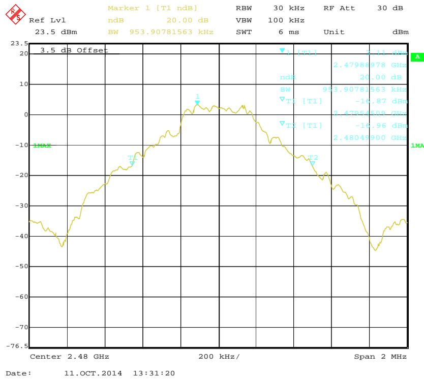
**EDR ( $\pi/4$ -DQPSK): Low Channel**
