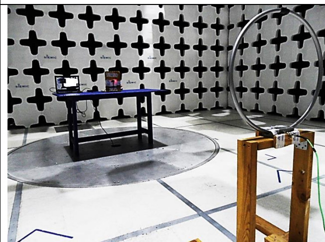
Radiated Emissions (<30MHz) – Front View
