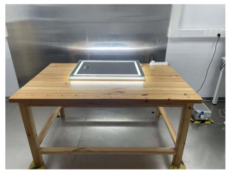
**Radiated Emission Test View Below 1GHz**
