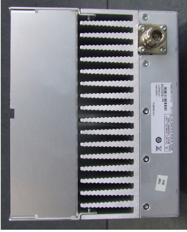
Photograph 10: Power Amplifier – Rear panel
