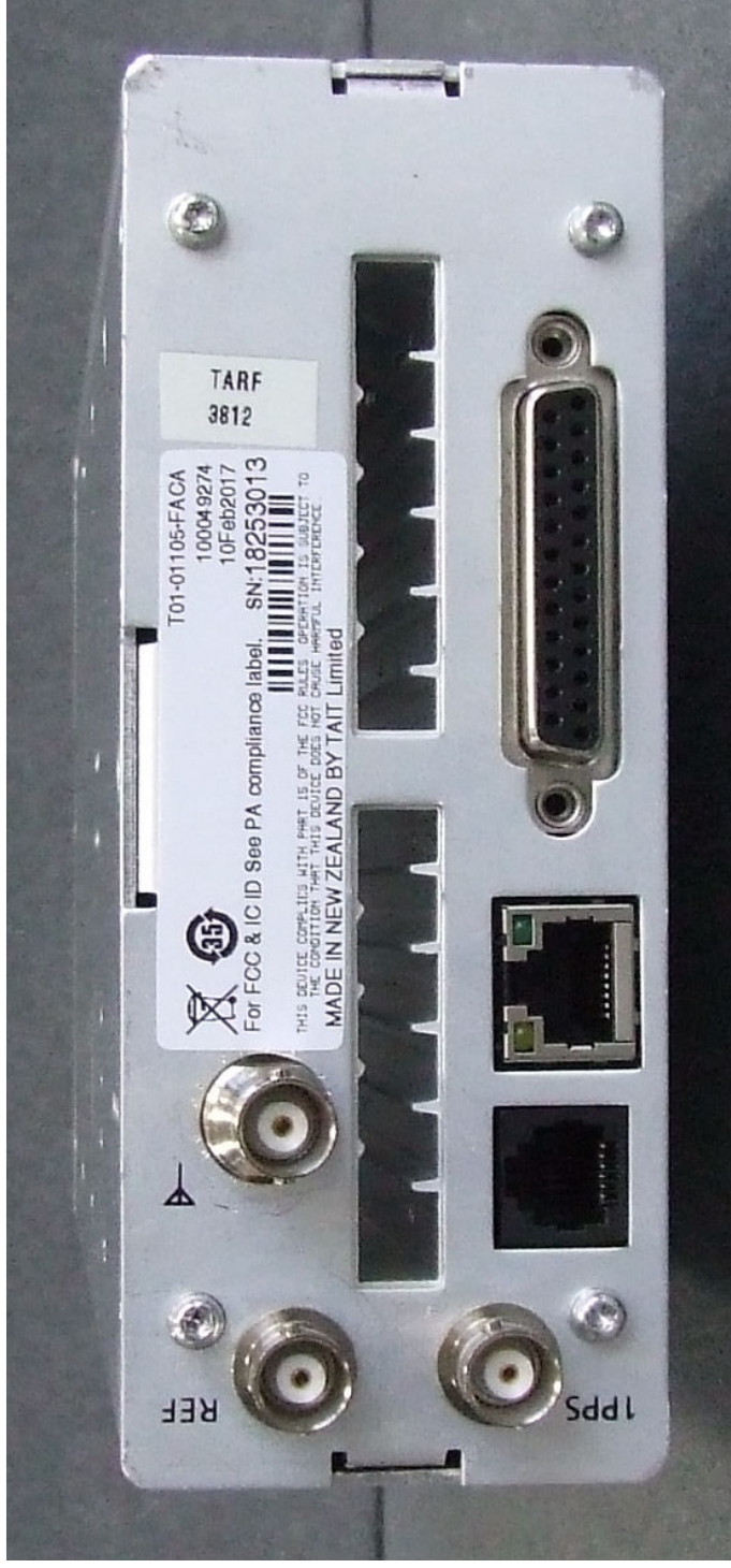
Photograph 07: Reciter module – Rear panel
