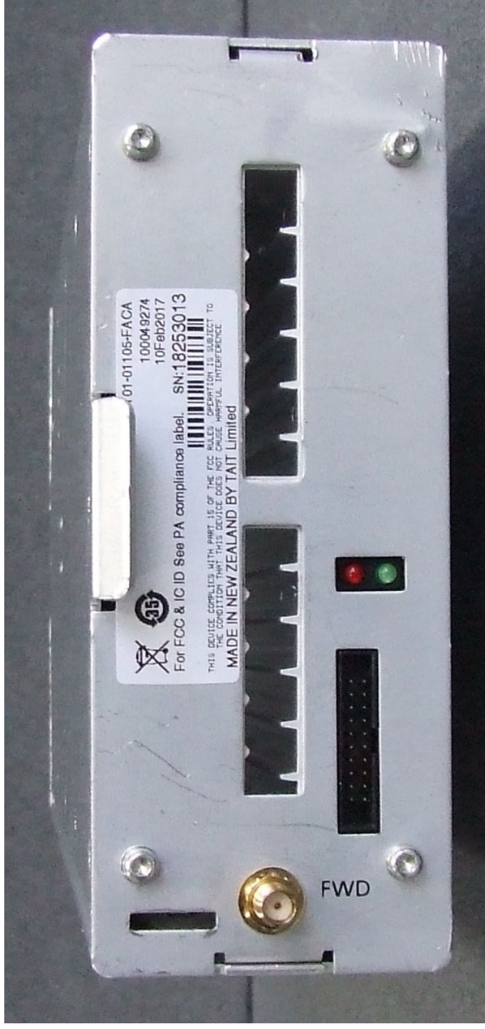
Photograph 06: Reciter module – Front panel
