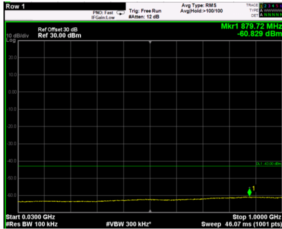
Channel: TOP, Modulation: 64QAM, BW=5MHz, Range: 30MHz - 1GHz
