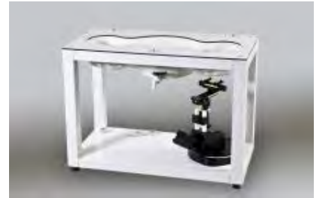
Figure 3.6 SAM Twin Phantom
