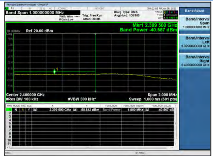
802.11b LOW CHANNEL, Reference level
