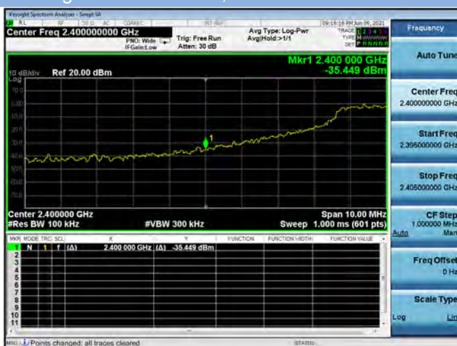
802.11g LOW CHANNEL, Carrier level
