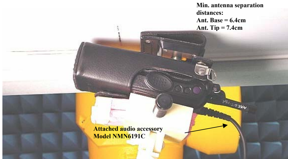
Figure 9. Assessment @ the body. DUT with carry case accessory model NTN8380B (w/ NTN8039B belt loop) against the phantom With attached audio accessory model NMN6191C
