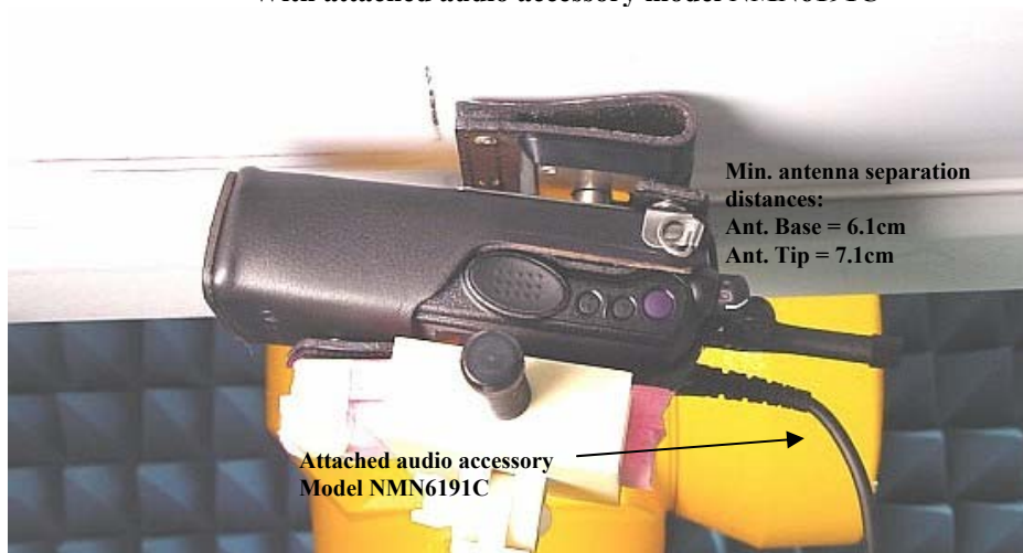
Figure 6. Assessment @ the body. DUT with carry case accessory model NTN8385A(w/ 2.5" swivel) against the phantom. With attached audio accessory model NMN6191C
