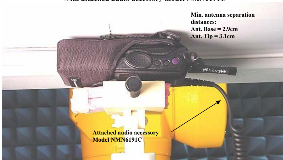
Figure 10. Assessment @ the body. DUT with carry case accessory model NTN8725A (w/ NTN8383A T-Strap) against the phantom With attached audio accessory model NMN6191C
