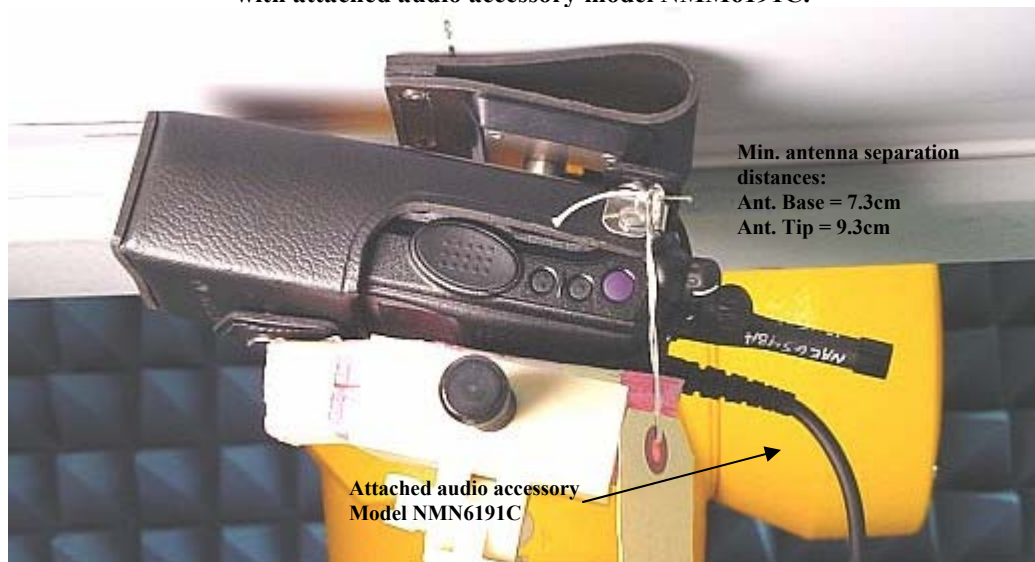
Figure 3. Assessment @ body. DUT with carry case accessory model NTN8381C against the phantom with attached audio accessory model NMM6191C.
